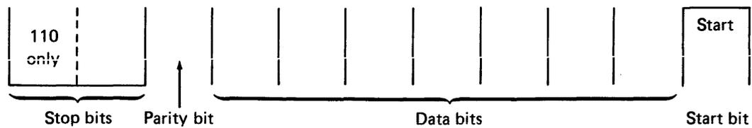
Figure 3-9. Asynchronous Format
