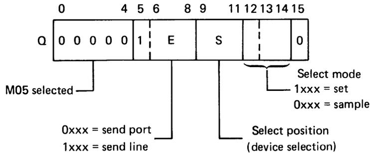
Figure 2-3. Q Register Format
