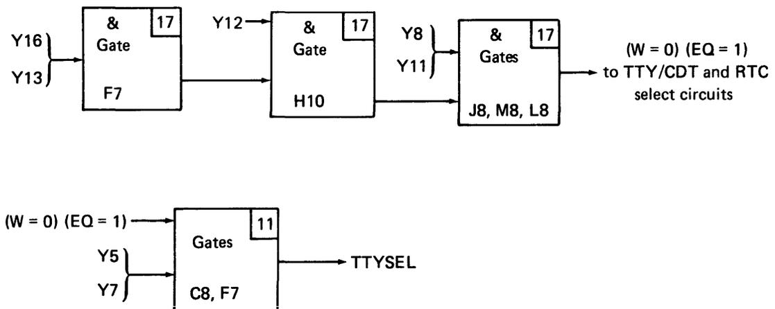
Figure 2-9. Block Diagram of TTY/CDT Selection Circuits
