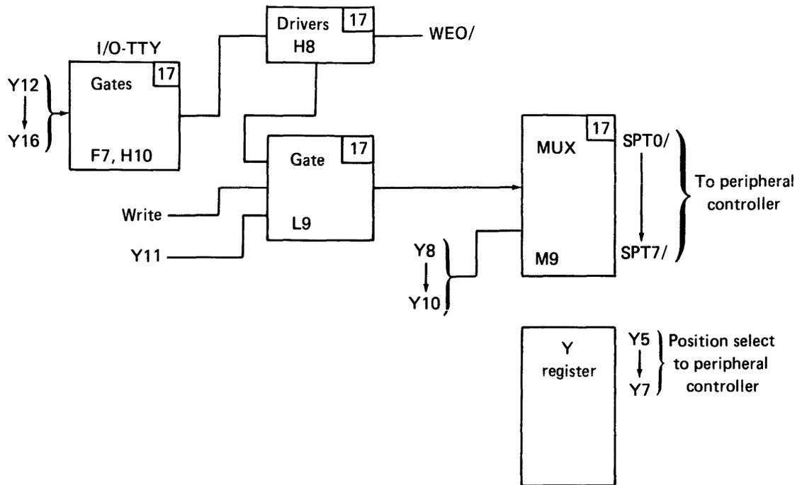
Figure 2-7. MO5 Scheme Selection Circuit
