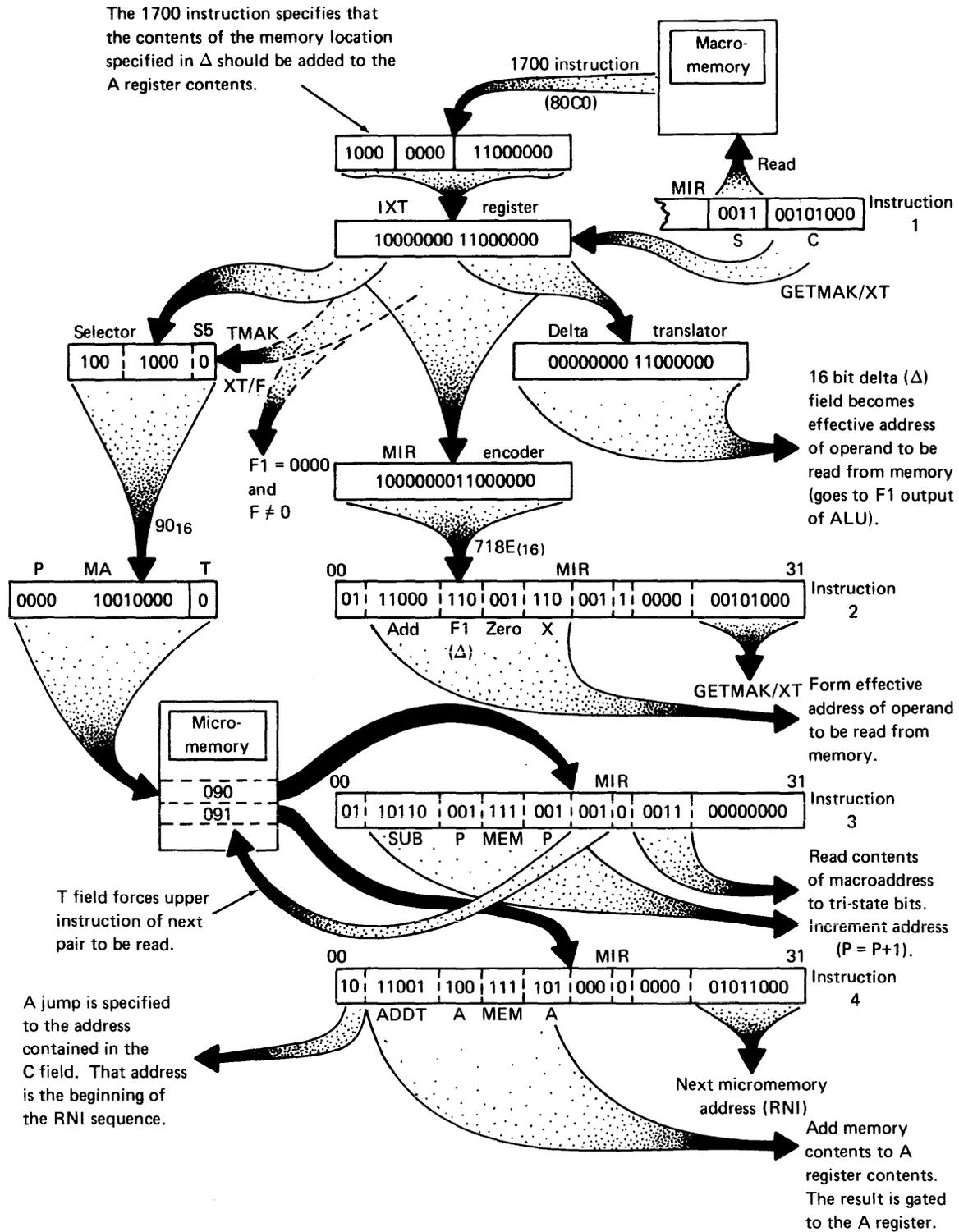
Figure 3-22. ADD to A Register Emulation Process
