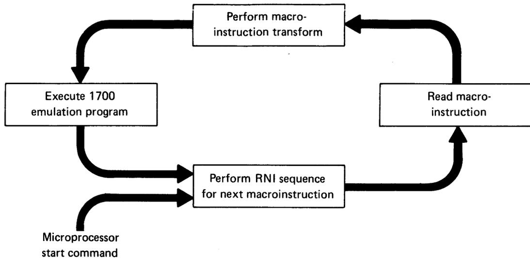
Figure 3-21. Sequence of Events in Emulation Process
