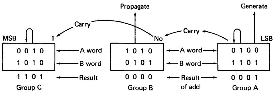
Figure 1-12 shows a typical add operation demonstrating the adder functions using look-ahead carry. In this example, a total of sixteen bits from two sources is added. The contents of each four-bit ALU chip is shown and the signals interfacing to the look-ahead carry generator are indicated.
