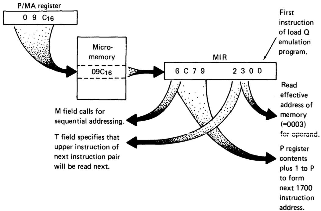
Figure 3-19. Execution of Emulation Program from Micromemory
