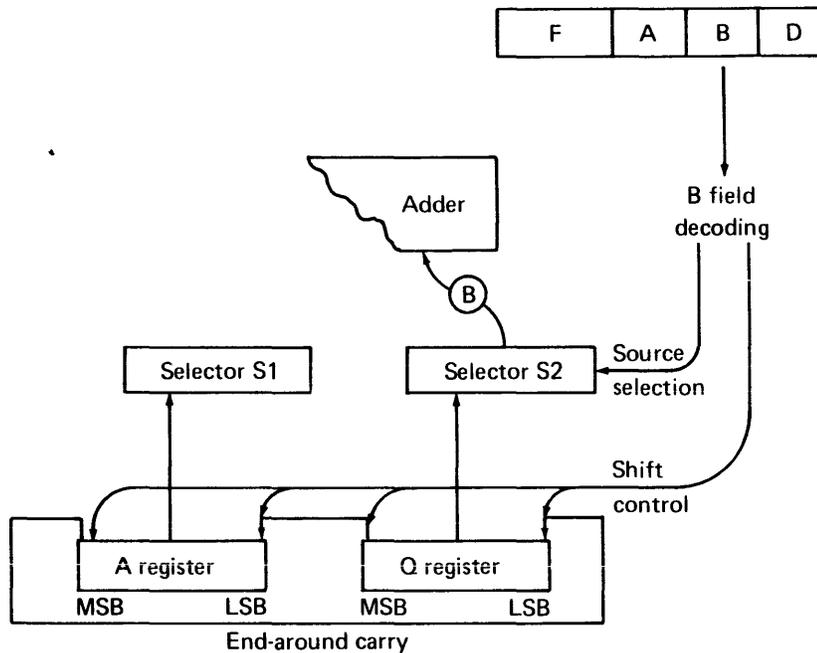
Figure 2-11. B-Field Decoding
