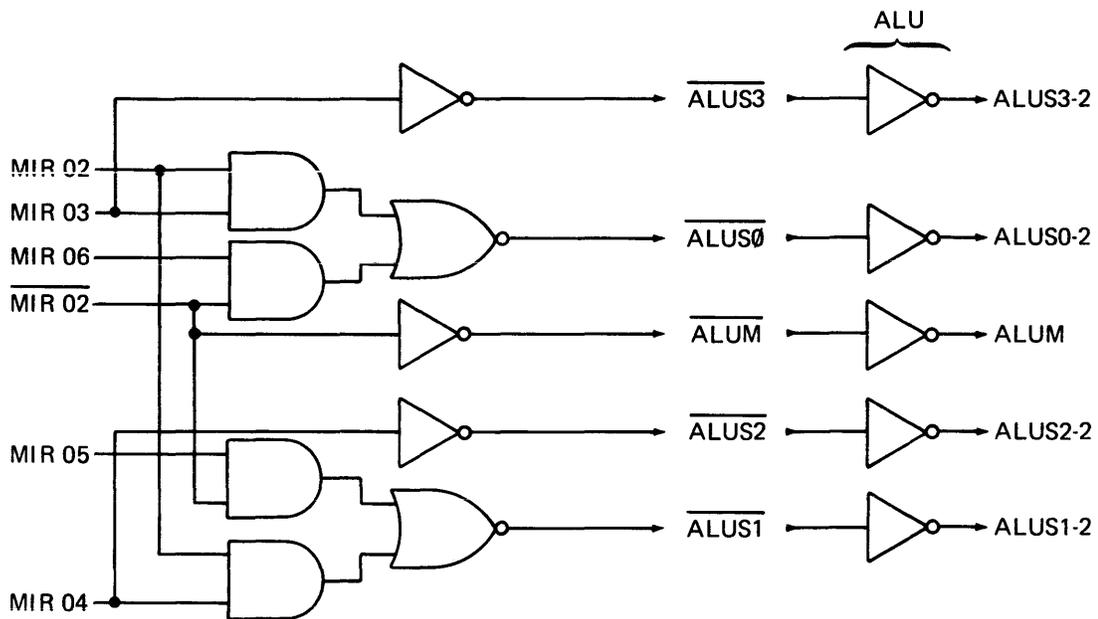
Figure 3-12. F-Field Decoder for Arithmetic and Logical Operations
