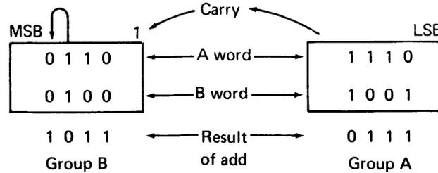
**Generate.** A generate signal occurs when an arithmetic operation is performed resulting in a carry by a four-bit group that cannot be absorbed in that group. This signal is sent from the ALU chip to the carry generator. For example:
