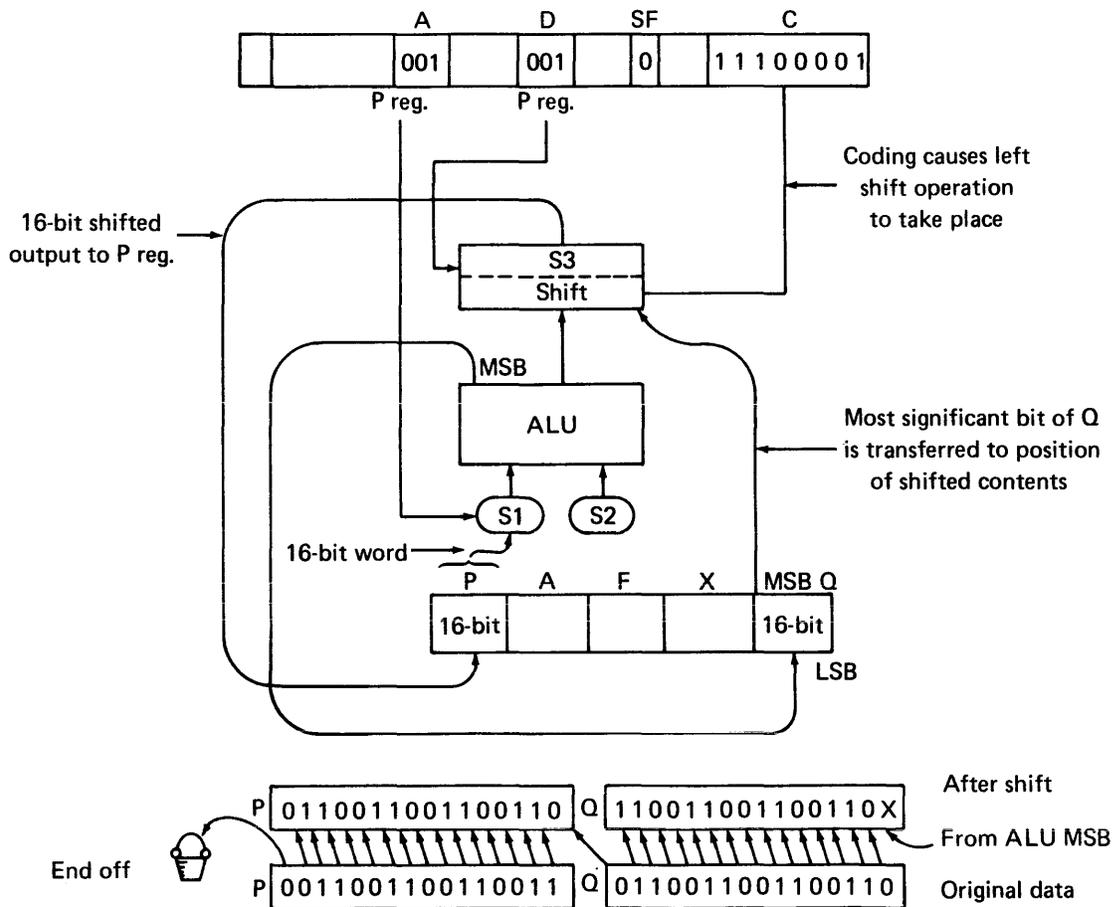
Figure 1-15. Double-Length Register Shift (P and Q)
