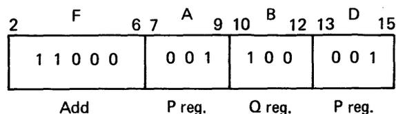
Figure 3-9. Add Operation of P and Q. Result to P
