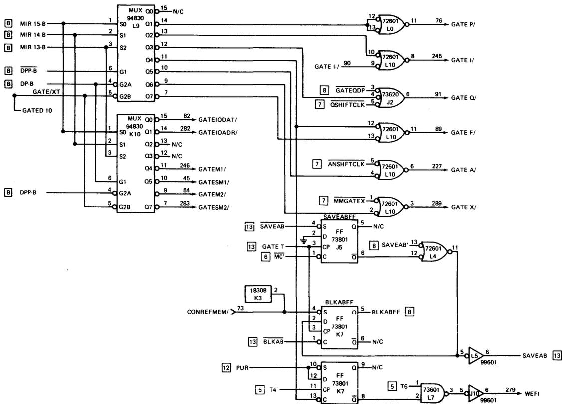
Figure 3-13. D-Field Decoder
