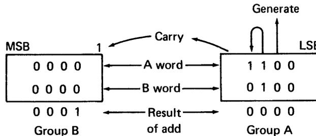
**Propagate.** A propagate signal is generated to the carry generator when an arithmetic operation results in all 1s and there is, therefore, no place for a carry to the group to be absorbed. Any carry into this group would be forced into the next group able to absorb the carry.
