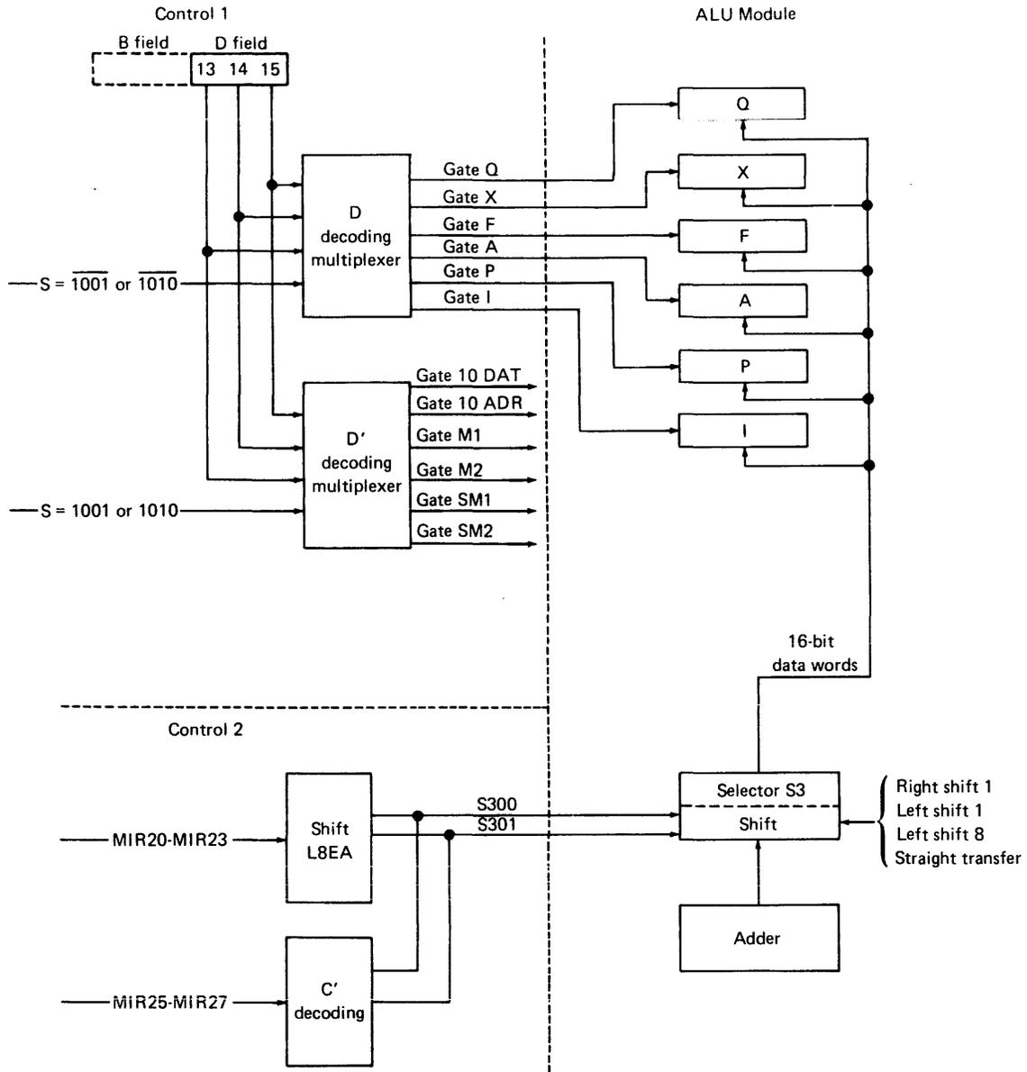
Figure 2-14. D-Field Decoding
