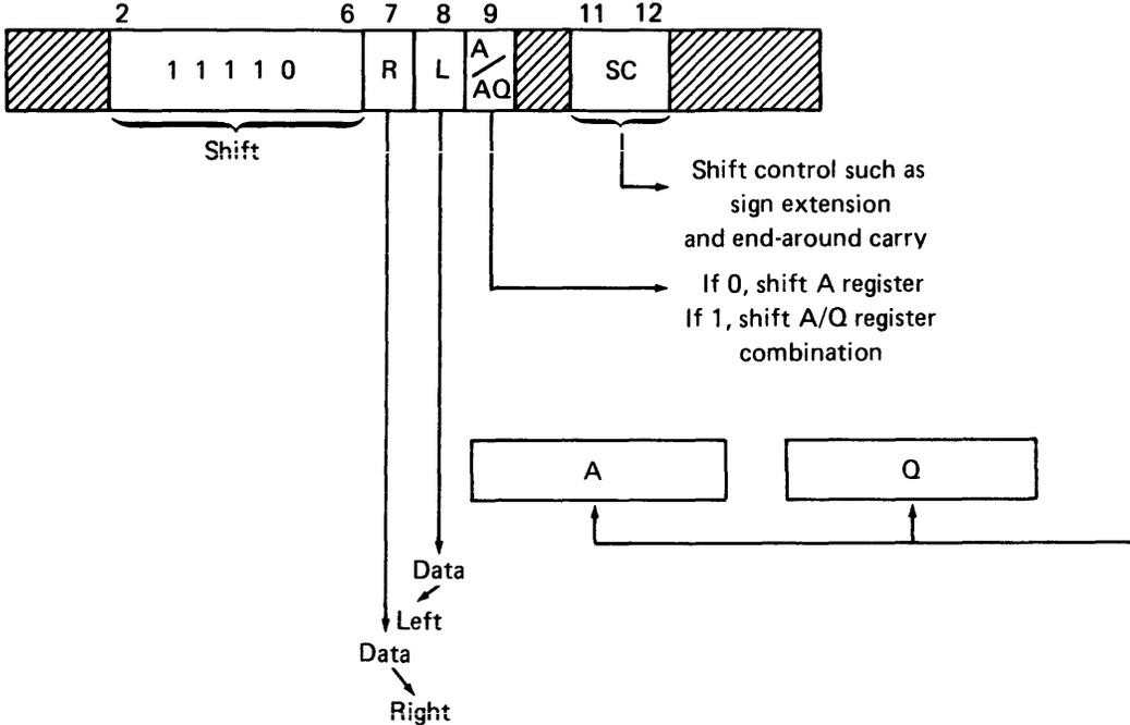
Figure 2-8. ALU Control Subfield Meanings for Shift and Scale Operations
