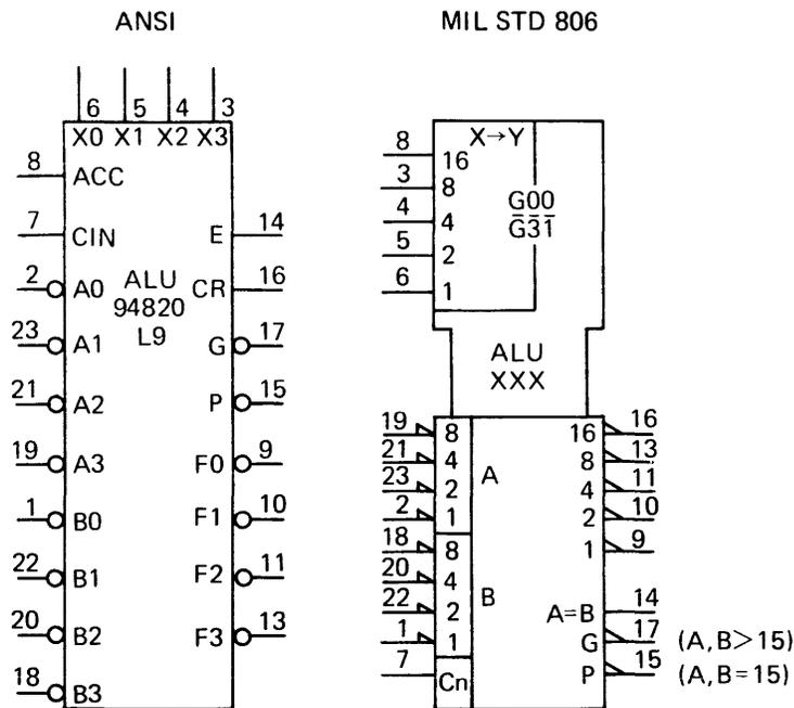
Figure 1-11. Four-Bit Adder
