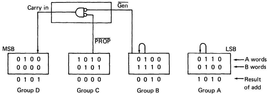
Figure 1-12. Typical Additive Operation Using Look-Ahead Carry
