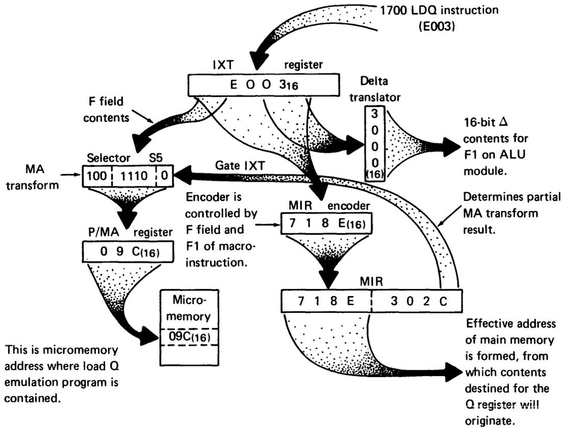
Figure 3-18. Transform of a 1700 LOAD Q Instruction
