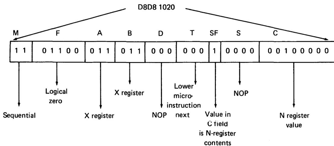
Figure 2-18. N Register Value Set to  $32_{10}$  ( $20_{16}$ )
