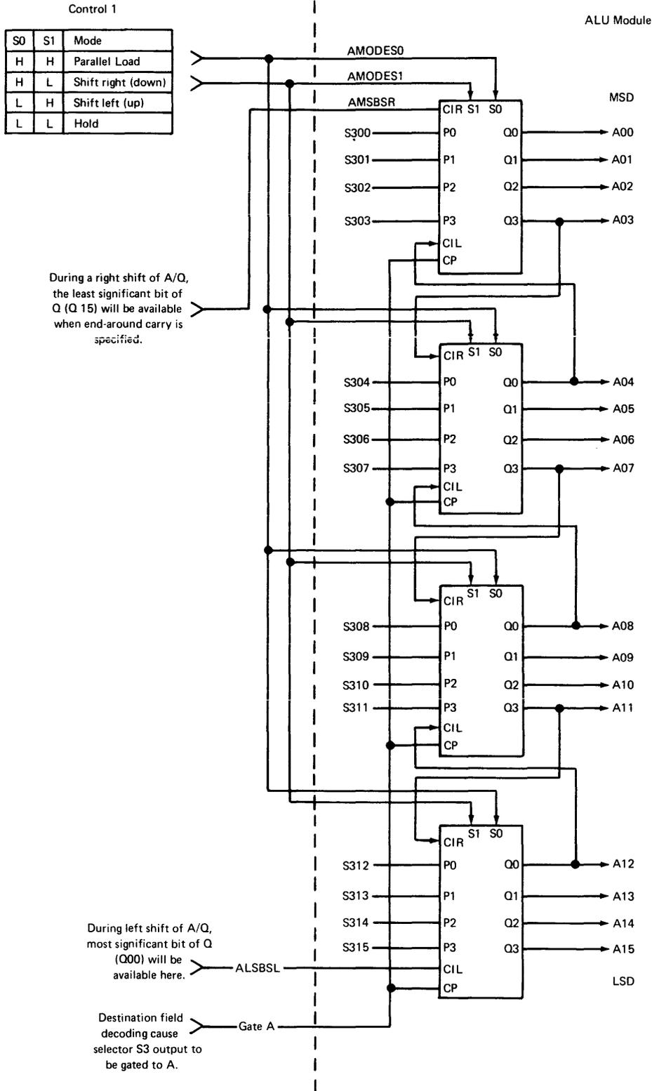
Figure 3-3. A Register and Control Signals
