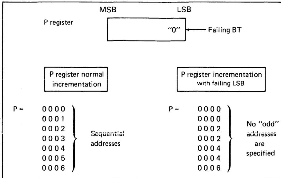
Figure 3. P Register Failure
