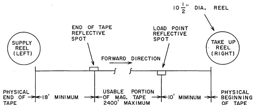
Figure 3. Physical Layout of Tape
