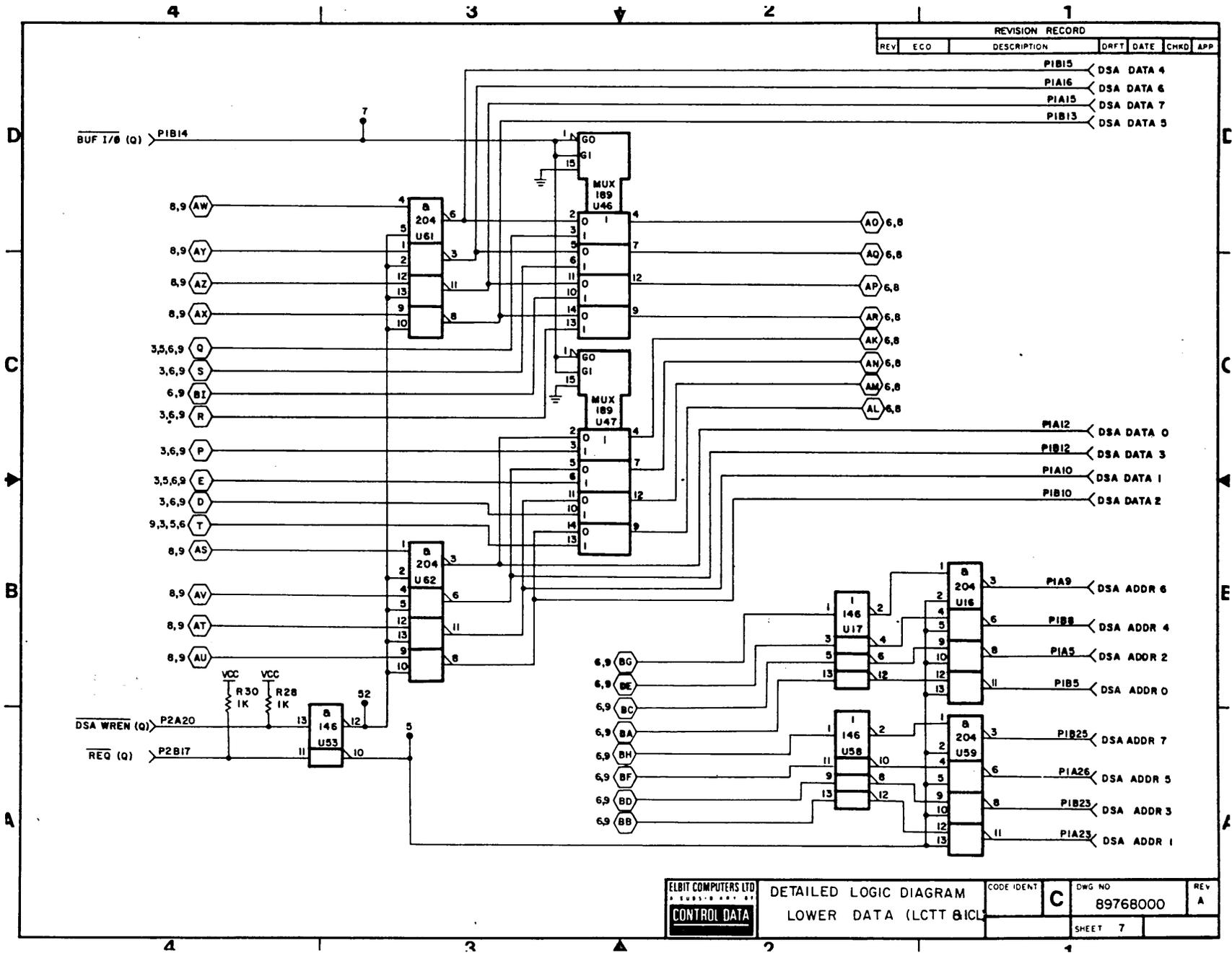
Figure 5-28. Lower Data Section - Lower DSA Data Path Logic Diagram (Cont'd)
