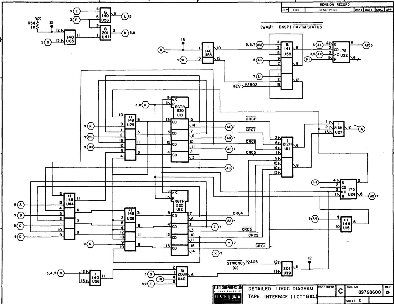
Figure 5-49. Tape Interface - CRC Generator Detector Logic Diagram
