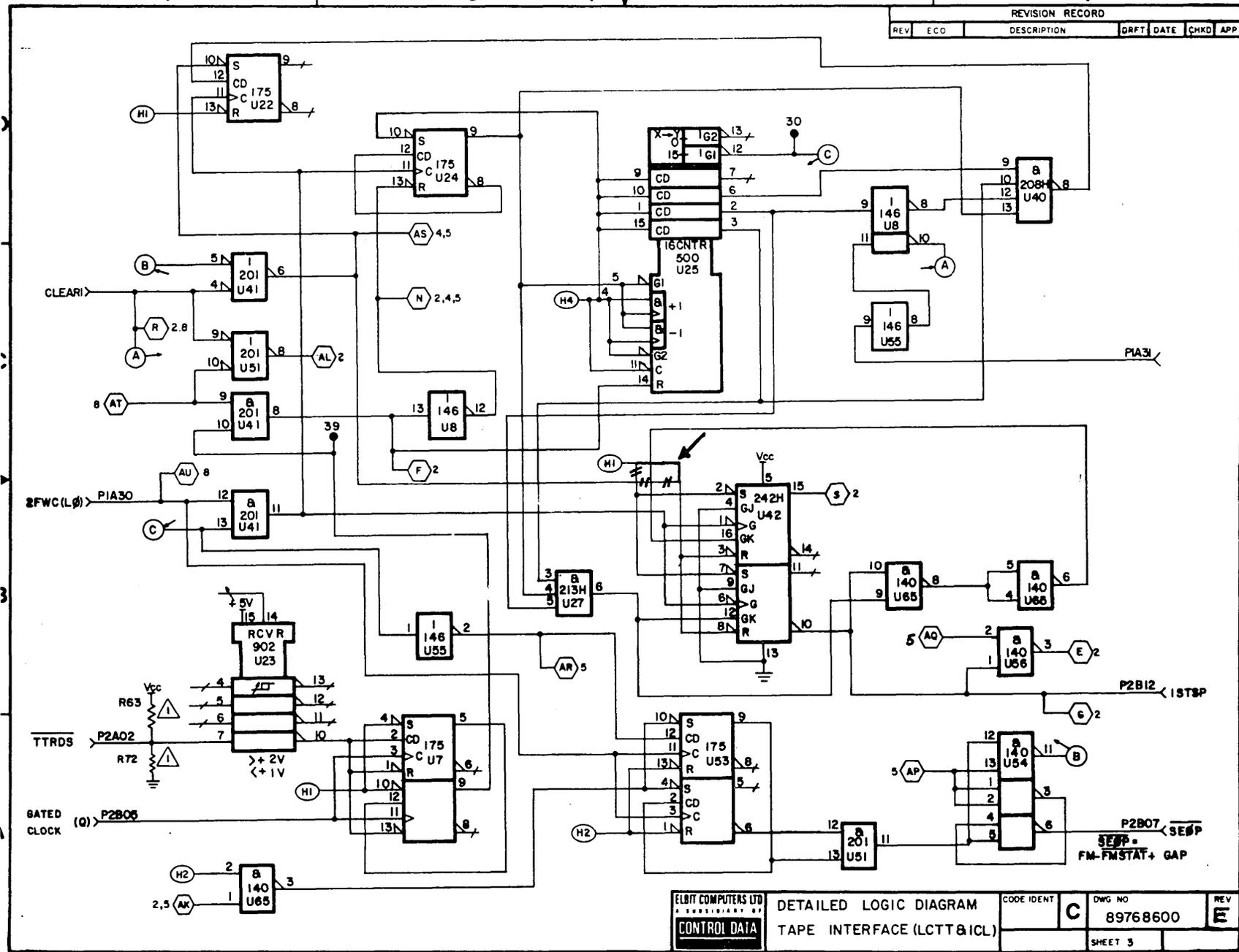
Figure 5-52. Tape Interface - Data Strobe/EOR Detector Logic Diagram
