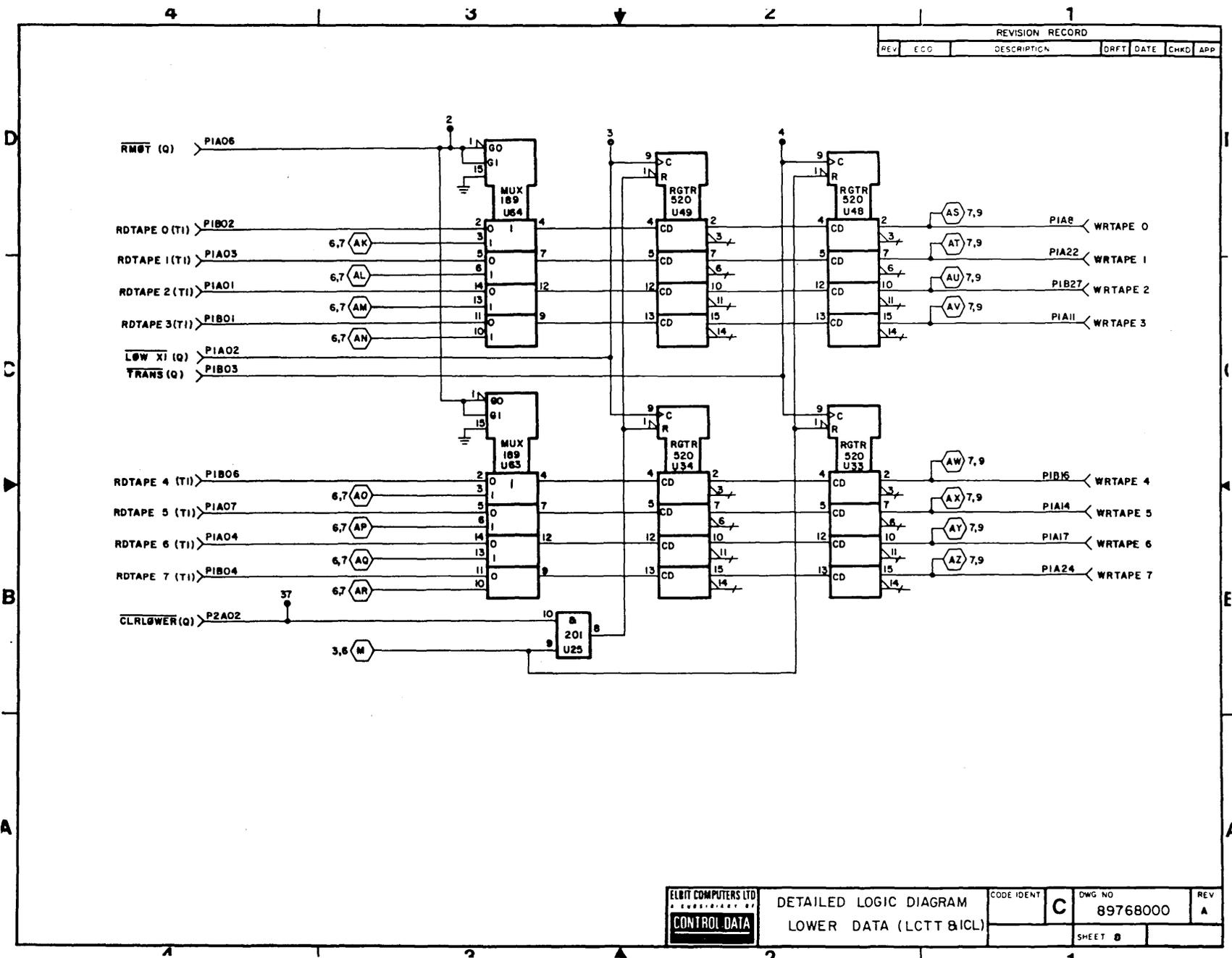
Figure 5-30. Lower Data Section - Lower A Data Path Logic Diagram
