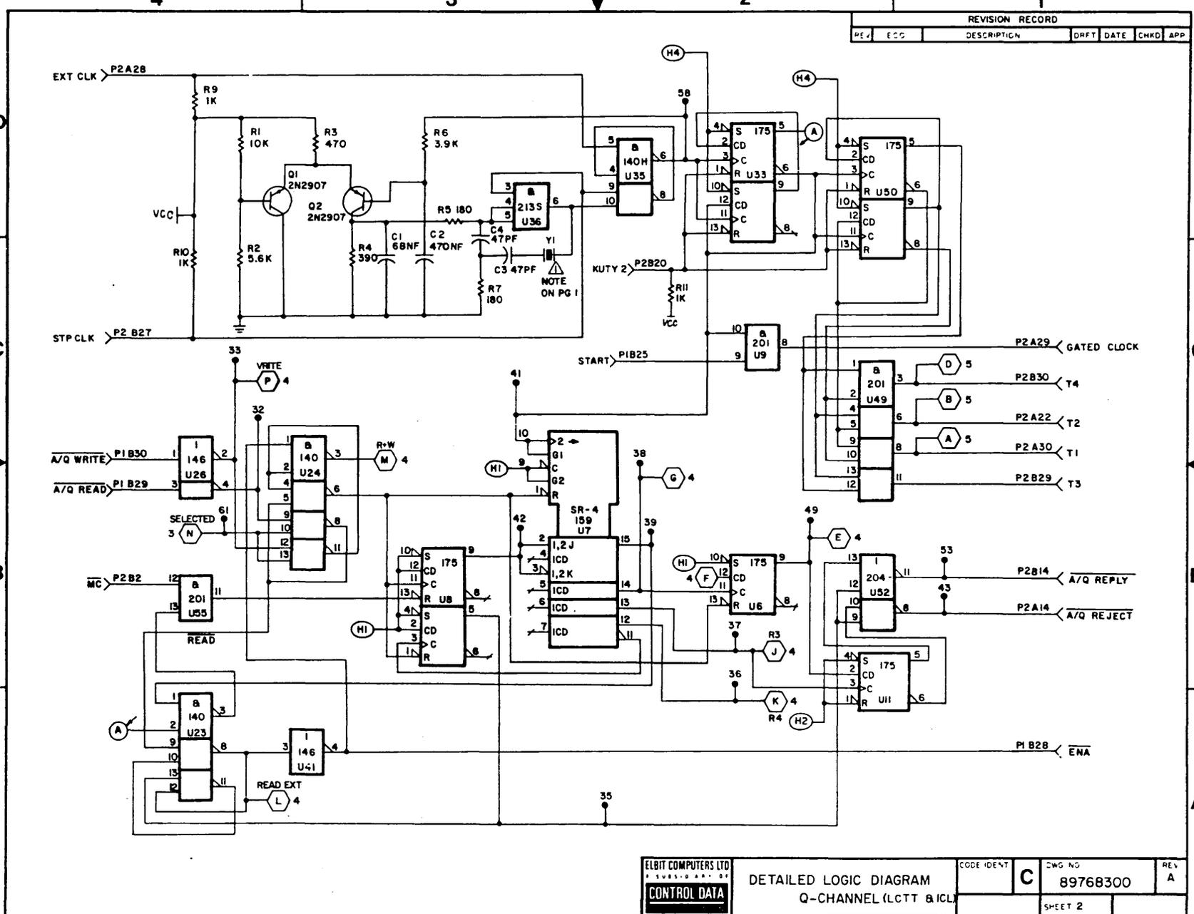
Figure 5-4. Q-Channel - Clock and Reply/Reject Logic Diagram
