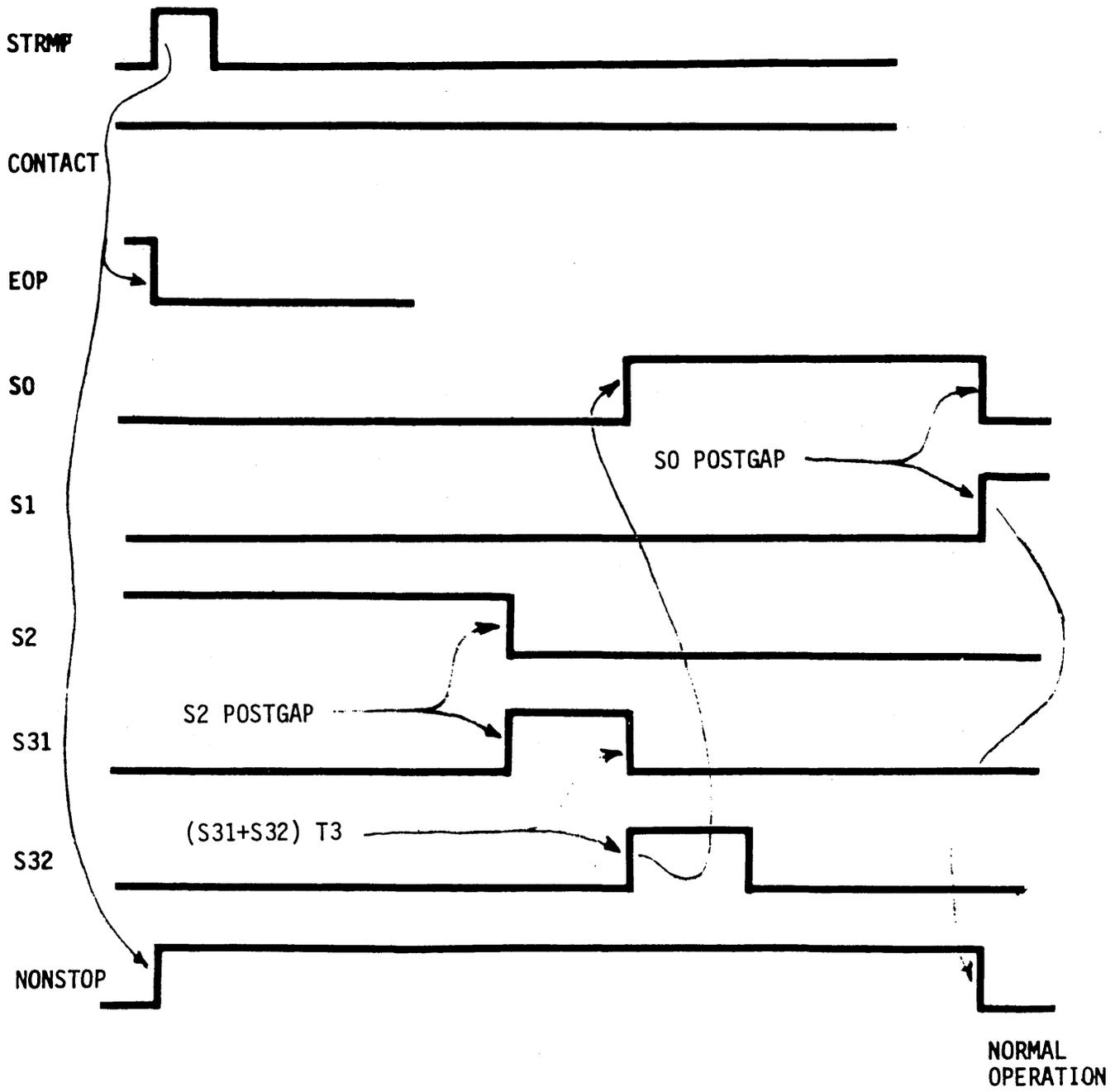
Figure 5-37. Non-Stop Motion Operation
