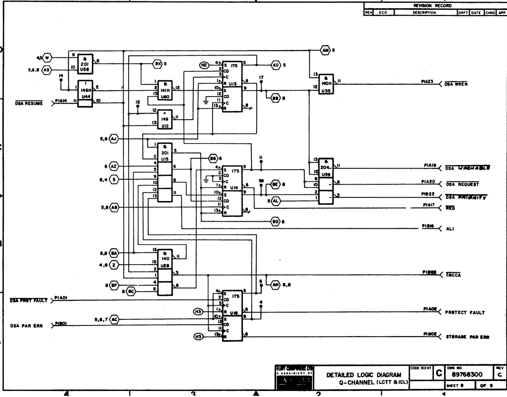
Figure 5-17. Q-Channel - Request Resume Logic Diagram
