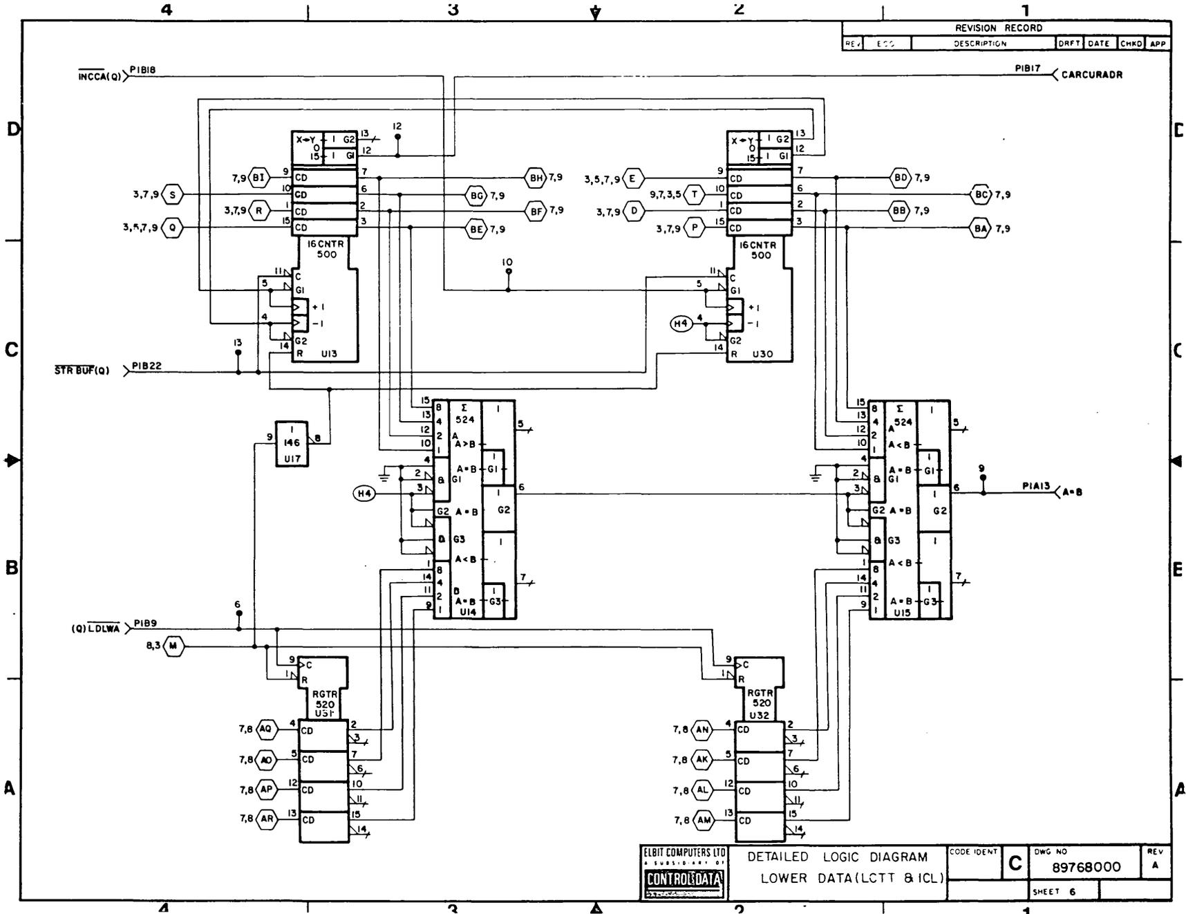
Figure 5-27. Lower Data Section - Lower DSA Data Path Logic Diagram
