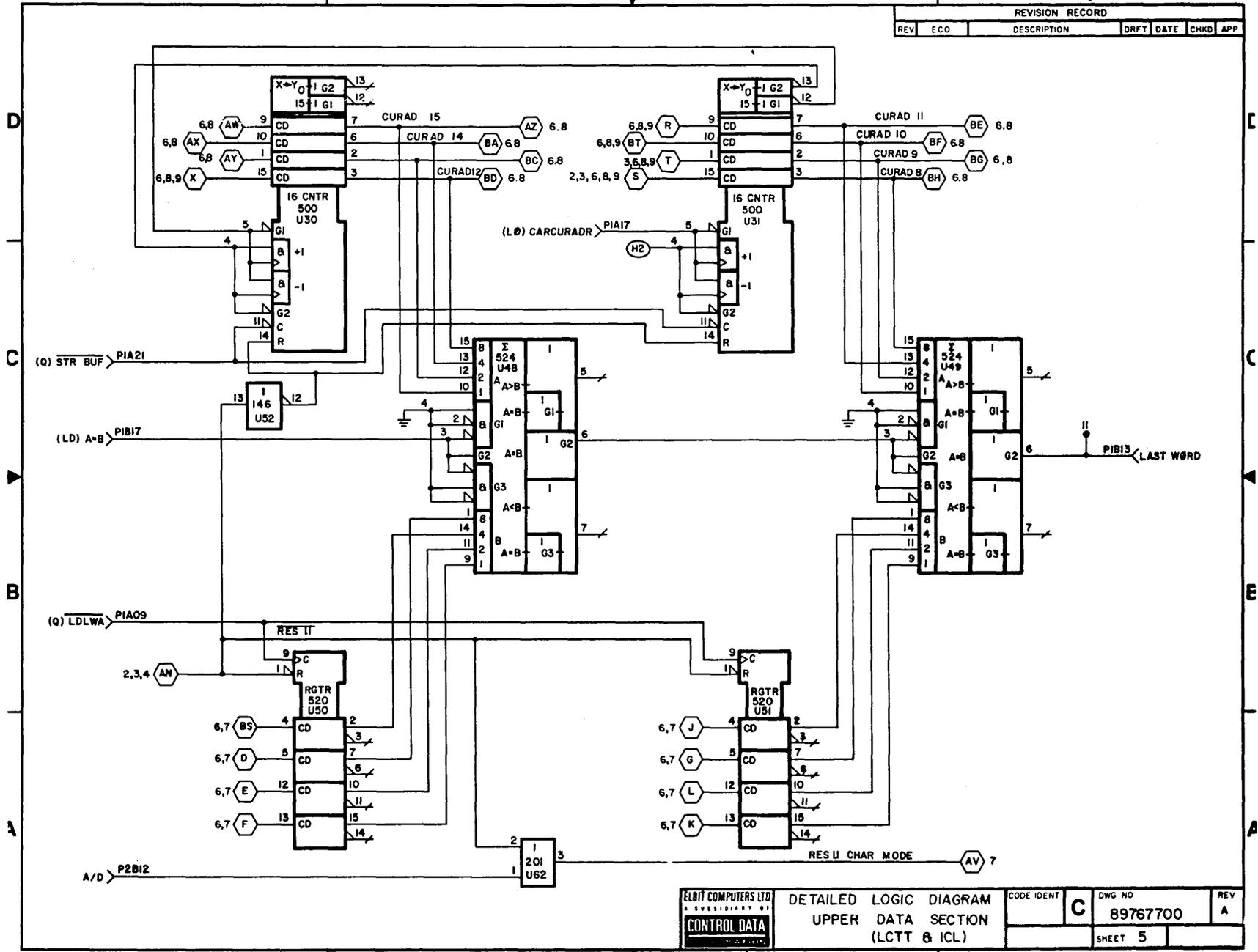
Figure 5-41. Upper Data Section Upper DSA Data Path Logic Diagram
