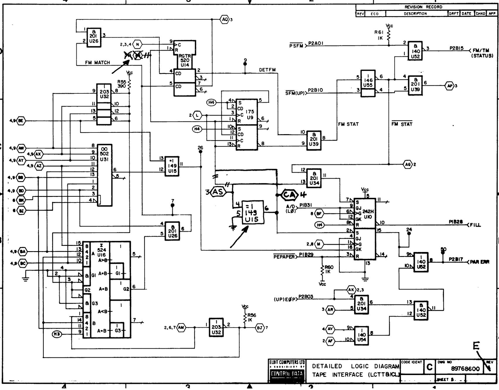
Figure 5-54. Tape Interface - Parity Error/Fill/FM Detector Logic Diagram
