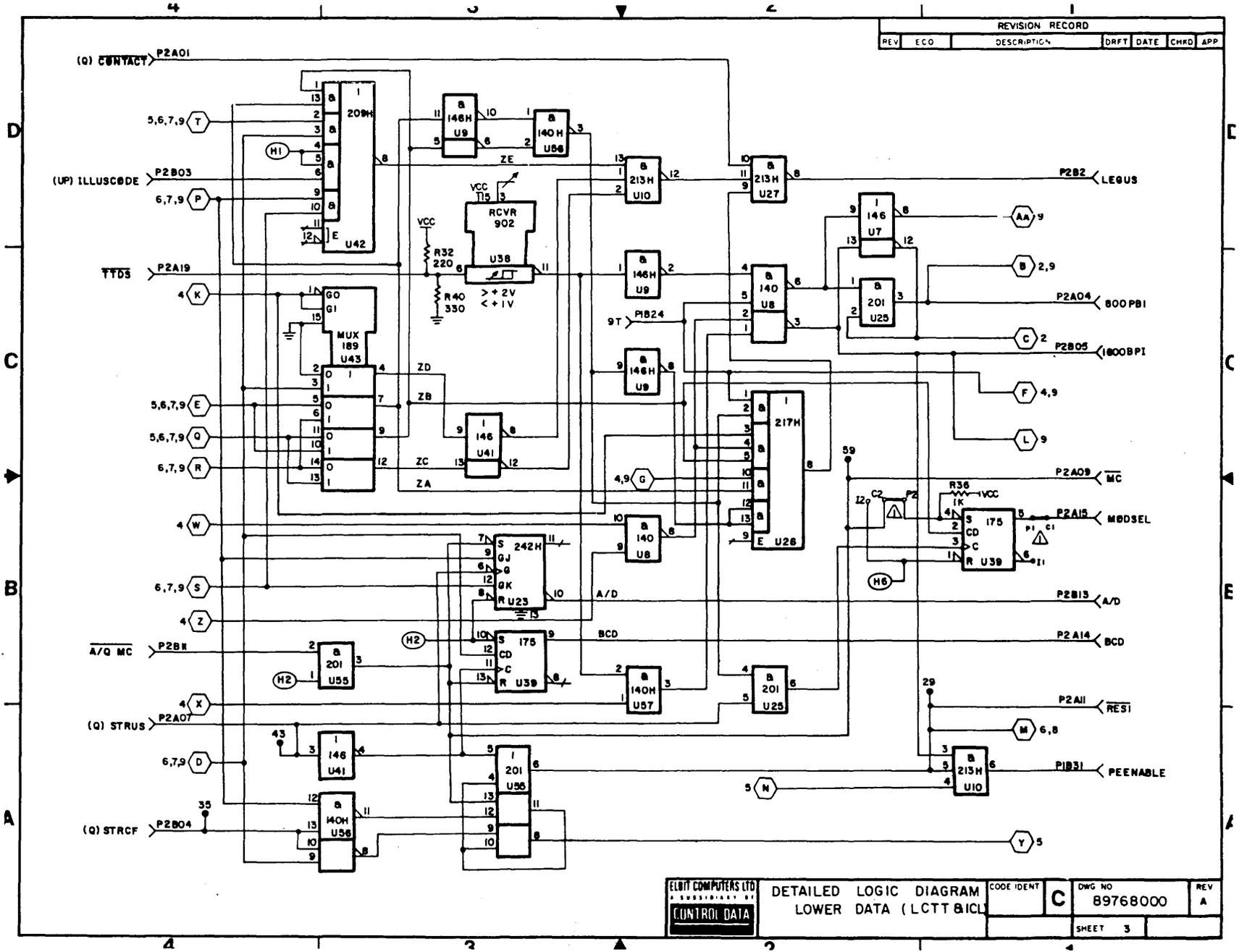
Figure 5-23. Lower Data Section - Operation Conditions Logic Diagram
