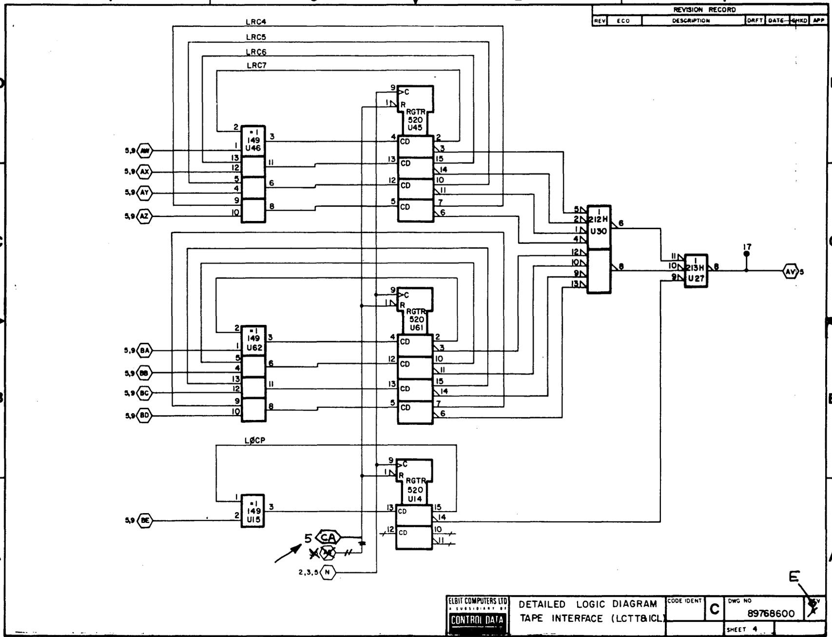
Figure 5-53. Tape Interface - LRC Detector Logic Diagram
