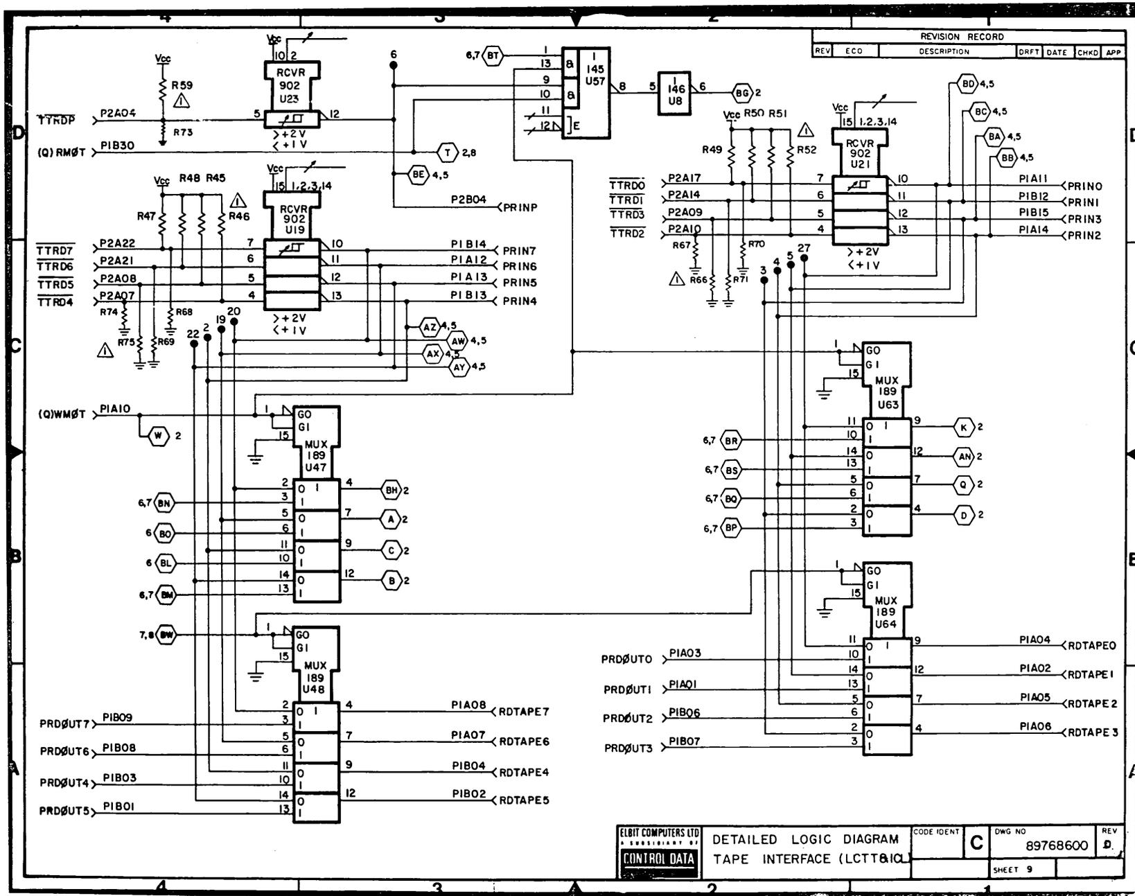
Figure 5-60. Tape Interface - MTT/PE Read Data Path Logic Diagram
