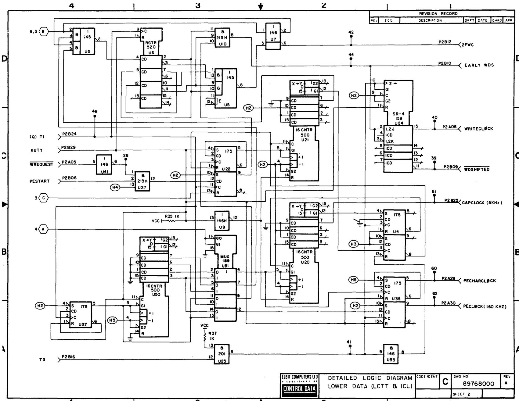
Figure 5-22. Lower Data Section - Basic Timing Generator Logic Diagram
