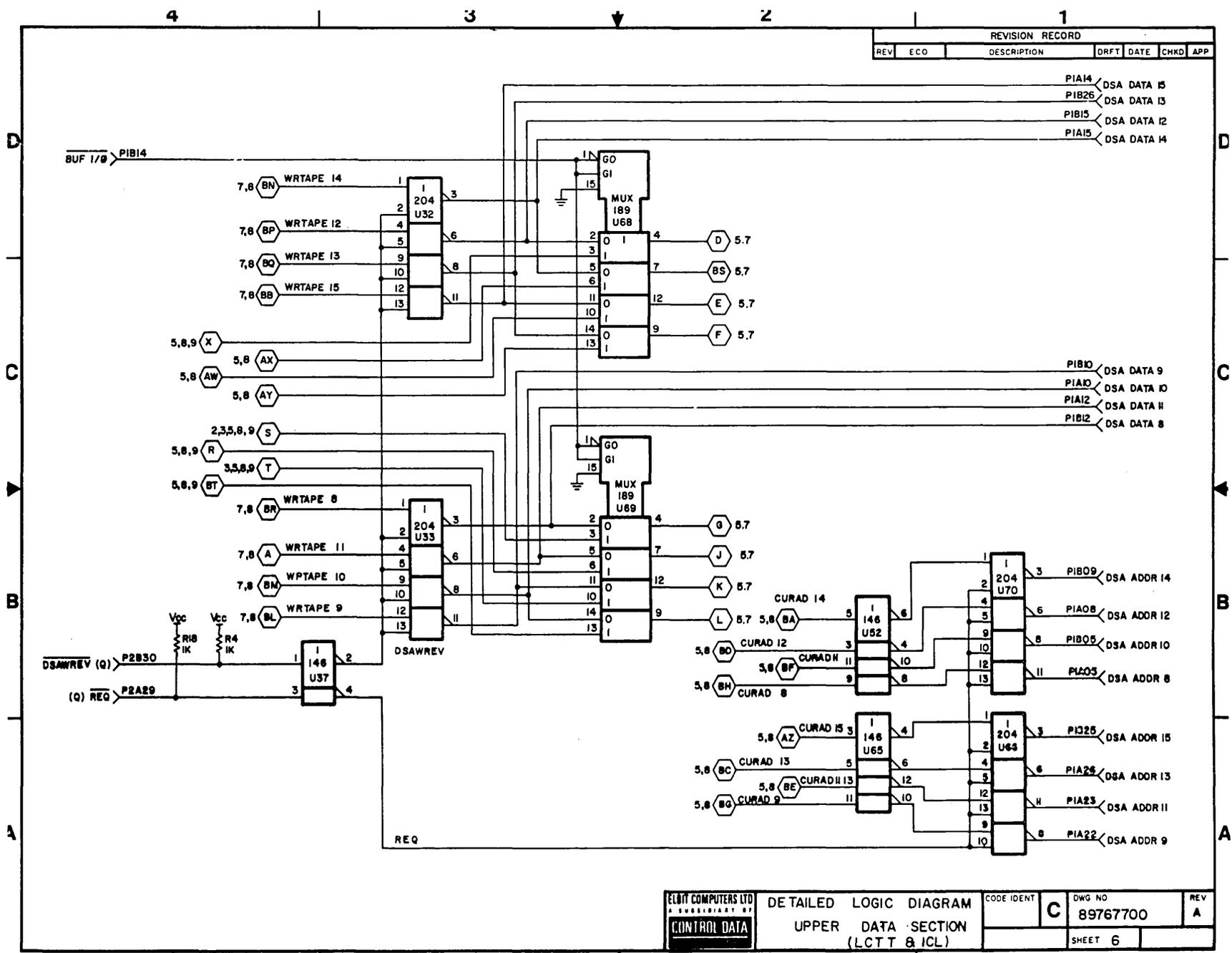
Figure 5-42. Upper Data Section - Upper DSA Data Path Logic Diagram (Cont'd)
