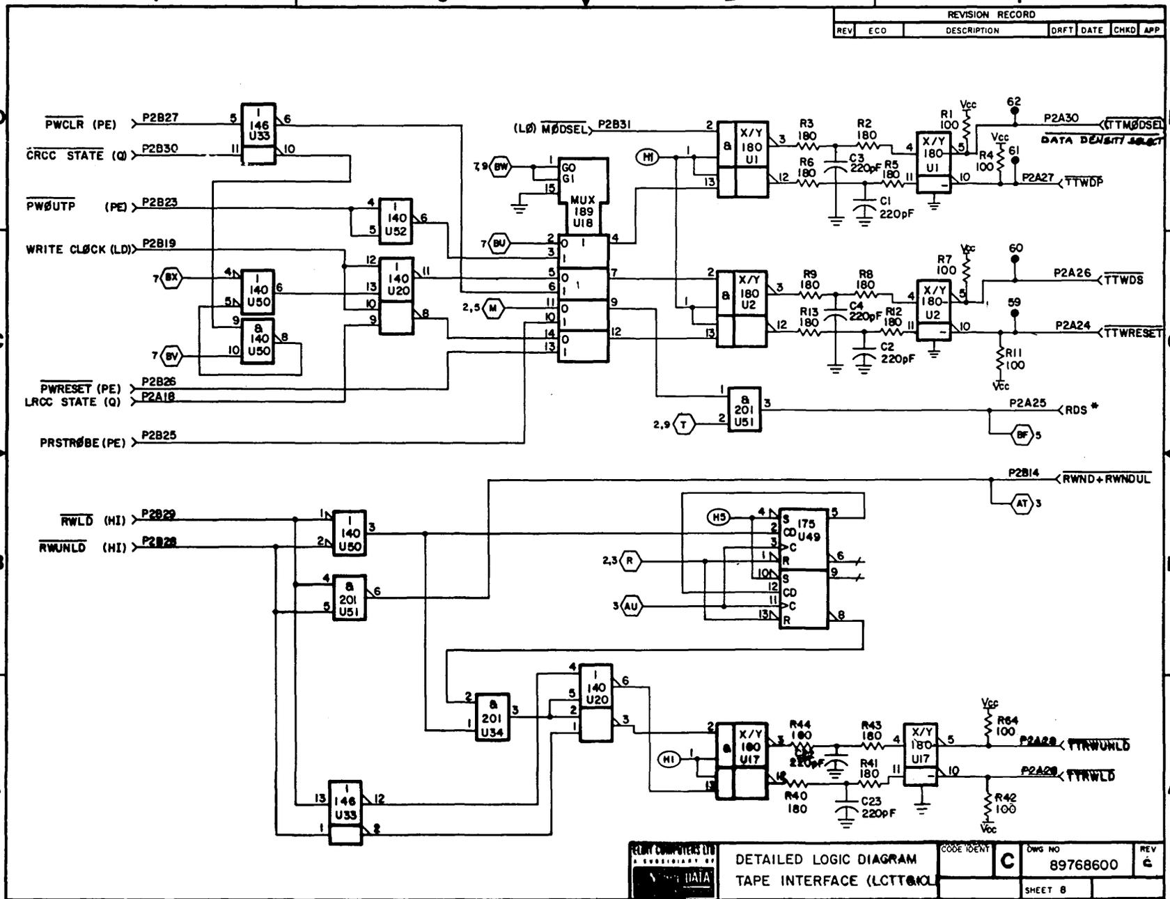
Figure 5-58. Tape Interface - MTT/PE Write Data Path Logic Diagram (Cont'd 2)
