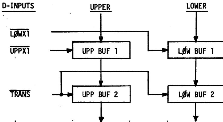
Figure 5-7. Double Buffer Control
