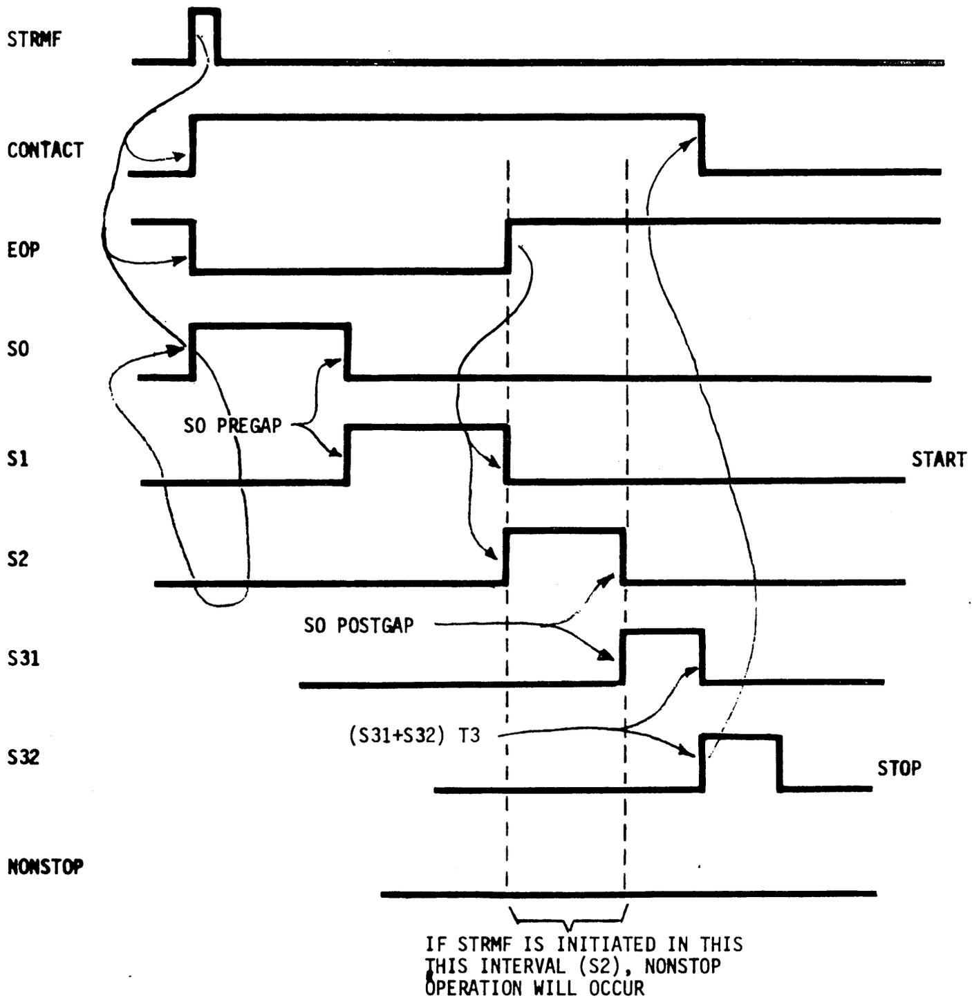
Figure 5-36. Normal Motion Operation
