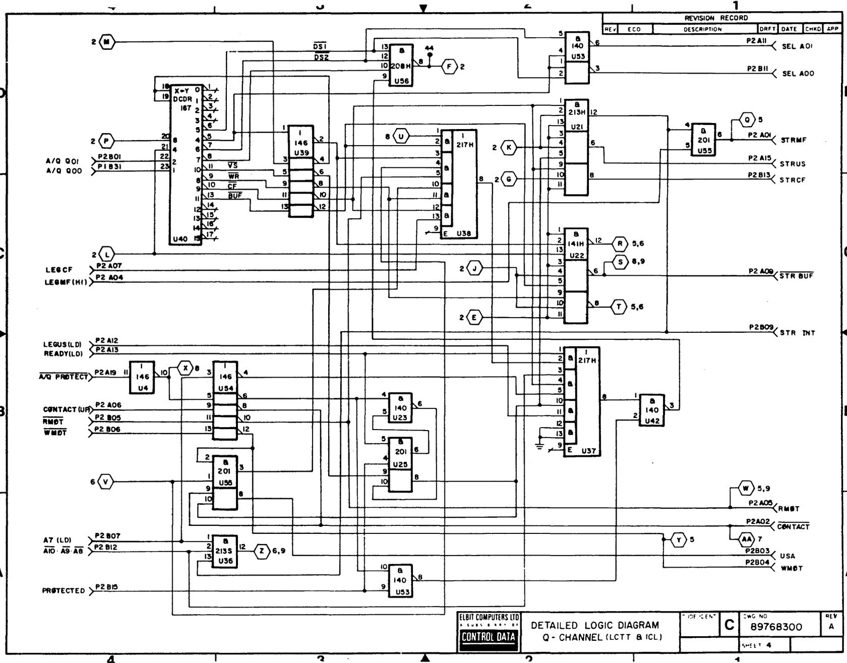
Figure 5-6. Q-Channel - Operation Decoder Logic Diagram (Cont'd)
