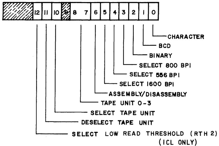
Figure 2-3. Unit Select for A-Register
