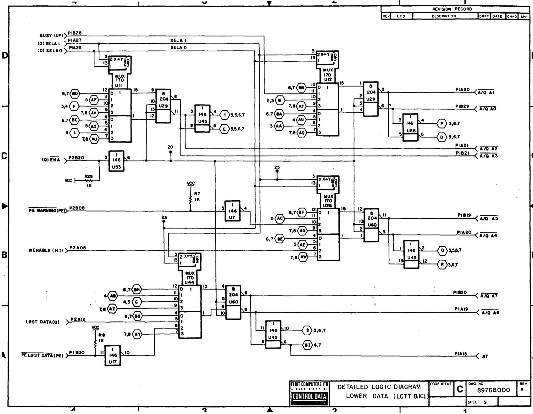
Figure 5-31. Lower Data Section - Lower A Data Path Logic Diagram (Cont'd)
