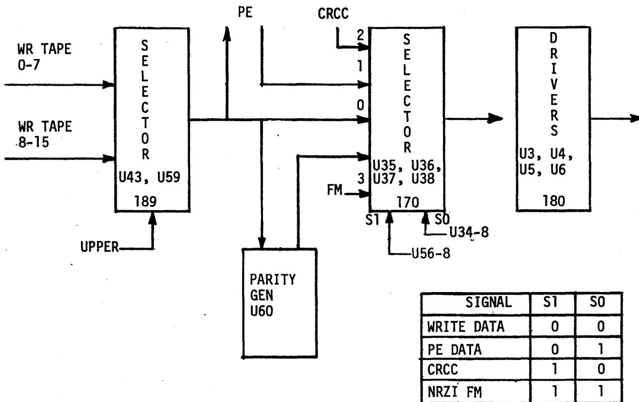
Figure 5-55. MTT/PE Write Data Path
