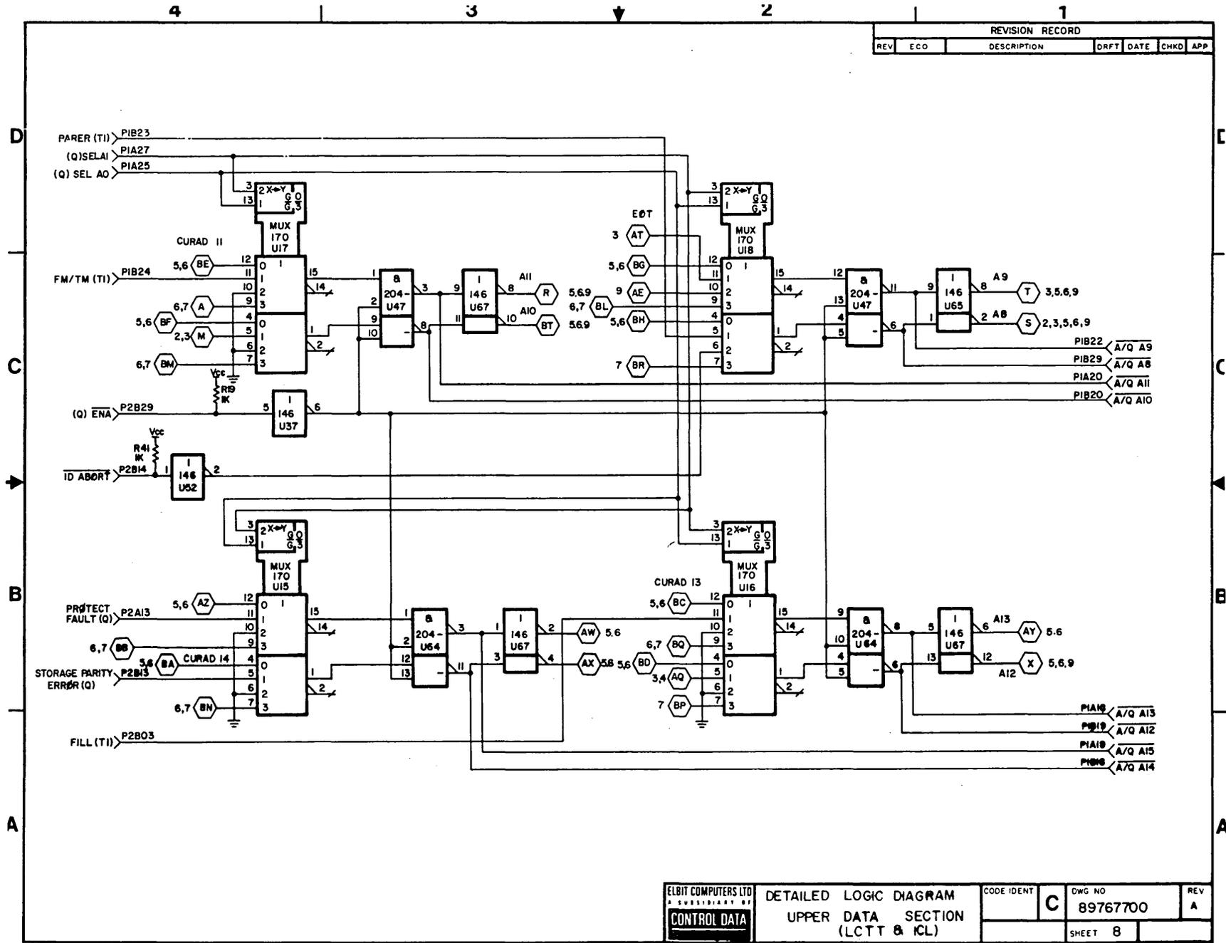
Figure 5-45. Upper Data Section - Upper A Data Path Logic Diagram (Cont'd)
