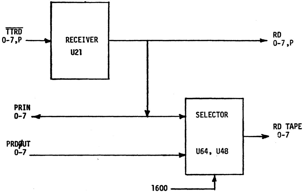
Figure 5-59. MTT/PE Read Data Path
