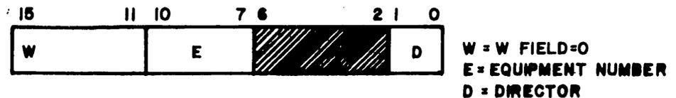
Figure 2-1. Format of Q-Register
