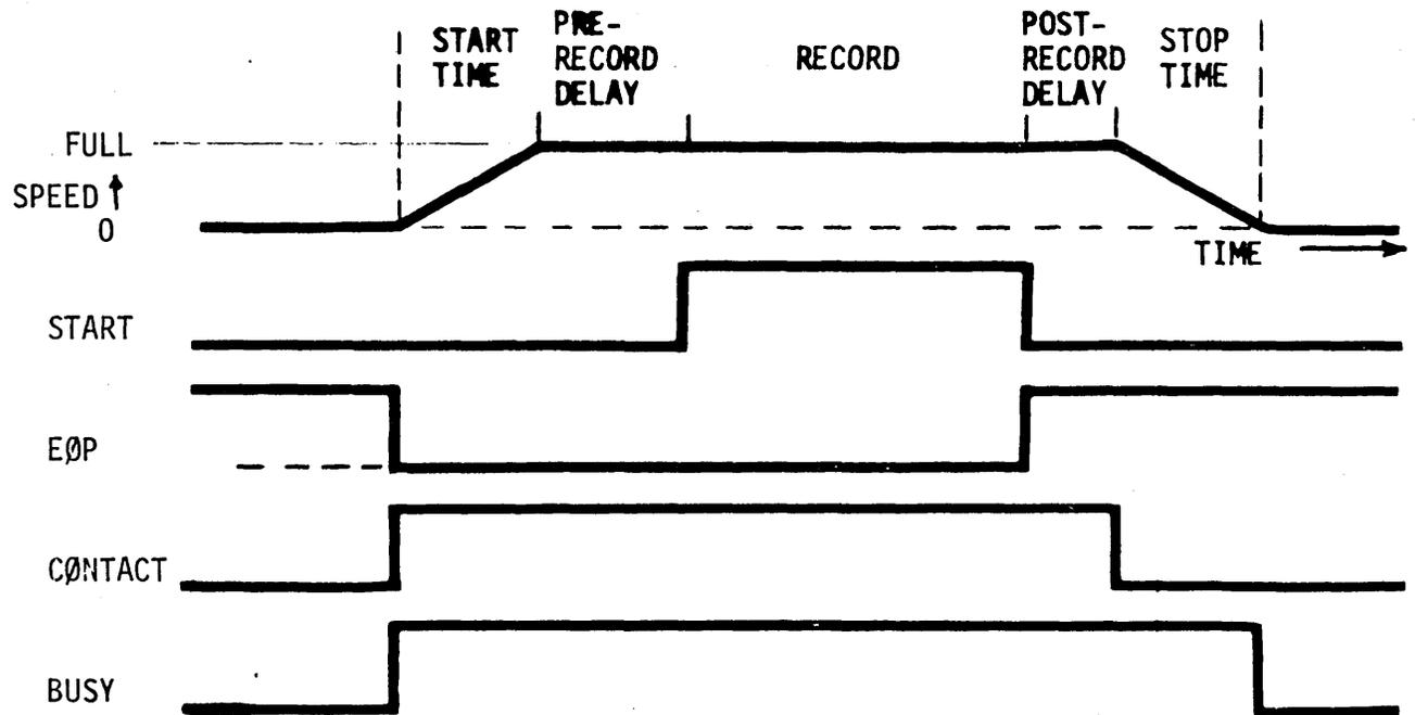
Figure 5-35. Motion Sequencer Control (Single Record Timing)
