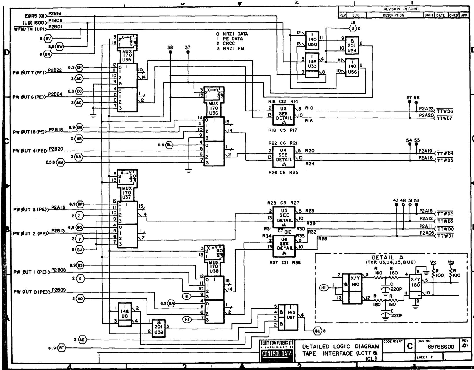
Figure 5-57. Tape Interface - MTT/PE Write Data Path Logic Diagram (Cont'd 1)
