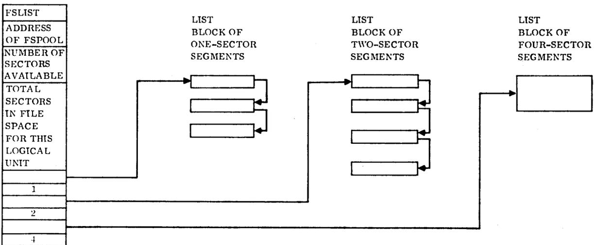
Figure 2-2. Example of File Space Pool and File Space Test
