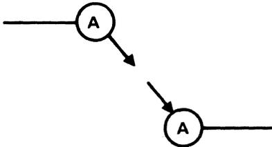
These symbols when used with the logic symbols in the following diagrams indicate that a connection exists between two points on a sheet. The arrows attached to each circle point from signal origin to signal destination. The letters C, H, I, O, and P are not used inside the circles, since they bear special significance on logic diagrams.
