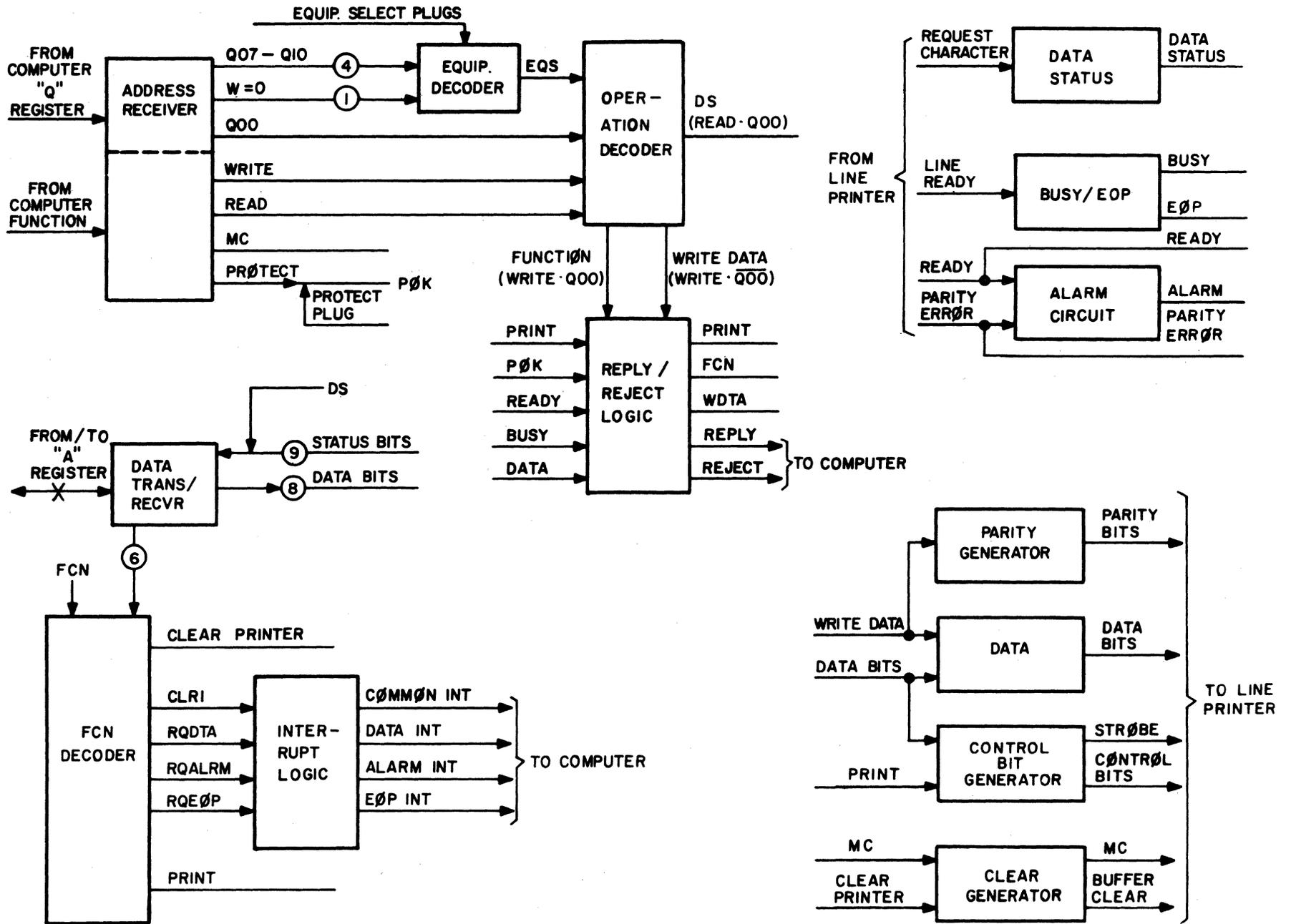
Figure 4-1. Line Printer Controller Block Diagram
