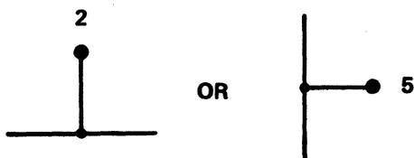
The test point symbol on the logic diagram shows the connection of a test point on the printed wiring board (PWB). The number adjacent to the symbol refers to the test point position on the PWB at the edge opposite the connectors. Only test point 1 is labeled on the edge of the PWB.
