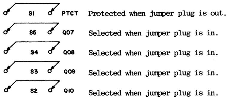
Figure 2-5. Jumper Plug Selection
