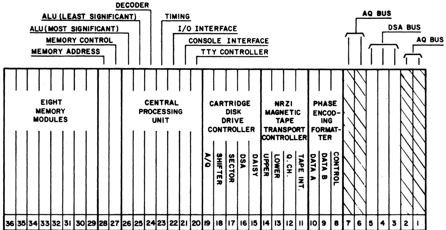
Figure 3-2. Location for Installation of Controller PW Assembly (A/Q Bus)
