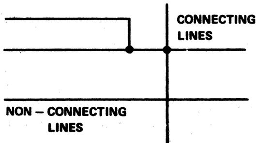
Lines connected to a common point or at a junction point are shown in the upper part of this illustration. No more than four lines are connected to a common point in the diagrams.
