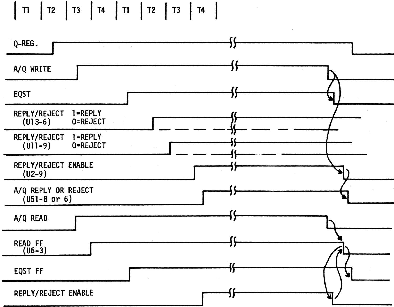
Figure 4-2. A/Q Timing Read/Write
