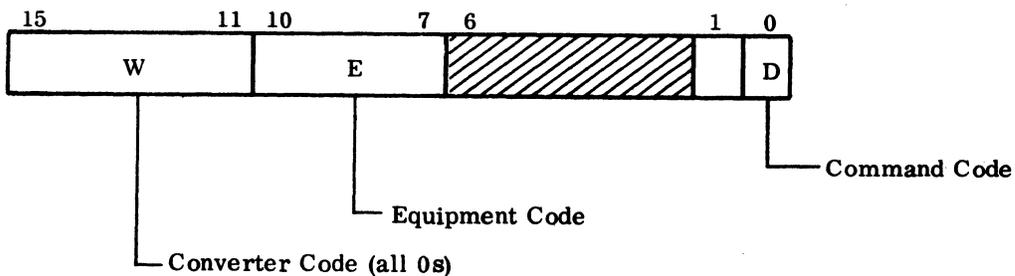
Figure 2-1. Q Register Format
