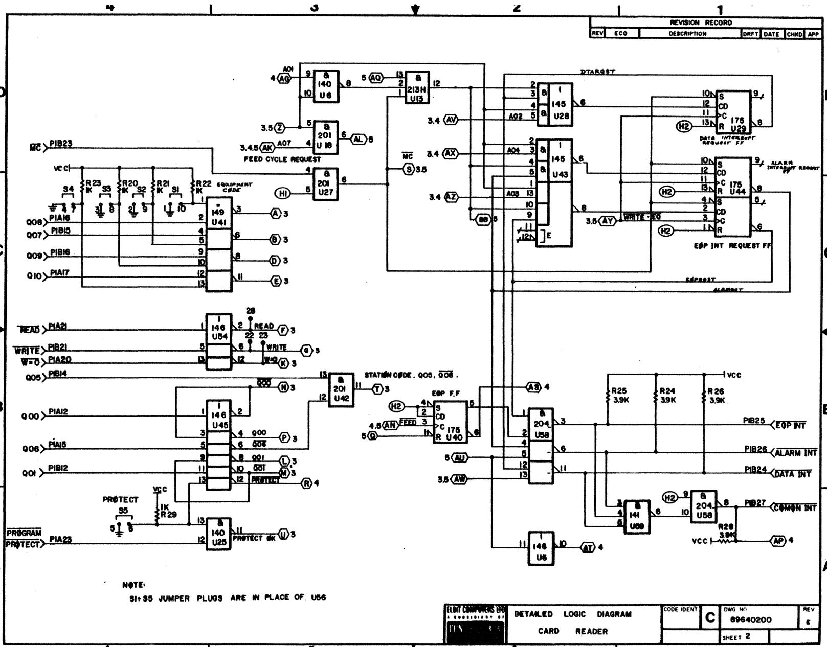
Figure 5-2: CARD READER PWA Detailed Logic Dgm: Interrupt Logic, Q Receivers and Protect Circuitry
