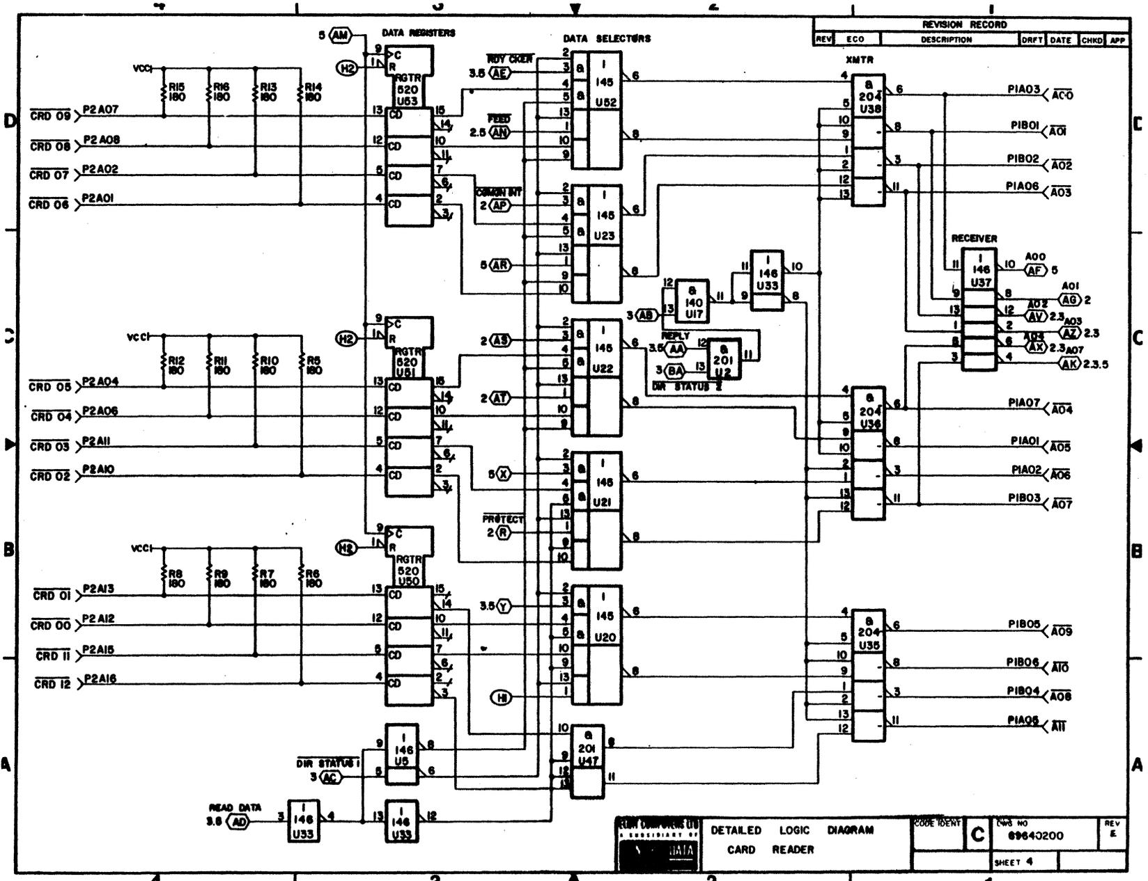
Figure 5-4. CARD READER PWA Detailed Logic Diagram: Data Transfer Logic
