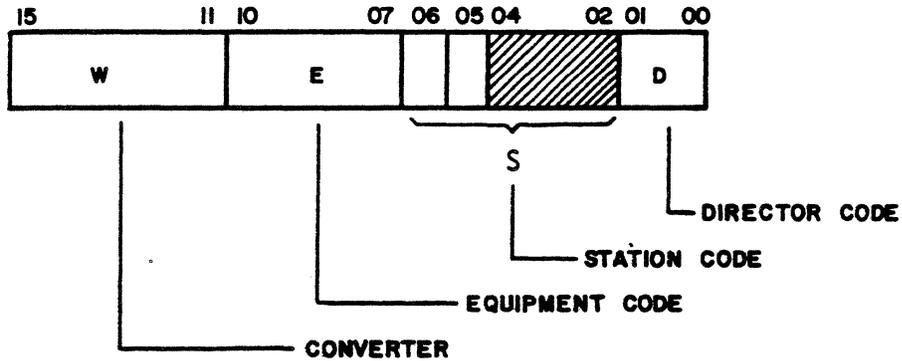
Figure 2-1. Q Register Format
