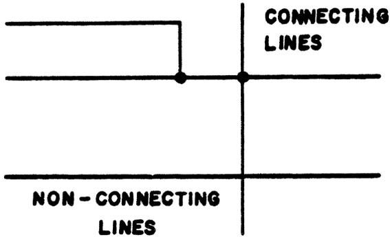
Lines connected to a common point or at a junction point are shown in the upper part of this illustration. No more than four lines are connected to a common point in the diagrams.
