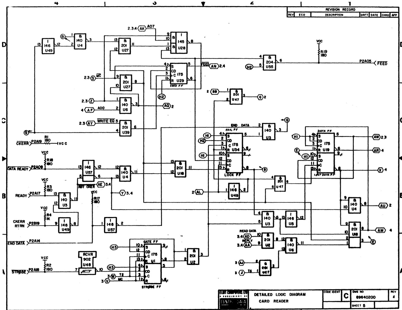
Figure 5-5. CARD READER PWA Detailed Logic Diagram: Card Reader Control Circuit
