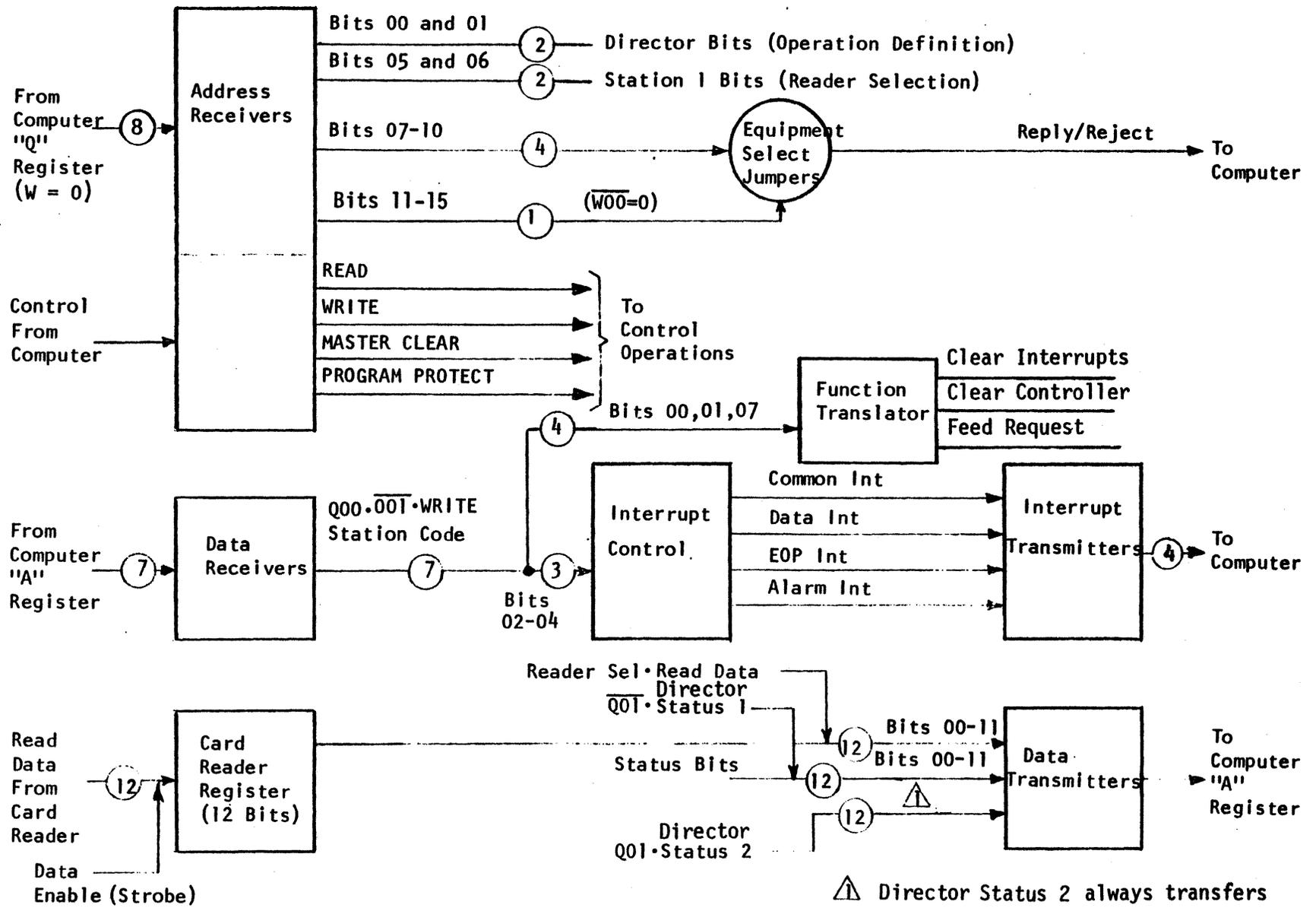
Figure 4-1. Card Reader Controller Block Diagram
