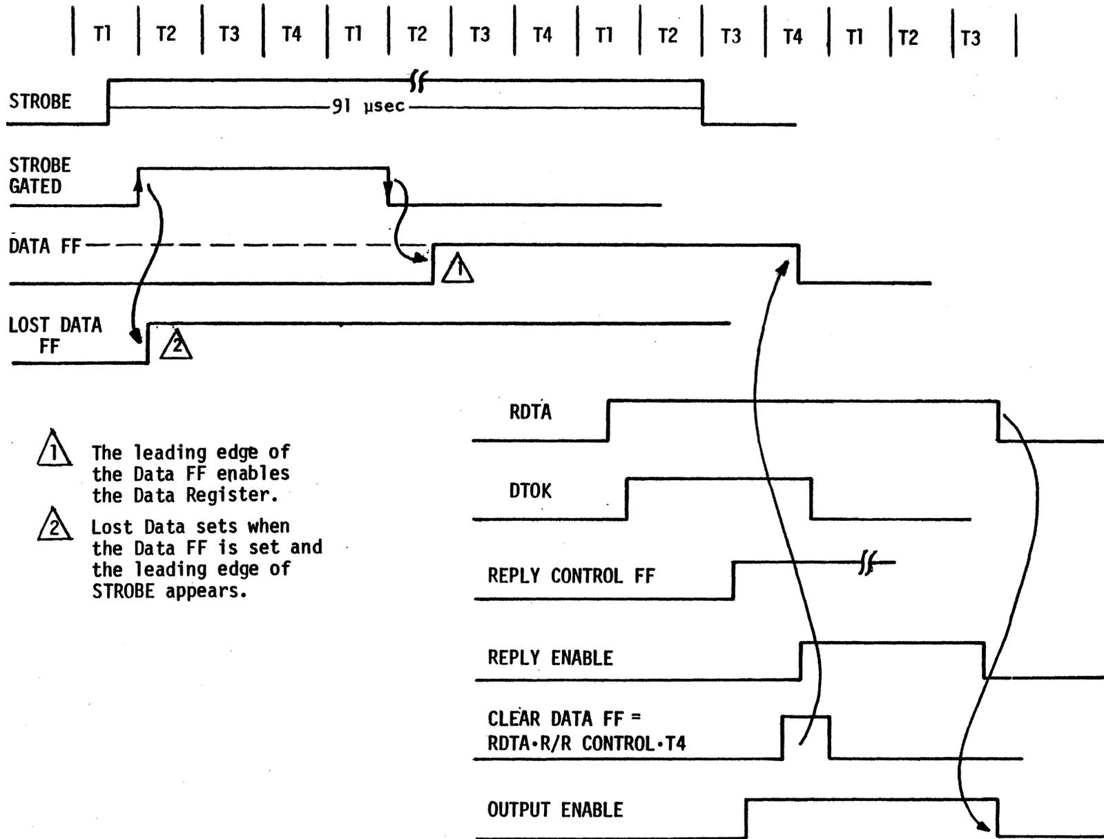
Figure 4-3. Data Transfer Timing Diagram
