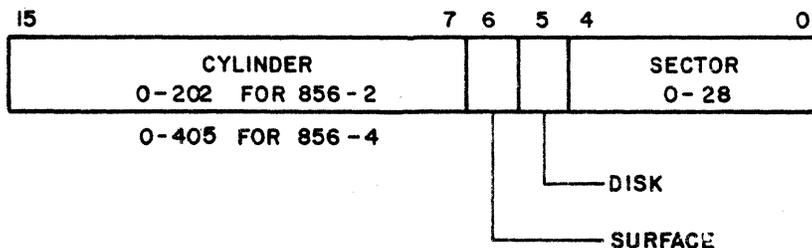
Figure 2-5. Cylinder Address Status Format
