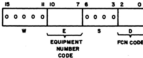
Figure 2-1. Q Register Format
