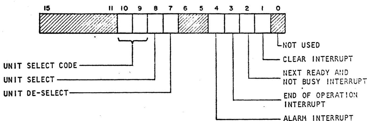
Figure 2-2 - Selectable Interrupt Conditions and Unit Selection
