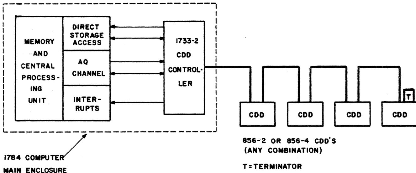
Figure 1-1. System Configuration
