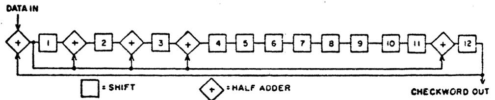
Figure 1-5. Checkword Generation
