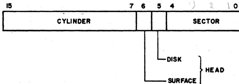
Figure 2-3. Load Address Format
