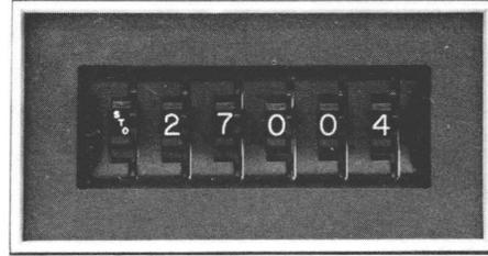
If the READ STO switch on the keyboard is depressed, the contents of memory location 27004 are displayed in the Communication register at a repetition rate determined by the auto step control. (If the memory location depicted by the breakpoint switch exceeds the storage capacity of the system, the computer selects the address that corresponds to the storage capacity of the system.)
