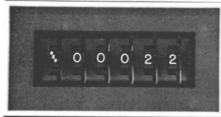
If the READ STO switch on the keyboard is depressed, the contents of register 22 are displayed in the Communication register at a repetition rate determined by the Auto Step control. (Only the lower two digits are of consequence when the REG designator is displayed. In this case register 22, the real time clock, is being referenced.)
