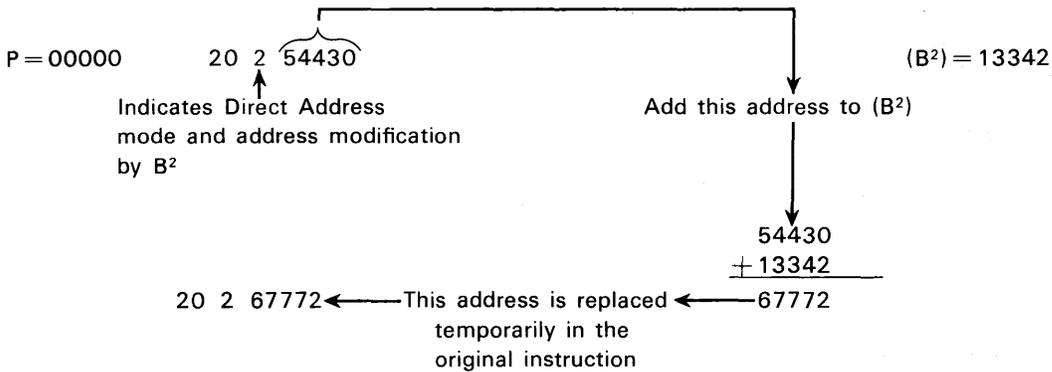
LDA with the 24-bit quantity stored at address 67772
