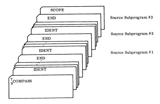
Placement of IDENT and END for assembly of several subprograms with differing COMPASS parameters.
