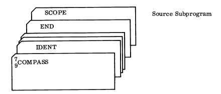
Placement of IDENT and END cards for assembly of multiple subprograms.
