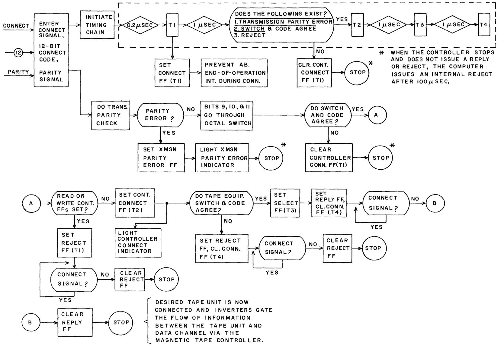
Figure 2-2. Connect Operation
