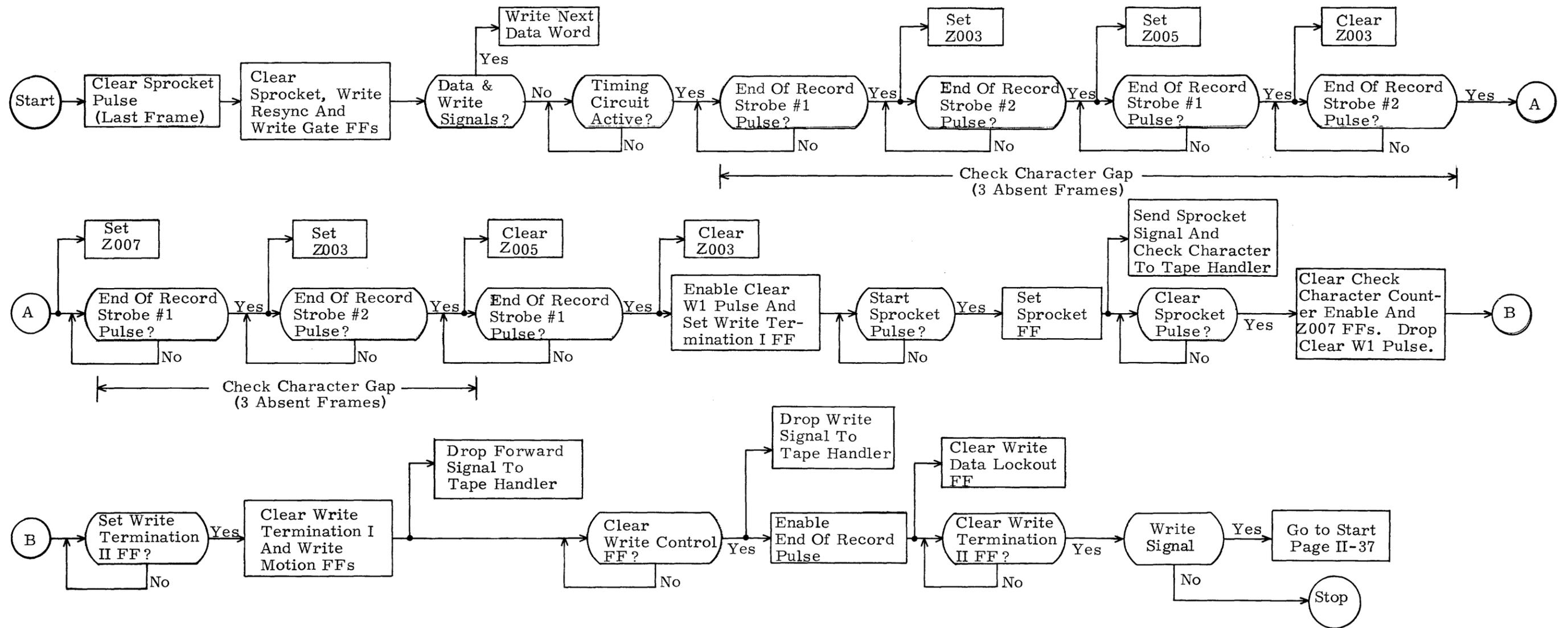
Figure 2-29. Flow Chart: Write Termination
