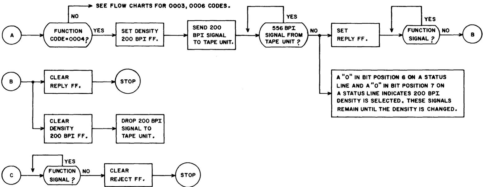
A "0" IN BIT POSITION 6 ON A STATUS LINE AND A "0" IN BIT POSITION 7 ON A STATUS LINE INDICATES 200 BPI DENSITY IS SELECTED. THESE SIGNALS REMAIN UNTIL THE DENSITY IS CHANGED.
