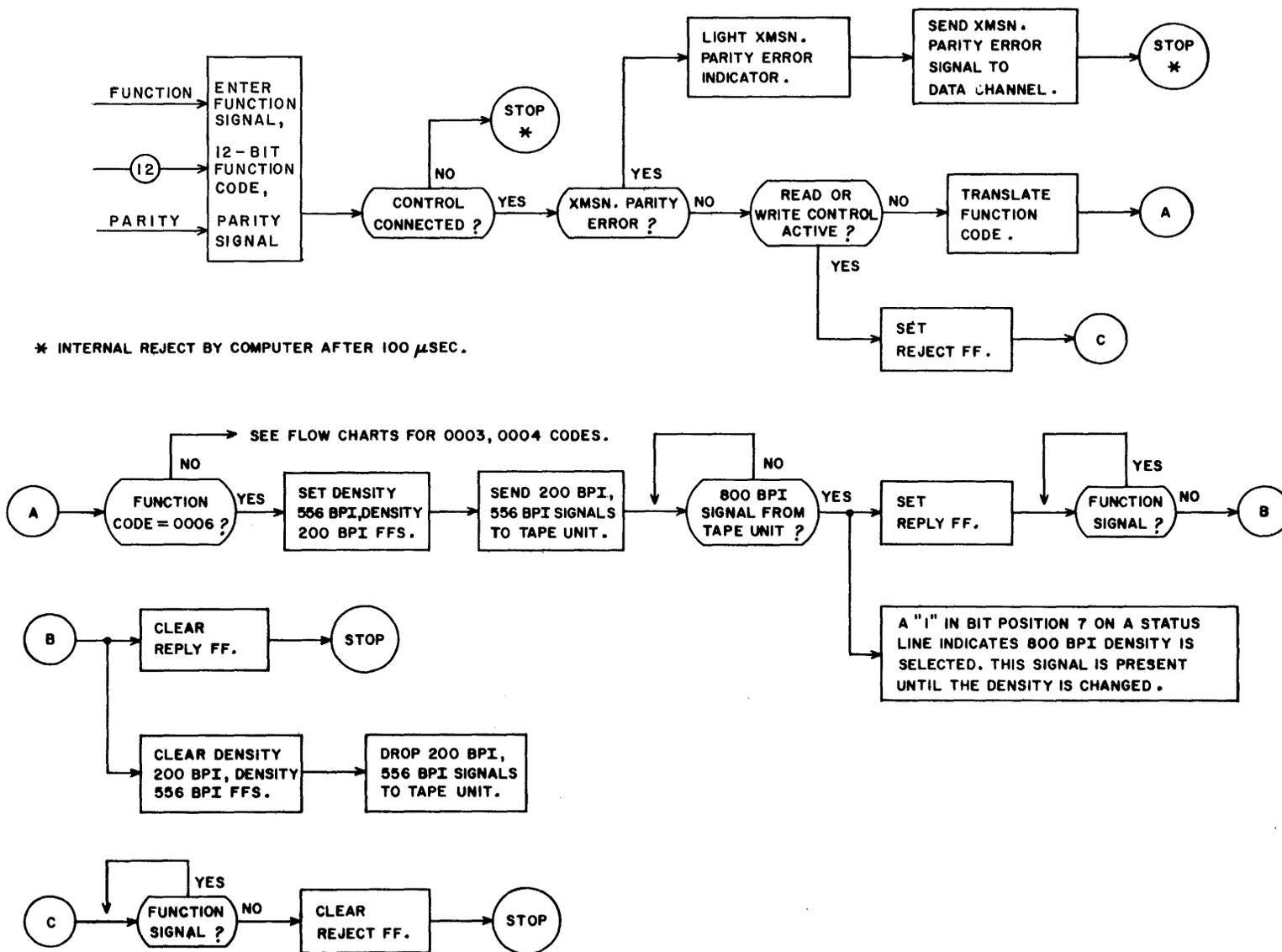
Figure 2-16. Tape Motion Signals
