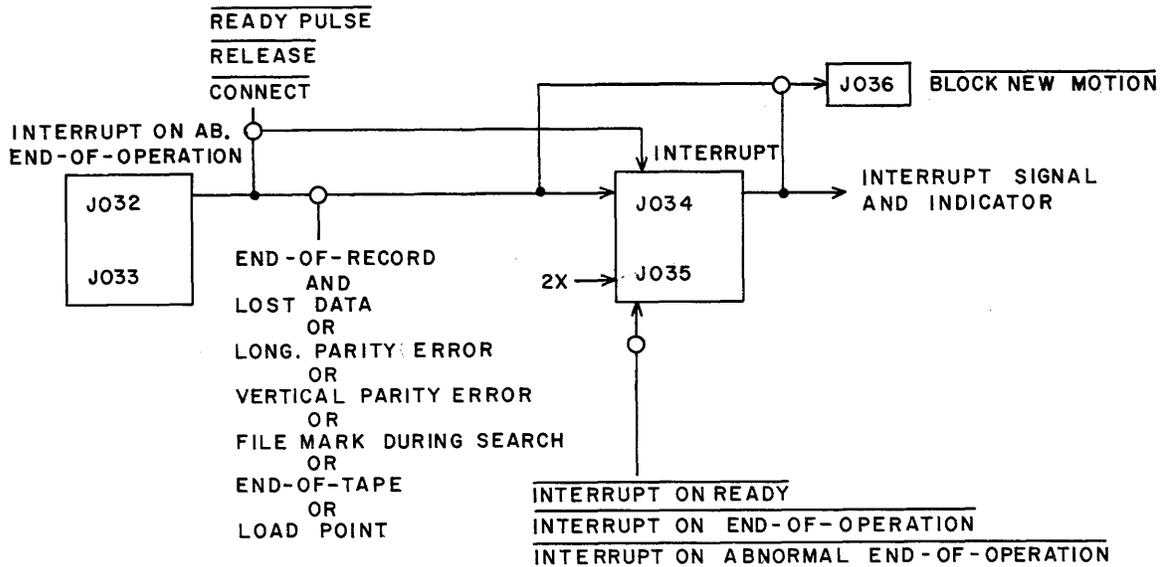
Figure 2-44. Interrupt on Abnormal End of Operation
