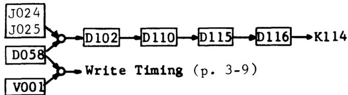
The Density Reply from the transport will enable one of three oscillators which control the frequency at which frames are written. The oscillator control the Write Timing Chain.
