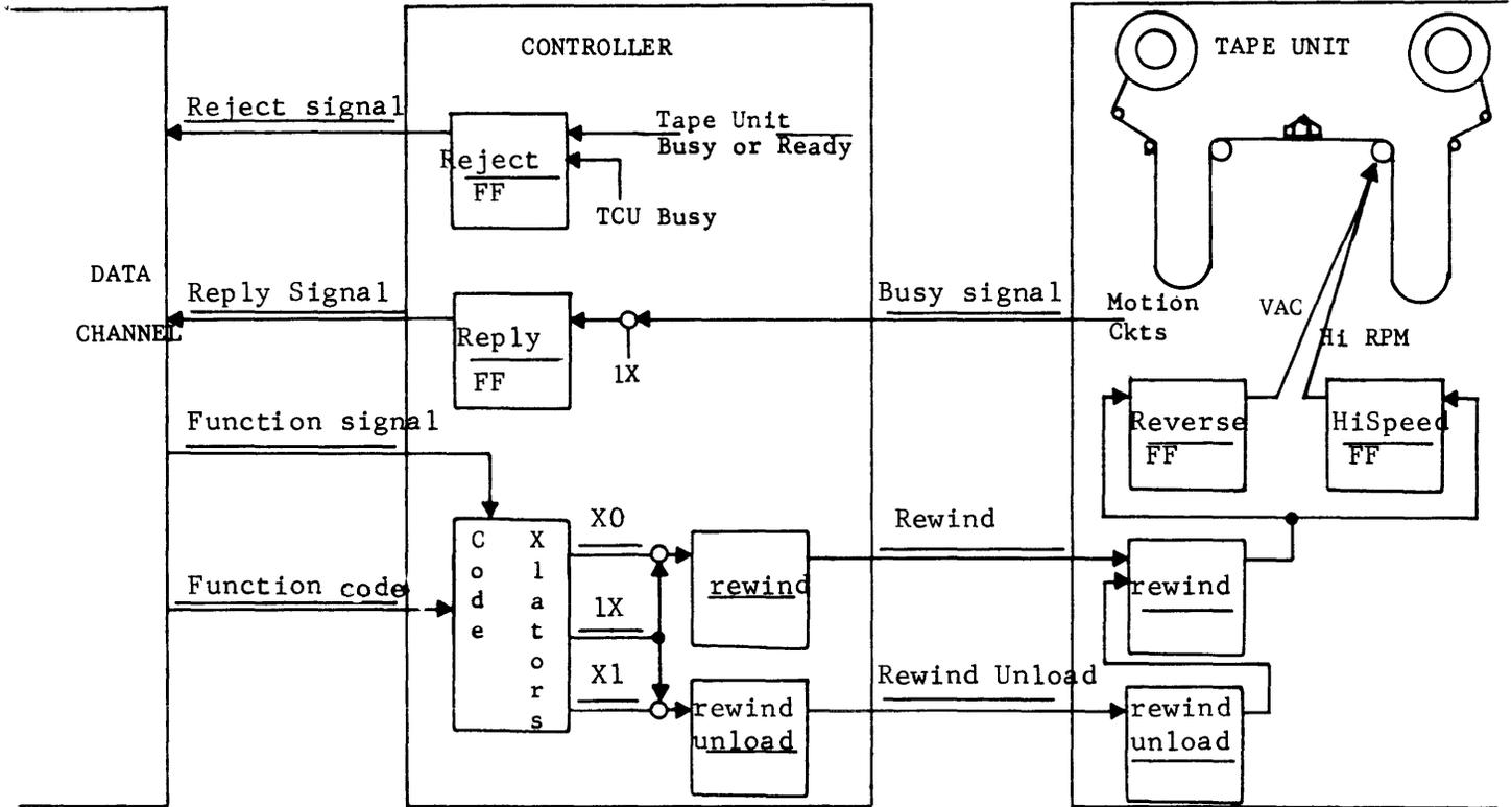
2. Describe the differences between a Rewind and a Rewind Unload Operation.
