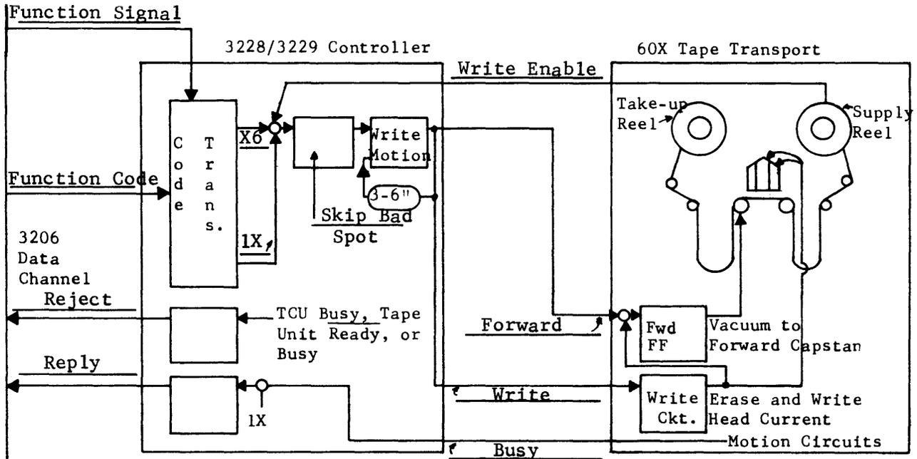
2. Would a "Write" Signal be sent to the selected tape transport if it is not ready? If no, explain what prevents it? If yes, how does the signal affect the transport? Give a detailed explanation.
