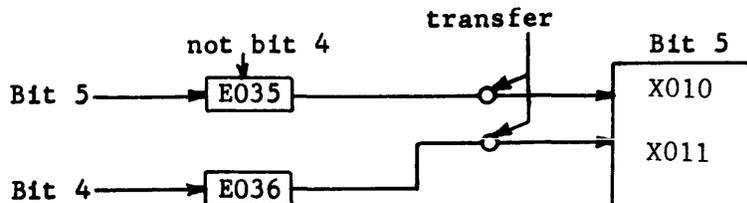
The external BCD code of an octal 12 must be converted to an internal BCD code of 00. This can be accomplished by detecting the presence of an octal 12 and preventing bit 1 and bit 3 flip-flops from setting.
