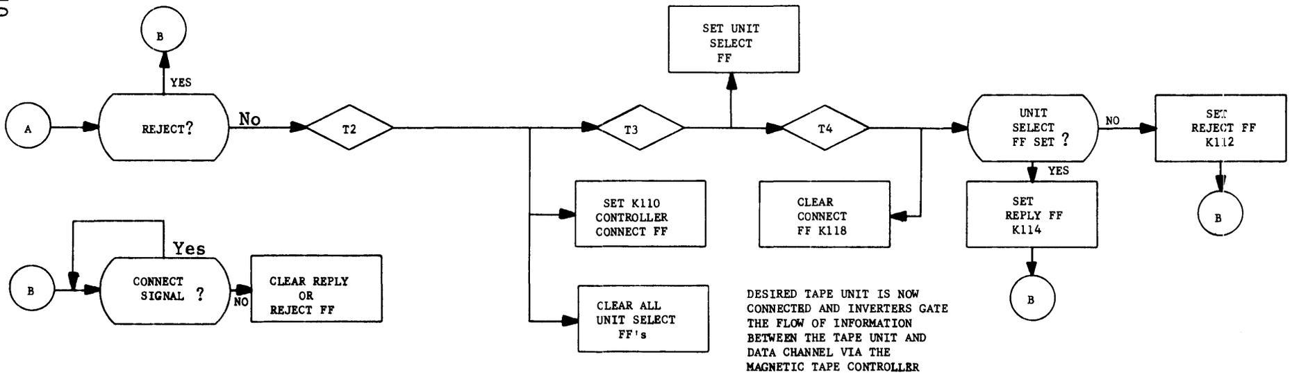
Figure 2-1. Connect Operation
