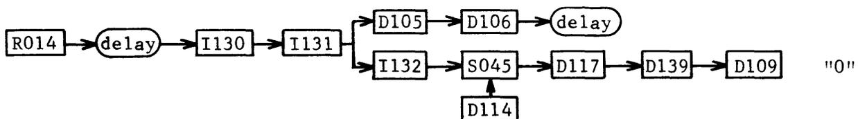
For the Format Functions 01 or 02 S045 and S040, translate bits 3, 4, and 5 only. Bits 0, 1 and 2 are translated by S010 thru S016 (page 3-3).
