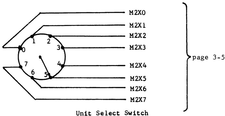
The lower 3 bits--bits 0, 1, and 2--from the Connect Code have been translated through the Tape Unit Select Inverter (page 3-3) one of which will have a logical "1" output. In the preceding example, for a correct comparison, S035 should be a "1" and be fed to eight AND gates, one at the output of every M2X5 card (page 3-5) where the actual comparison should occur.
