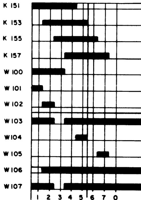
Times 0 through 7 are assigned to these enables (W100-W107) for ease in referring to them.
