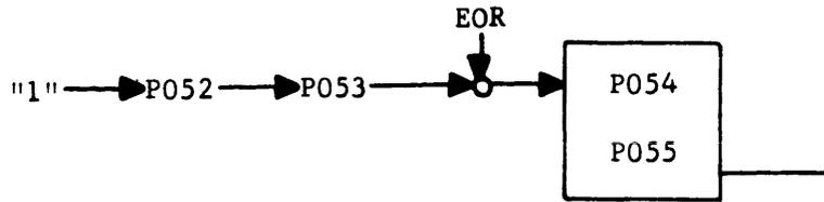
Each frame read back to the controller, except the Check Character, is checked for vertical parity error. The parity checker (p. 3-19) can be looked upon in the same way as the parity generator. Data from the N cards is fed into the checker. The determination made is: Is there an even number of bits in the six information bits of the frame? If the total is even, inverter P026 outputs a logical "1".
