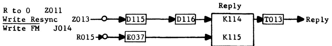
The Reply signal received in the channel causes the data signal to drop, clearing the Reply FF and dropping the Reply signal.
