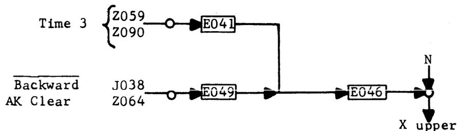
The information received has, at this time, passed through the parity checker, and vertical parity will be checked. A parity error will cause the Vertical Parity Error F (P050/051) to set. The error conditions are those that were discussed in Read Reply during Write.
