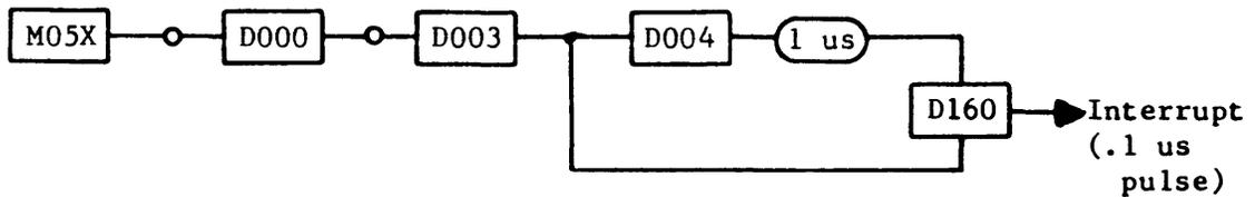
The Ready is lost during the Clear or Release functions, but the interrupt is prevented from occurring during the execution of these functions.
