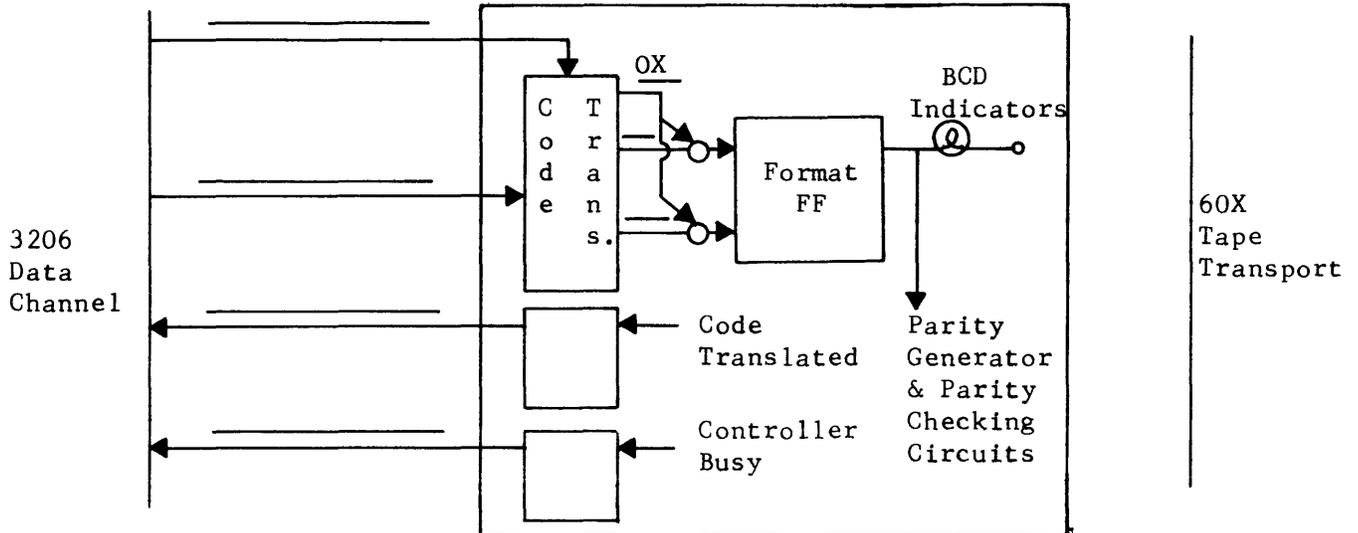
2. The format selection determines whether an odd or even number of bits shall be exchanged between controller and Tape Transport, and controller and channel. T      F
