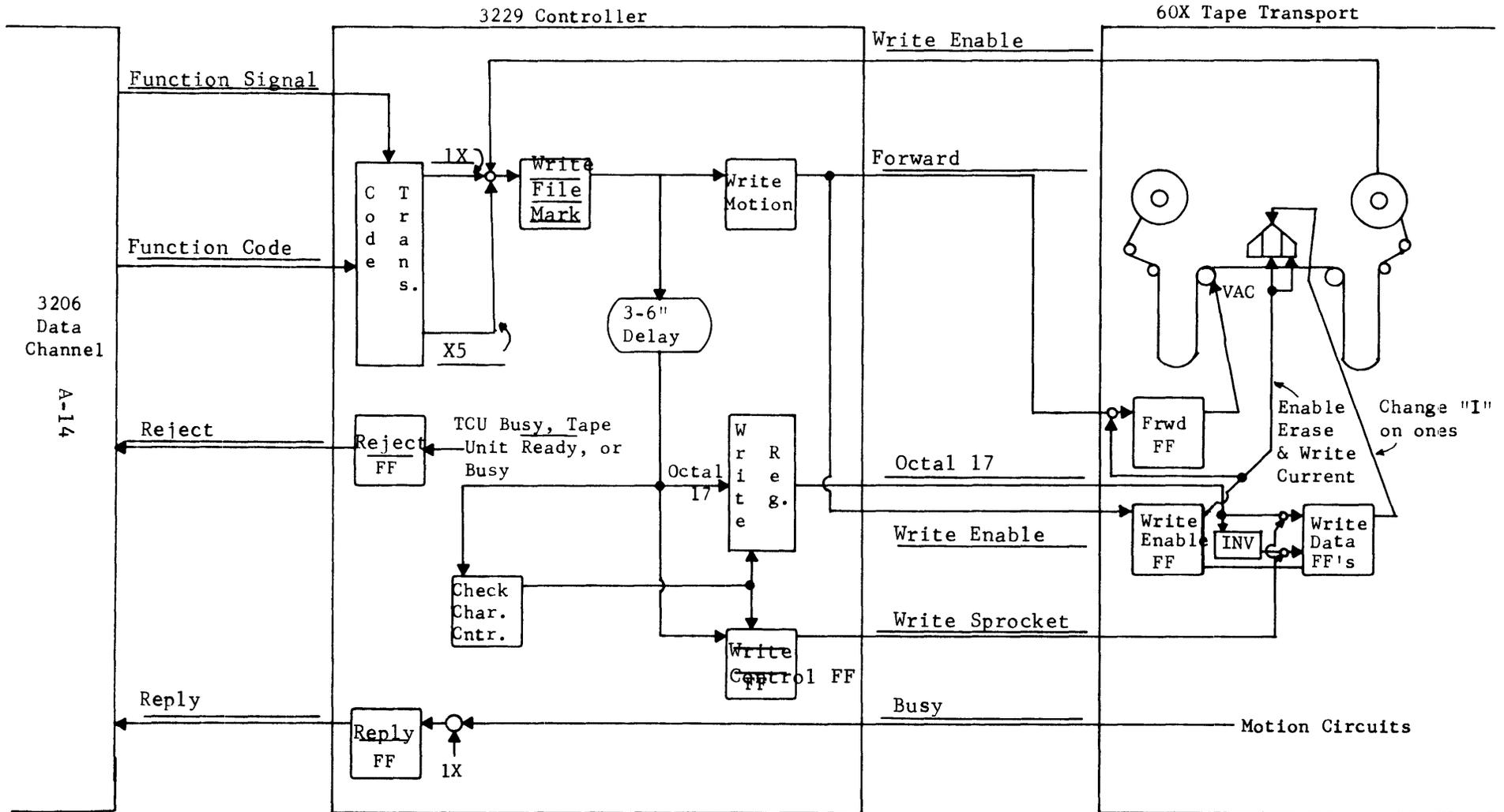
2. How can the same three Write oscillators operate 75 as well as 150 inch per second Tape Transports?
