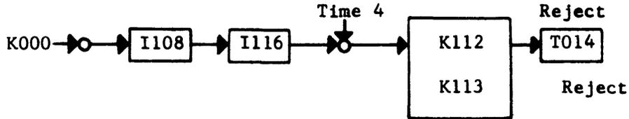
At time 4, K118/119 (Connect FF, p. 3-3) is cleared. The conditions for an Abnormal End of Operation Interrupt no longer exist.
