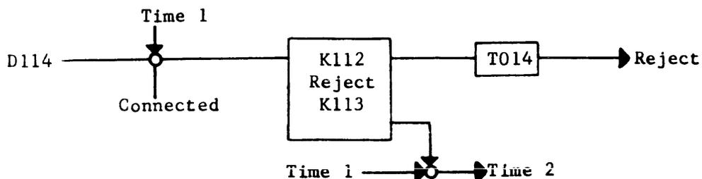
The Reject Signal returned to the channel causes the Connect Signal and Code to drop.
