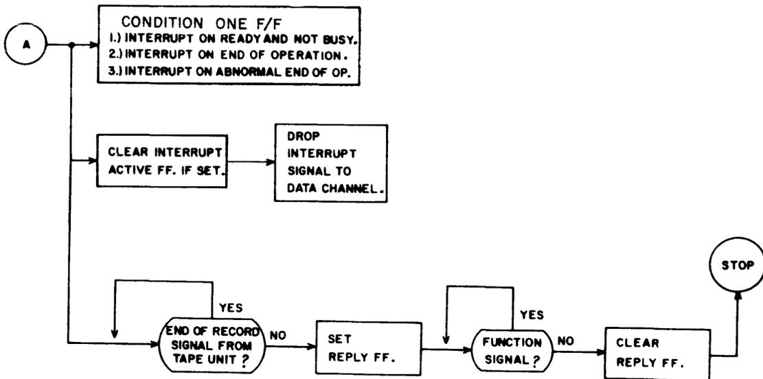
Figure 2-26. Select Interrupt Condition
