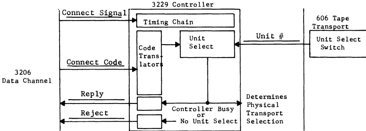
2. The channel sends the Connect signal to start the Connect Timing Chain.
