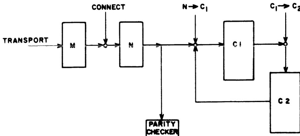
When Write Motion (Z020/021) sets and before Write Control sets, the C register is cleared.
