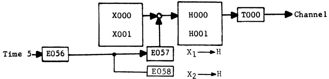
The enabling term, E057, will also set the Hold FF (Z094/095). This flip-flop is used to detect a Lost Data condition.
