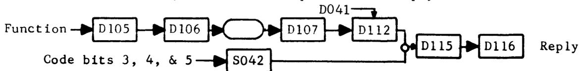
The Reply causes the Function signal and Code to be removed from the channel clearing the Reply FF and ending the Operation.
