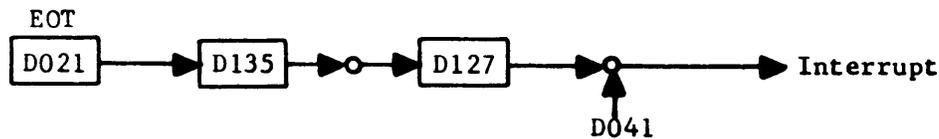
This indicates that another operation in a Forward direction should not occur due to the risk of dropping the tape leader from the supply reel and thereby creating a fault condition in the handler.
