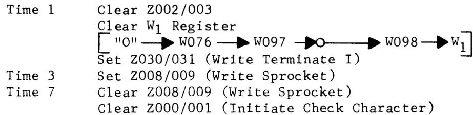
The Check Character is now on tape and the controller must revert to its static state. At Time 1 the Write Terminate FF was set. A time delay must elapse during which time the tape moves into the record gap. When this delay ends, Write Terminate I and Write Motion FFs. clear. Write Motion clearing causes the Forward signal to the transport to drop.
