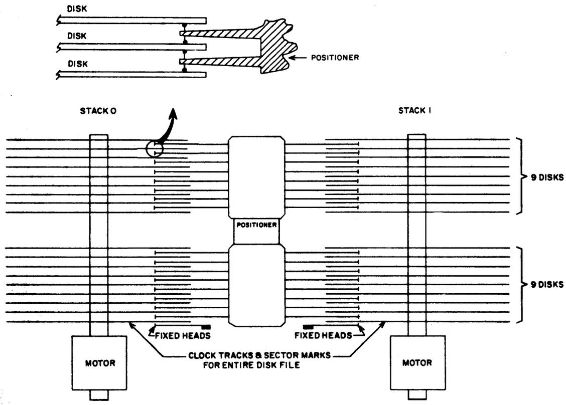
Figure 1-5. 821-1 Disk File Access Mechanism
