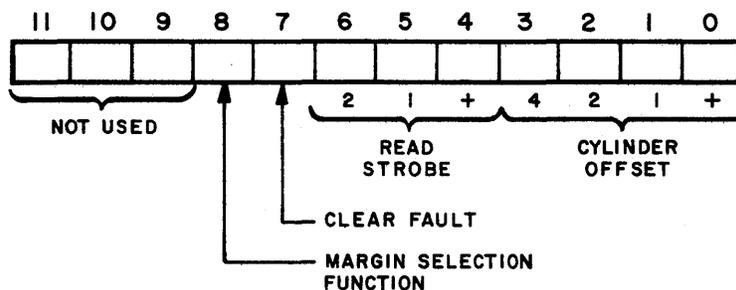
Figure 2-2. Margin Selection Code Bit Assignments
