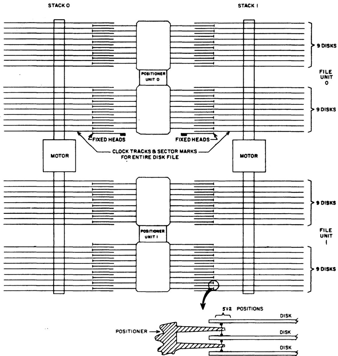
Figure 1-6. 821-2 Disk File Access Mechanism
