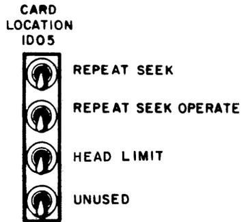
Figure 3-1. Maintenance Panel and Controls
