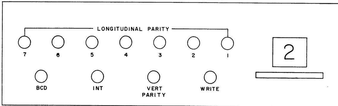
Figure 2.. 322X Equipment Number Switch and Indicator Panel\*\*
