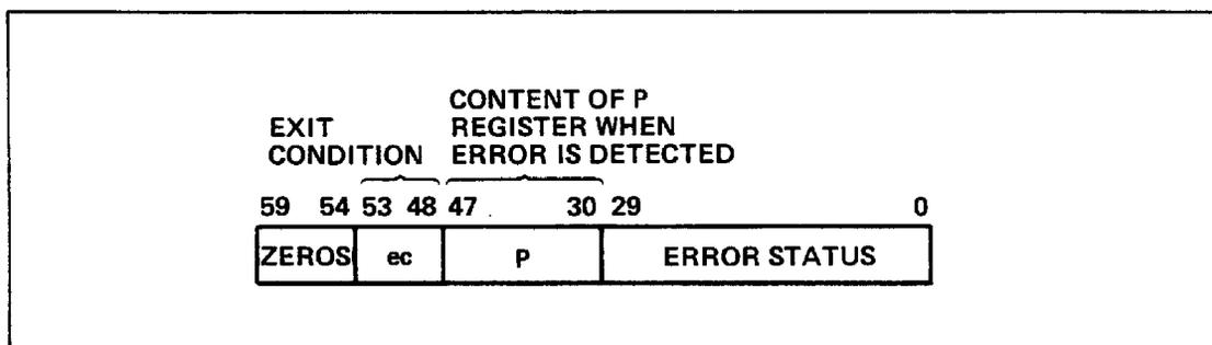
Figure 5-5. Format of Exit Condition Register at (RAC)
