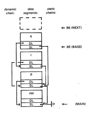
The stack, growing upwards, originates from the calling sequence: RTST  $\longrightarrow P \longrightarrow R \longrightarrow Q$ . BASE is the base address of the most recently created data segment. It is the head of the chains. NEXT defines the base address of the next data segment to be stacked.
