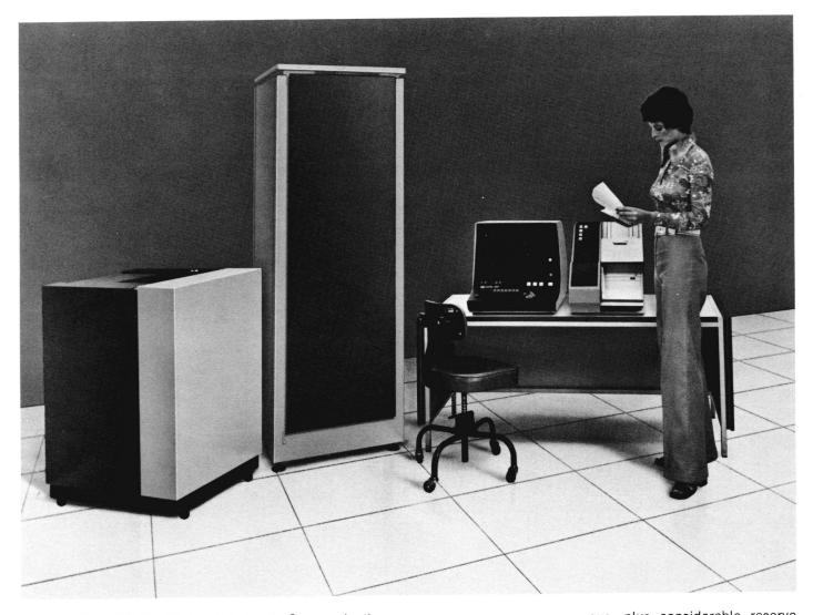
The CDC® CYBER 170/2550-1 Host Communication Processor (HCP) is the entry-level system of the CDC 2550 series and is designed for use with small Network Communication Systems (NCS). The primary function of the HCP within this network is to combine the interfacing functions of host computers and terminals into a unitized product package. The HCP also assumes various data-communications-related functions formerly residing in the host computer, and results in greater host computer efficiency.
