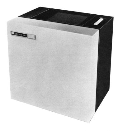
The CONTROL DATA 2570-1 Line Printer and Controller is an inexpensive and highly reliable, 300 lpm printout device. This printer is connected to the CDC 255X Series Host Communication Processor via a single printed-circuit board controller/adapter which can be plugged into any Interrupt Data Channel position in the computer's main or expansion enclosure.
