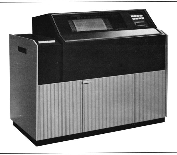
The CONTROL DATA 2570-2 Line Printer and Controller features an acoustically-dampened cabinet and enclosed stacking. Quiet operation is an outstanding feature of this printer, allowing its use in normal office environments.
