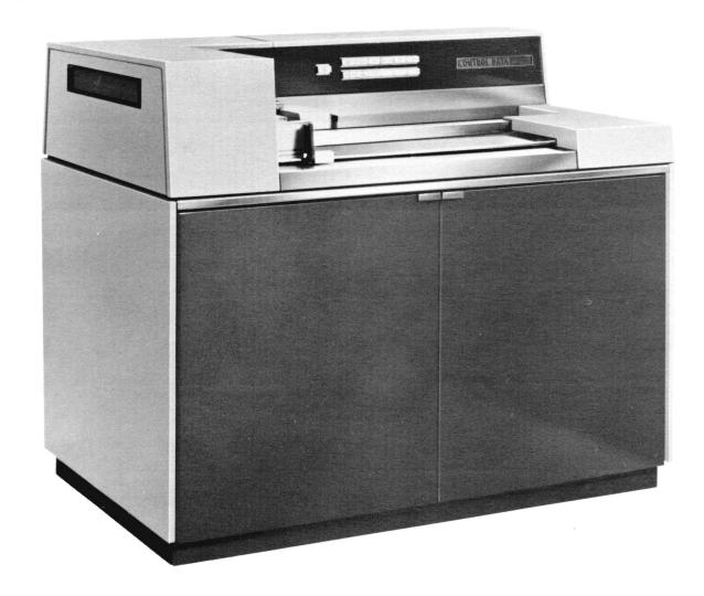
The CONTROL DATA 405 Card Reader is one member of a large family of peripheral products. This unit reads 80-column cards at the rate of 1200 cards per minute, and 51-column cards at 1600 cards per minute.
