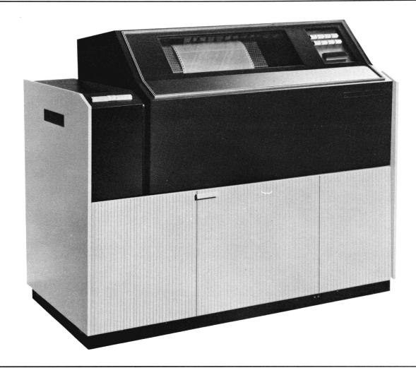
The CONTROL DATA 580 Series of Line Printers is a complete printer family featuring 1200, 1600, and 2000 line-per-minute operation, an acoustically-dampened cabinet, enclosed stacking, and extended-font print capability. Quiet operation permits use of the printer in an office environment.
