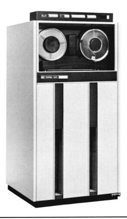
The Control Data 667 Series Magnetic Tape Transports are 7-track members of a new CDC® tape transport family. These units have been specially developed to provide high levels of performance, reliability and maintainability, based on the latest technology.
