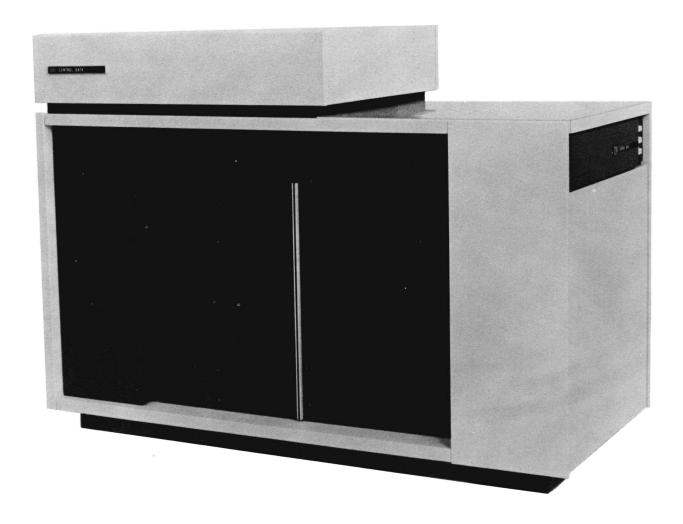
The CDC® 7077-1 Communications Station is used in conjunction with the CDC 791-1 Communications Subsystem Controller to increase the variety and volume of communications traffic to and from a CDC CYBER 70<sup>TM</sup> Series or a 6000 Series Computer System. The interface between the CDC CYBER 70 or 6000 computer is via a dedicated I/O channel and one dedicated PPU.
