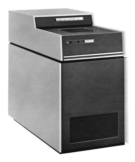
The CONTROL DATA Model 844-21 Mass Storage Subsystem consists of up to eight 844-21 Disk Storage Units with associated single or dual 7054 or 7654 Storage Controllers. This provides a large-capacity, multi-access storage subsystem, using removable disk packs. Each drive has a usable capacity of 708 million bits; a full subsystem with eight on-line drives has a capacity of 5.7 billion bits. Additional data may be stored off-line using Model 881 Disk Packs.
