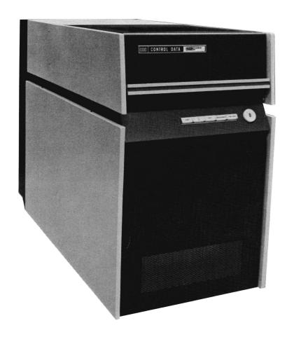
The CONTROL DATA Mass Storage Subsystem consists of up to eight 844-2 Disk Storage Units, with associated single or dual 7054 or 7654 storage controllers. This provides a large-capacity, multi-access storage device, using removable disk packs. Each drive has a capacity of 708 million bits, and an expanded subsystem with eight on-line drives, has a capacity of 5.7 billion bits. Additional data may be stored off-line, using Model 872 Disk Packs.
