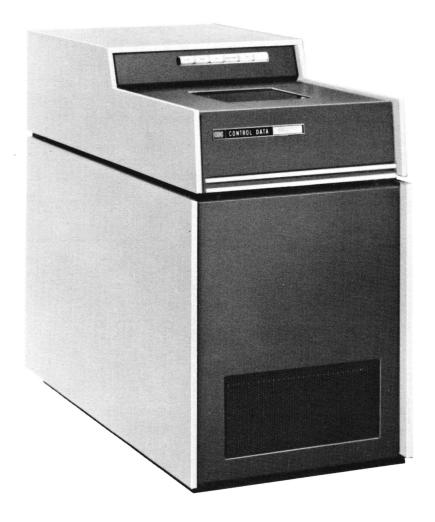
The CONTROL DATA Model 844-41 Mass Storage Subsystem consists of up to eight 844-41 Disk Storage Units with associated single or dual 7054-41, -42 Storage Controllers. This provides a large-capacity, multi-access storage subsystem, using removable disk packs. Each drive has a usable capacity of 1422 million bits; a full subsystem with eight on-line drives has a capacity of 11.4 billion bits. Additional data may be stored off-line using Model 883 Disk Packs.
