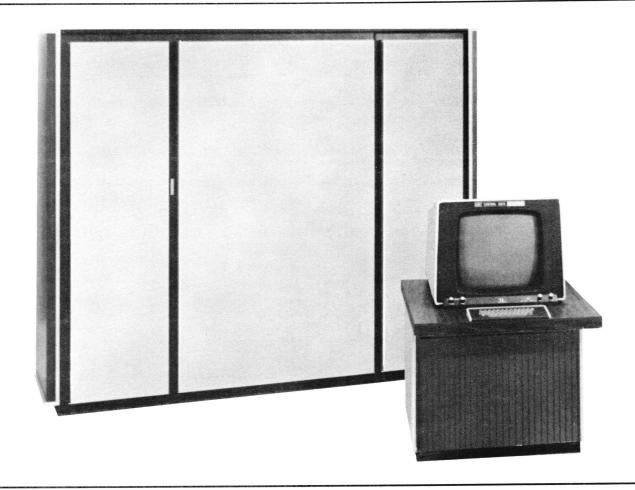
The Model 172 is the smallest system of the CDC® CYBER 170 family of compatible computers. This system can be used as a central computer for batch operations and/or as the nucleus for networks of interactive terminals. It is suitable for data management applications, scientific computation, commercial data processing and data communications. Due to hardware and software compatibility among all CDC CYBER 170 systems, Model 172 serves as an expandable base for long-range growth plans.
