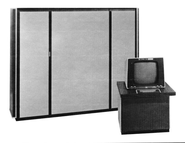
The Model 173 is the intermediate-sized system of the CDC® CYBER 170 family of compatible computers. This system can be used as a central computer for batch operations and/or as the nucleus for networks of interactive terminals. It is suitable for data management applications, scientific computation, commercial data processing and data communications. Due to hardware and software compatibility among all CDC CYBER 170 systems, Model 173 serves as an expandable base for long-range growth plans.
