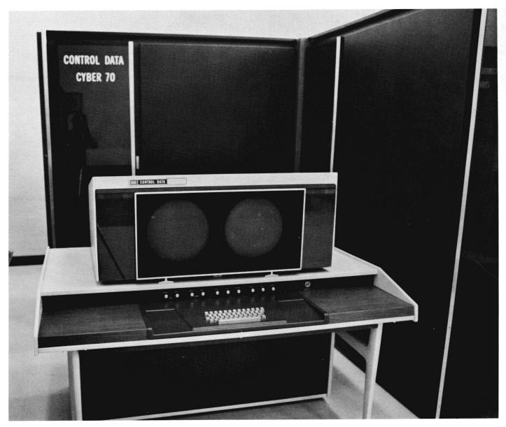
The CONTROL DATA CYBER 70 Series/Model 73 is a general-purpose computing system which provides multiprogramming and multiprocessing capability for scientific, commercial, and data-management applications. The Model 73 is also suitable for communications-oriented applications supporting large networks of interactive terminals or where real-time operations are required.
