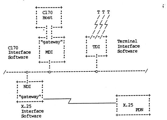
The specific functional role of a DI determines which DCN interface software components are resident in that DI.
