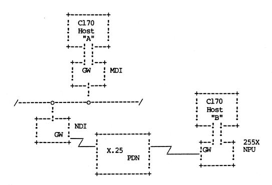
C170 host "A" is connected to an NDI that interfaces to X.25; C170 host "B" is connected to a front-end 255X that interfaces to X.25. The C170 A-A connection in the diagram is really comprised of four distinct intermediate connections joined together by gateway functions:
