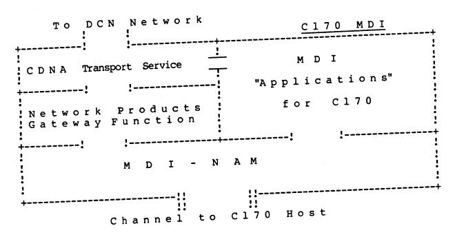
Implementation of MDI-NAM made it possible to define the concept of an MDI "application" within the MDI. An MDI "application" uses the services of MDI-NAM to communicate with a corresponding helper application within the Cl70 host. These application pairs communicate over Network Products A-A connections using Network Products protocols and serve to provide access to Cl70 host resources for the DCN. The three application pairs defined for Release 1 are as follows:
