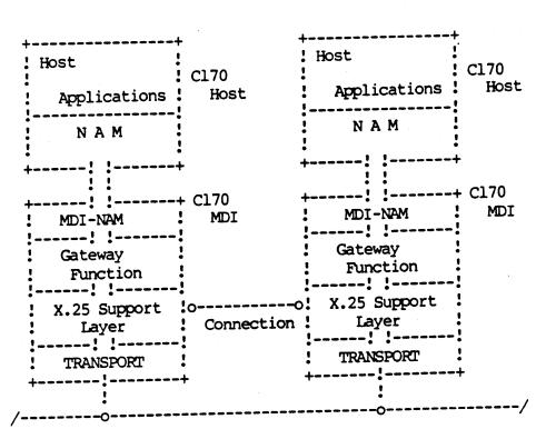
Each C170 host is interfaced to the DCN via a C170 MDI. An NP connection exists between the gateway function in each MDI and its associated C170 host. Gateway functions communicate with each other using an X.25 Support Layer connection.
