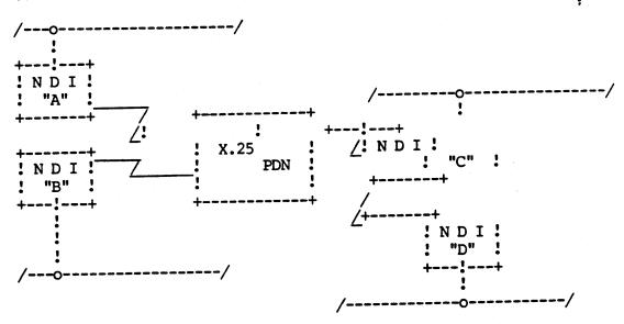
Assuming the configuration is fully connected, each NDI pictured above maintains one Ethernet network solution and three X.25 virtual circuits as point-to-point network solutions; e.g., NDI "A" uses one virtual circuit to communicate with NDI "B", the second to communicate with NDI "C", and the third to communicate with NDI "D". These virtual circuits are used by Internet entities within the NDIs for sending and receiving Internet datagrams.
