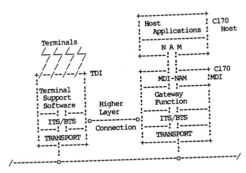
Terminals are interfaced to the DCN by Terminal Support Software in TDI components. The Terminal Support Software maintains a higher layer connection to a T-A gateway function in a C170 MDI, which interfaces the higher layer connection to an NP terminal connection. Host selection is processed by DCN, based on terminal user input. Application selection is processed by NVF in the C170 host.
