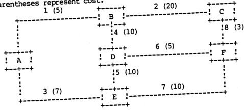
Let us assume that we are looking at routing tables in system A and we are interested in all paths from system A to the network solution numbered 8. The following is a partial list of all possible paths from system A to network solution 8.
