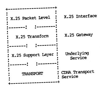
Like NP gateway functions, the X.25 Transform must register its Title in the network Directory. A Title is required for every logical interface to an X.25 Public Data Network (PDN) or X.25 Trunk. A logical interface to a PDN or X.25 trunk is defined as one or more physical links to a PDN or X.25 trunk.
