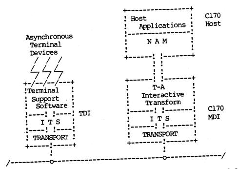
The C170 Interactive Virtual Terminal (IVT) representation of data must be transformed to the ITS representation for transmission across the DCN. This transformation is performed by the "T-A Interactive Transform." The T-A Interactive Transform maps the IVT protocol on to the one supported by ITS. The T-A Interactive Transform is not a layer and is mentioned here simply to provide a more complete picture of the Release 1 higher layer group.
