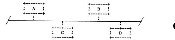
Let us assume we are trying to build the LCR-DS in system A. This configuration contains only one network solution that is locally connected to system A. Systems B, C, and D cannot provide any new information to system A to help it build its LCR-DS. In this case, the LCR-DS will contain a single row that is associated with the locally connected network solution.
