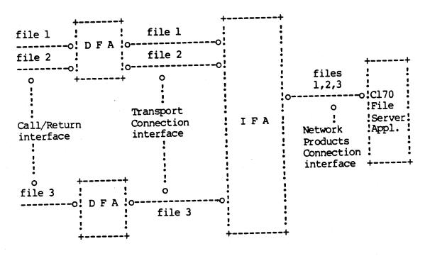
Each IFA in the network can be configured to support any subset of the supported file-types. The configuration can be dynamically altered via configuration commands. The IFA registers a separate Title for every file-type supported. Each Title is associated with the IFA's network address.
