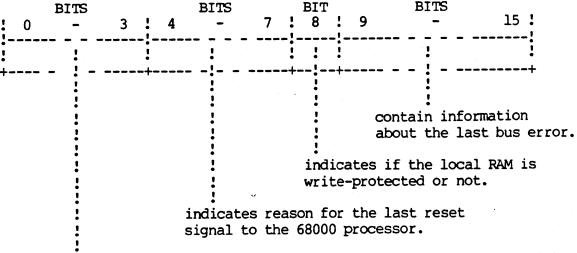
indicate environmental status such as battery low, temperature warning, temperature shut down, and AC power low.
