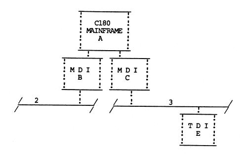
Suppose the C180 mainframe is sending a data unit to TDI-E. The address of this TDI will be stated to be Network ID=3/System ID=E. When this data unit reachs MDI-C, the MDI-C 3B software will do the following:
