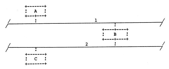
Suppose system A wants to send a data unit to system C. System A will send it to system B on network solution 1. System B will receive it on network solution 1 and will determine that it is destined for system C. System B will then transmit the data unit on network solution 2. System C will receive it on network solution 2. The function performed by system B, in this example, is called a relay.
