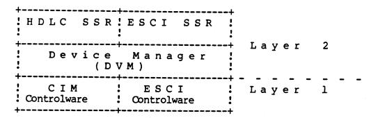
DVM provides a general-purpose interface between layer 1 software on intelligent cards (e.g. CIM and ESCI) and the Stream Service Routines (SSRs), which execute on the MPB card. This interface is provided via a table called Device Control Block (DCB)
