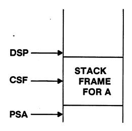
DSP, CSF and PSA are all reset from A's stack frame save area.
