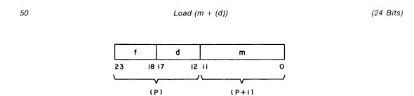
This instruction clears the A register and loads a 12-bit quantity. The upper six bits of A are zero. The 12-bit operand is obtained by indexed direct addressing. The quantity "m", read out of memory location P+1 serves as the base operand address to which (d) is added. If d=0, the operand address is m, but if  $d\neq 0$ , then m+(d) is the operand address. Thus may location d be used for an index quantity to modify operand addresses.
