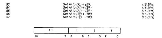
These instructions perform one's complement addition and subtraction of 18-bit operands and store an 18-bit result in address register Ai. Overflow, in itself, is ignored, but an address range fault may result from overflow in this set of instructions.
