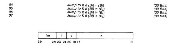
These instructions test an 18-bit word from register Bi against an 18-bit word from register Bj (both words signed quantities) for the condition specified and branch to address K on a successful test. All tests against zero (all zeros) can be made by setting Bj = B0.
