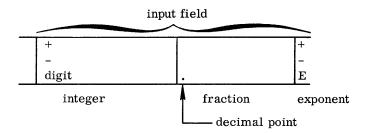
The total number of characters in the input field is specified by w; this field is scanned from left to right; blanks are interpreted as zeros. A field may contain up to 15 significant digits.
