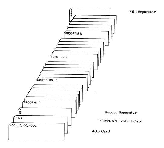
When a RUN card specifies G or C mode and the object program field length differs from the length designated on the JOB card, the compiler does not request the system to change the job field length until completion of the compilation.
