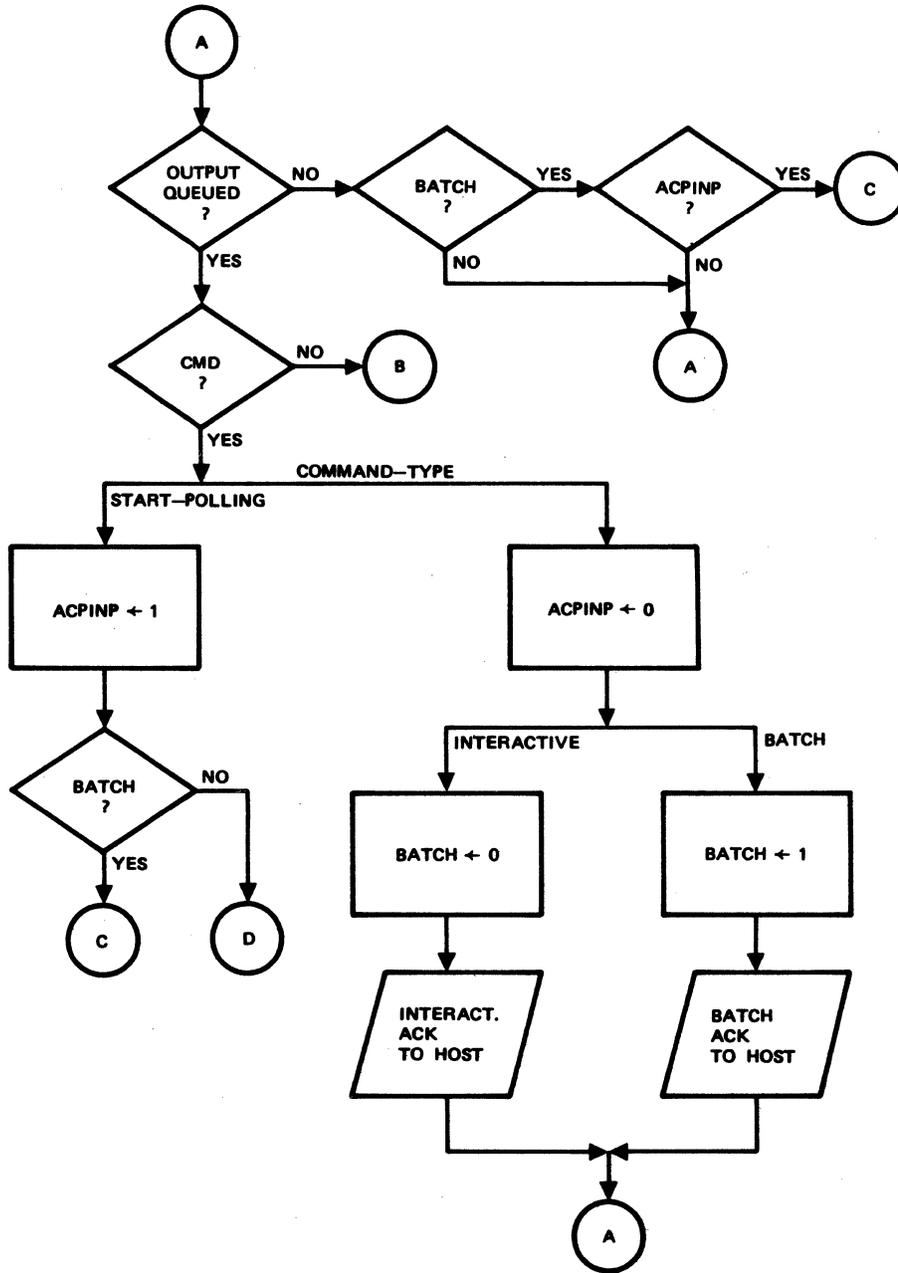
Figure 3-5. Mode 4 TIP Flow Diagram (Sheet 1 of 3)
