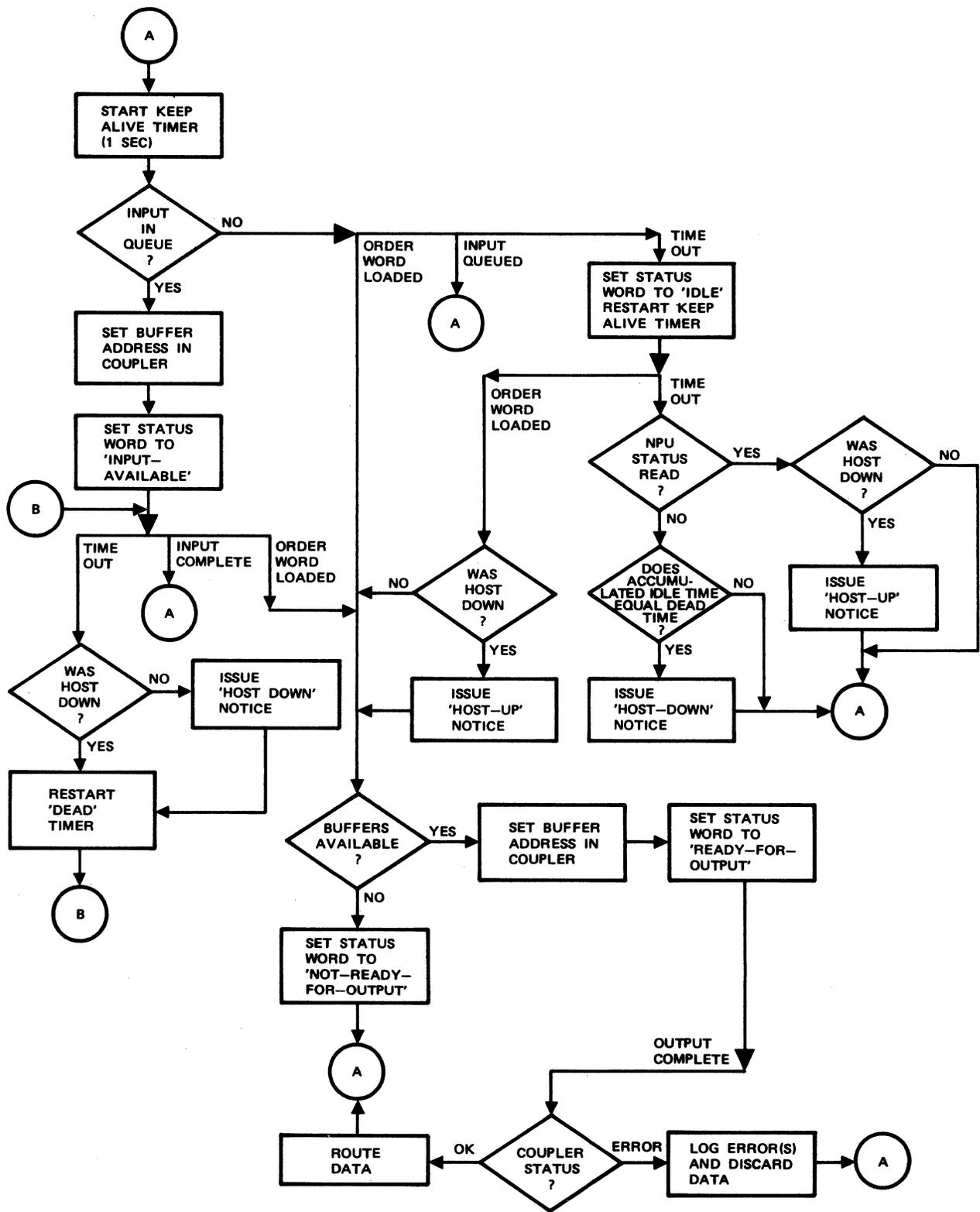
Figure 3-3. Data Transfer Protocol - NPU Sequence, Flow Diagram
