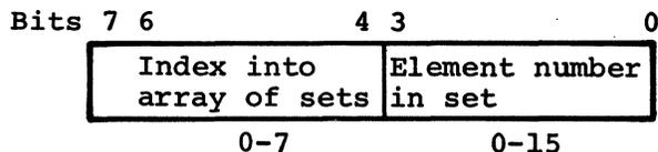
128 bits are reserved (one for each possible ASCII character) in an array of type JSASCIASET, where JSASCIASET = array [0..7] of SETWORD. Characters are located in the set by bit number; e.g., a blank (\$20) is bit number \$20. Bits of the JSASCIASET array are numbered as follows:
