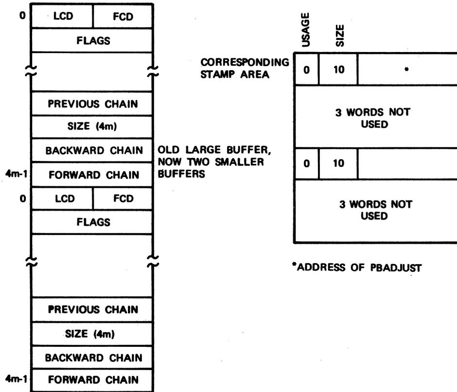
Figure 4-3. Buffer Break-up and Stamping
