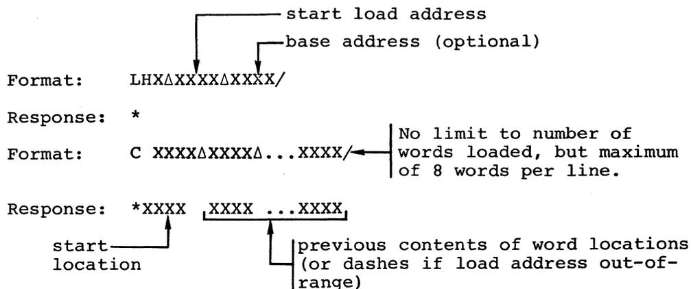
Figure 4-10. C Command and Response Format
