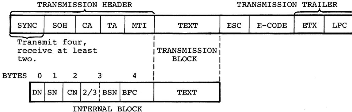
The TIP inserts 14 SYN characters between the MTI and TEXT on all output where MTI is coded for clear write or reset write. Each byte, including the longitudinal parity check (LPC) character, has odd parity in bit 7. The LPC is coded to create odd parity on bits 0-6 of all characters except SYN characters. The TIP generates output parity and passes the received parity bit (entire received 8-bit
