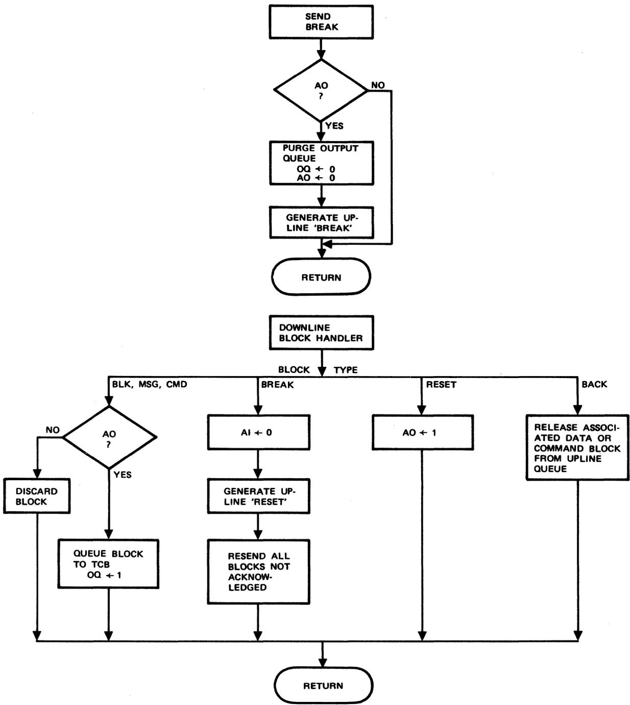
Figure 3-4. Common TIP Subroutines Flow Diagram
