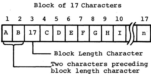
For the above example, the operand must contain an adjustment count of three to compensate for characters A and B and the block length character itself.
