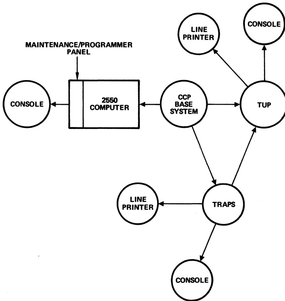
Figure 4-9. Overview Diagram of the Debug Aids System
