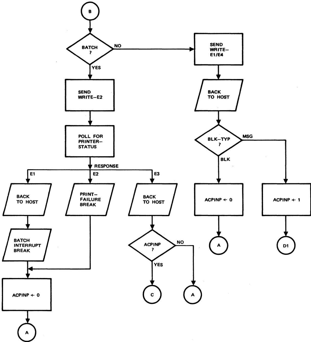
Figure 3-5. Mode 4 TIP Flow Diagram (Sheet 2 of 3)
