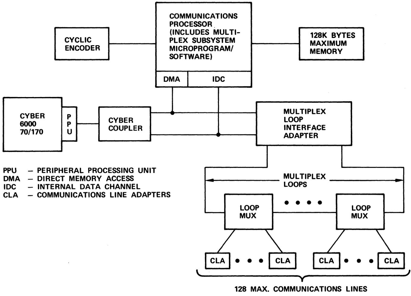
Figure 1-1. Typical System Configuration
