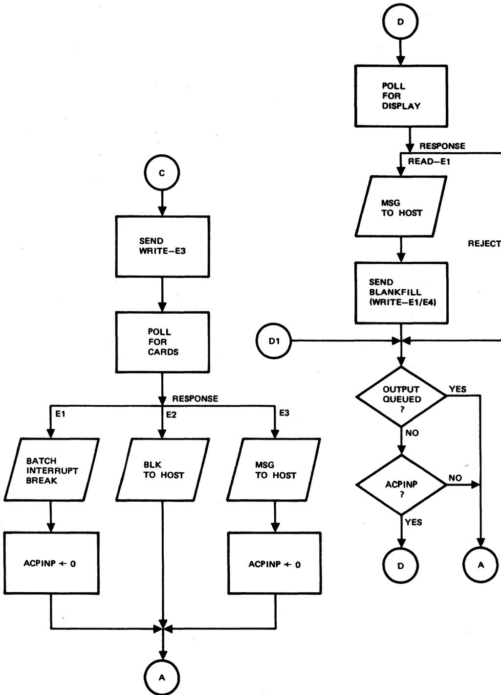
Figure 3-5. Mode 4 TIP Flow Diagram (Sheet 3 of 3)
