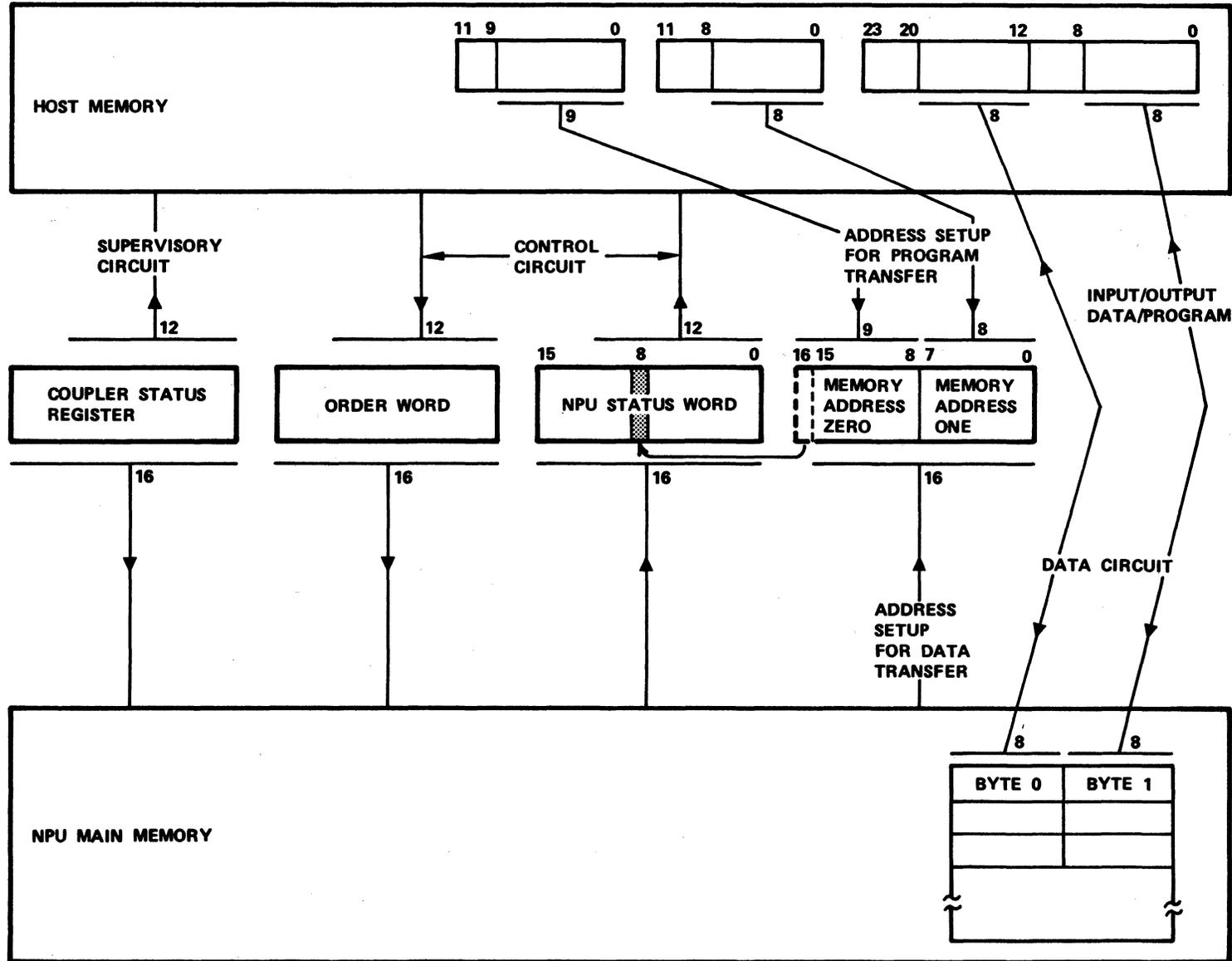
Figure 3-1. CYBER Coupler Registers
