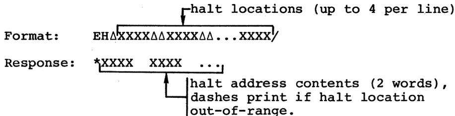
Figure 4-12. Enter Halt Command and Response Format
