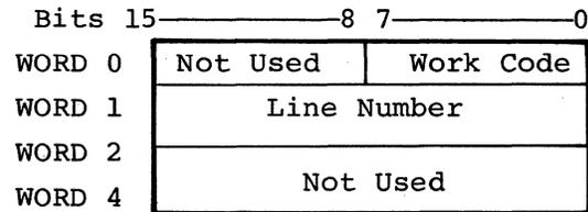
The line number is available as an integer or as two bytes (port and subport). The work code is of type integer and is interpreted as follows:
