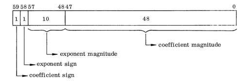
The lower 48 bits are reserved for expressing the magnitude of the coefficient. The computer assumes the binary point to be to the right of the coefficient, thereby providing a 48-bit integer coefficient which is equivalent to about 15 decimal digits. Bit  $2^{59}$  is used to express the sign of the coefficient. The following rules apply to signed coefficients:
