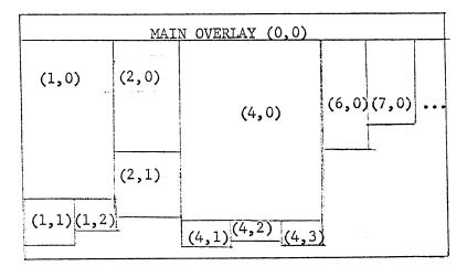
Overlays (1,1) and (1,2) are secondary to overlay (1,0)Overlay (2,1) is secondary to overlay (2,0)Overlay (2,1) may not be called from (1,0) or (1,1) or (1,2) but only from (2,0), or (0,0)
