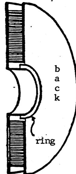
The operating system requires the operator to insert (or remove) the ring depending on the PO = W or R parameter on the LABEL or REQUEST control statement. If the parameter is omitted then no ring is assumed and enforced by the operating system.
