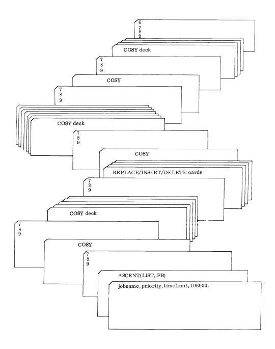
ASCENT/ASPER ASSEMBLY FROM COSY DECKS with five COSY decks on a tape named RIBBON.
