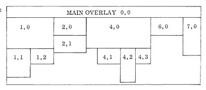
0,0 is the main overlay which remains in memory during execution. 1,0 is a primary overlay. When 1,1, a secondary overlay, is loaded, it is subordinate to 1,0 and there are two levels of overlay. Loading 1,2 destroys 1,1 and 1,2 becomes subordinate to 1,0 but there are still two levels of overlay. When 2,0 is loaded, it destroys 1,0 and its secondary overlay; and there is only one level of overlay until 2,1 is loaded. Similarly, when 4,0 is loaded, it destroys 2,0 etc.
