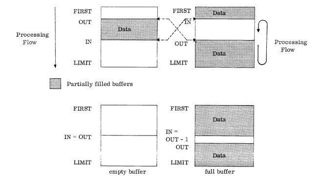
When a buffer is filled to capacity, the unused word between IN and OUT distinguishes it from an empty buffer for which IN = OUT. The capacity of a buffer is LIMIT - FIRST - 1. A buffer is generally initialized with IN = OUT = FIRST, then IN and OUT circle the buffer as data is inserted and extracted.
