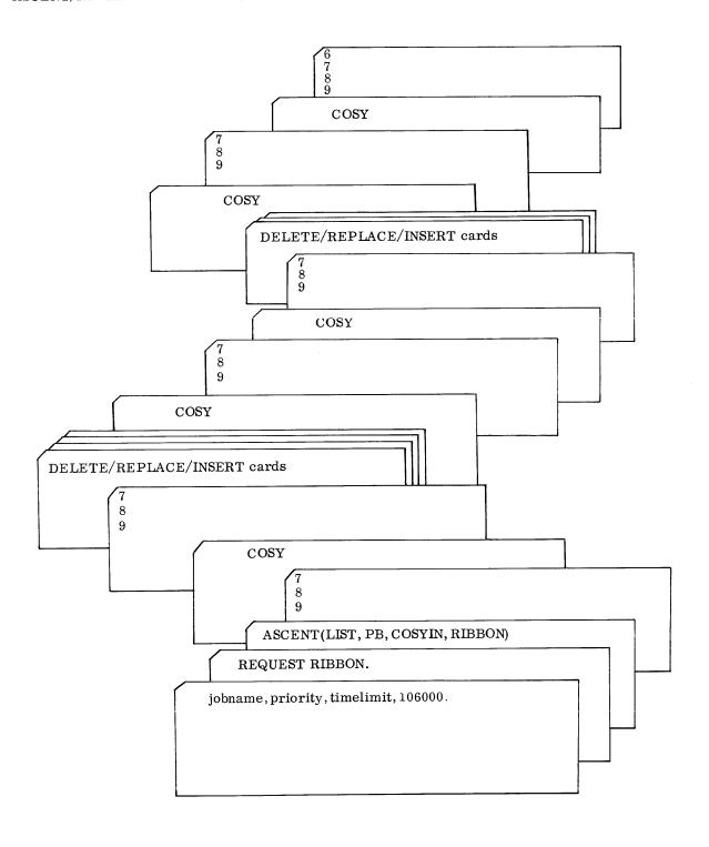
ASCENT/ASPER ASSEMBLY FROM COSY DECKS; with five COSY decks on a tape that will be named RIBBON; the second program to be named PRONTO and the fourth EPIC. Modifications are specified for PRONTO and EPIC only.
