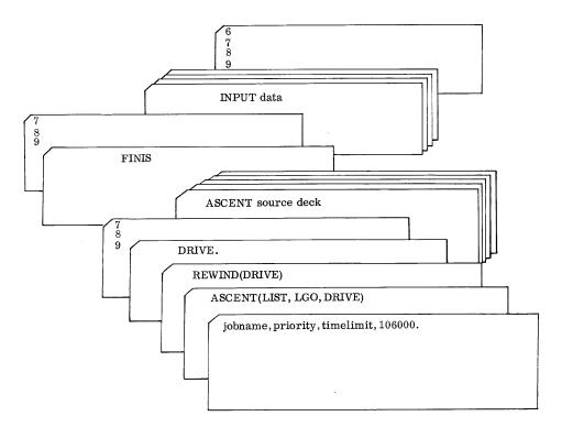
ASCENT/ASPER ASSEMBLY FROM COSY DECKS with modifications; output listing, and binary decks. Since no REQUEST card is included, the input file is on disk.
