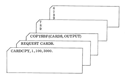
The Hollerith card file read into operator assigned card reader will be printed on OUTPUT file of job CARDCPY.
