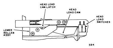
Figure 6-12. Automatic Head Loading Override
