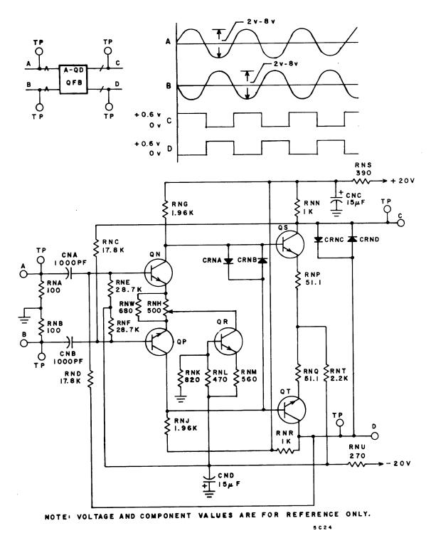
Figure 7-27. Quantizing Detector - QFB
