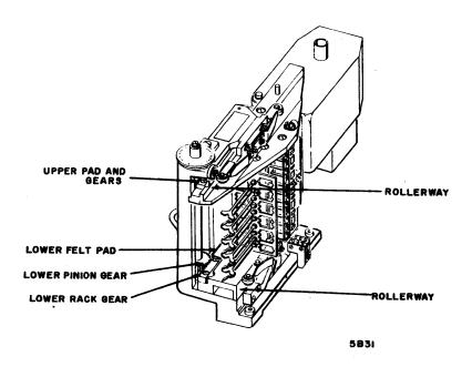
Figure 6-4. Carriage Lubrication
