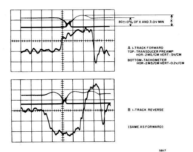
Figure 6-20. Cylinder Transducer Trace
