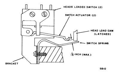
Figure 6-17. Heads Loaded Switch (S300A/S300B) Adjustment (Shown without TB302/TB303)
