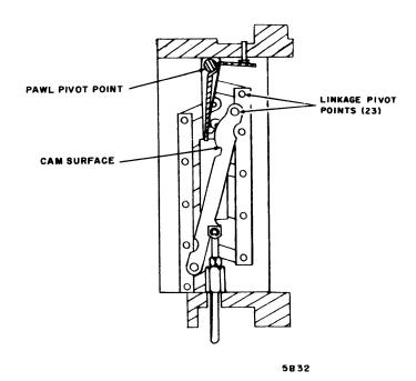
Figure 6-5. Head Latch Lubrication
