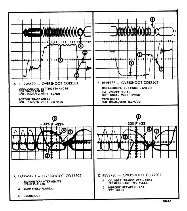
Figure 6-32. Intermediate Speed Characteristics
