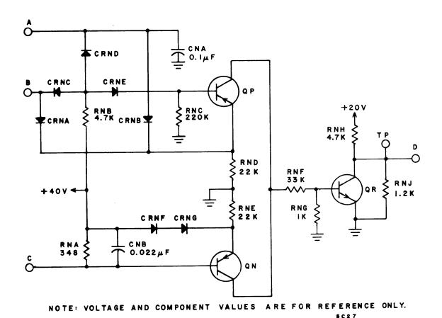
Figure 7-26. Quantizing Detector - QFA
