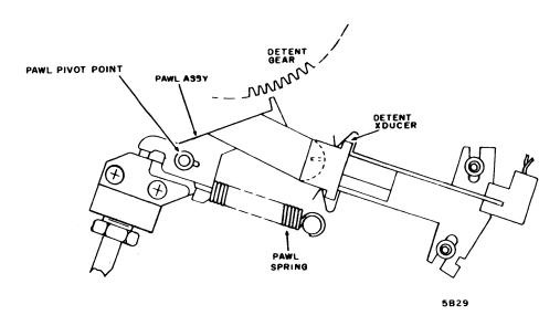
Figure 6-3. Detent Pawl and Gear Lubrication
