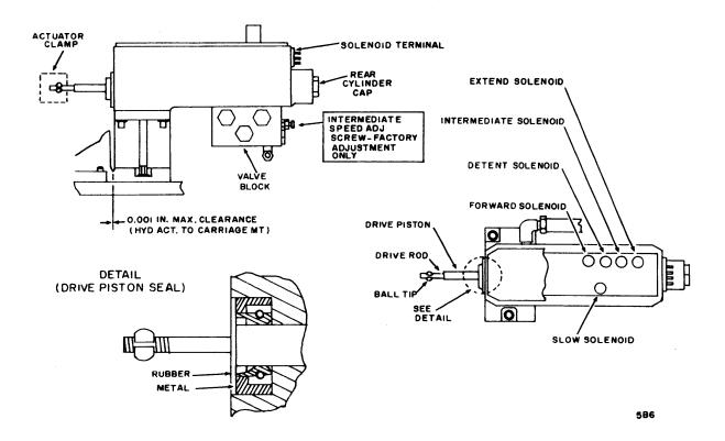
Figure 6-14. Hydraulic Actuator
