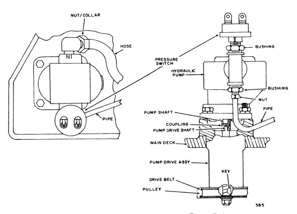
Figure 6-13. Hydraulic Pump and Pump Drive.
