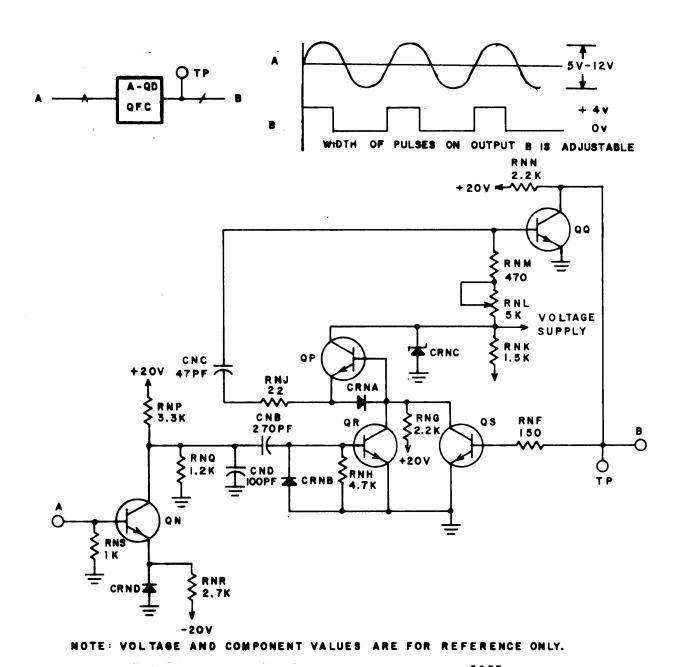
Figure 7-28. Quantizing Detector - QFC
