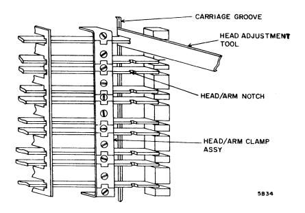
Figure 6-8. Head/Arm Assembly Adjustment
