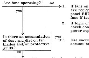
If fans on underside of logic chassis are not operating, check power supply panel BRUSH MOTOR fuse. Replace fuse if faulty.
