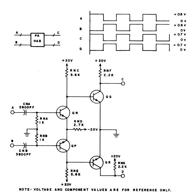
Figure 7-11. High Level Amplifier - HAB
