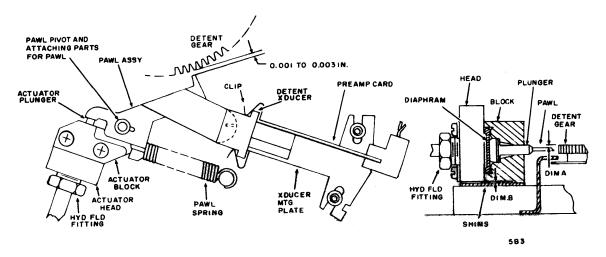
Figure 6-11. Detent Mechanism
