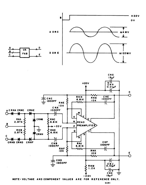
Figure 7-8. Low Level Amplifier - FAB
