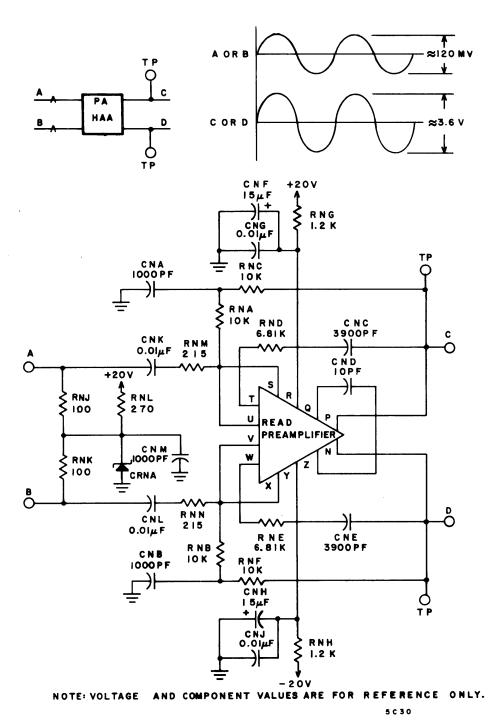
Figure 7-10. High Level Amplifier - HAA
