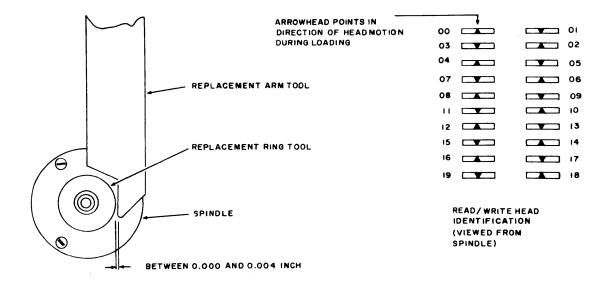
Figure 6-19. Carriage/Carriage Mount Alignment
