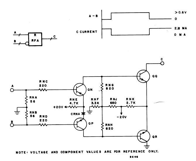
Figure 7-31. Line Receiver - RFA
