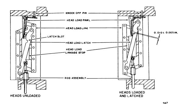
Figure 6-15. Head Load Linkage
