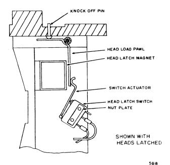
Figure 6-16. Head Latch Switch (S304) Adjustment (Shown without TB204)
