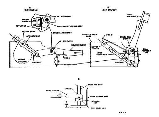
Figure 6-10. Disk Cleaner Adjustment
