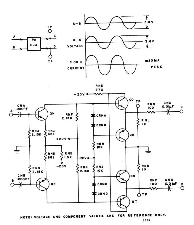
Figure 7-12. High Level Amplifier - HJA
