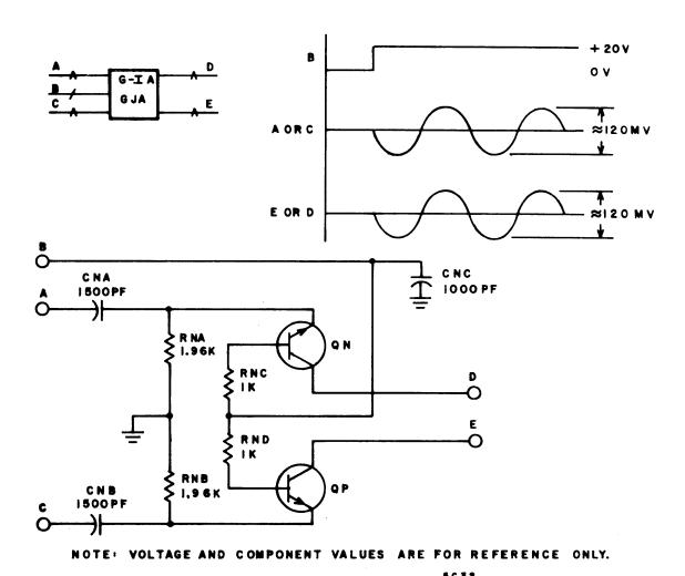
Figure 7-9. Gated Intermediate Level Amplifier - GJA
