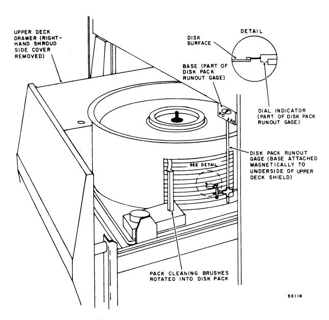
Figure 7-52. Disk Pack Runout Check
