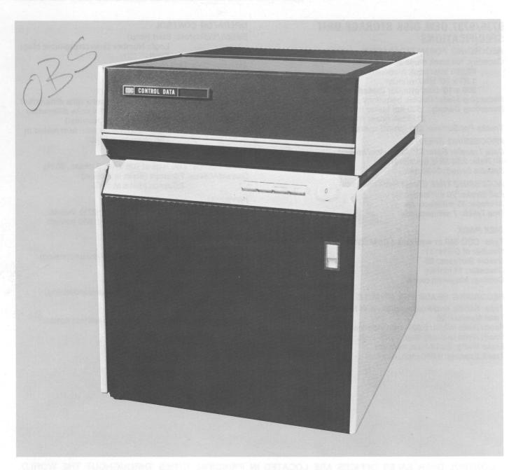
The CONTROL DATA 9736 and 9737 Disk Storage Units are large-capacity, random-access storage devices which record and read information in IBM-compatible recording modes. The recording format is fully compatible with the IBM 2314 Direct Access Storage Facility, permitting full pack interchangeability between the 9736/9737 and any machine using the same recording format.
