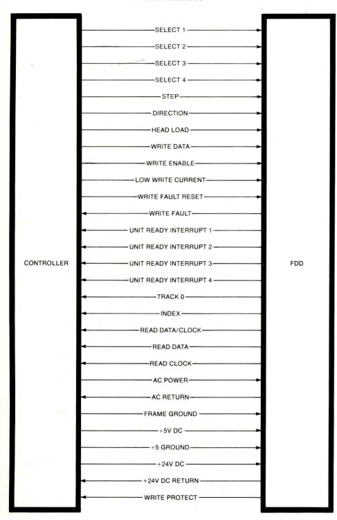
The 9404 is capable of handling double-density recording, using MFM encoding, and allows for future expansion of data capacity. An optional write-protect feature is also available, which uses a phototransistor LED system to optically sense a hole in the disk jacket. If necessary, this function can be disabled by covering the hole with opaque tape.
