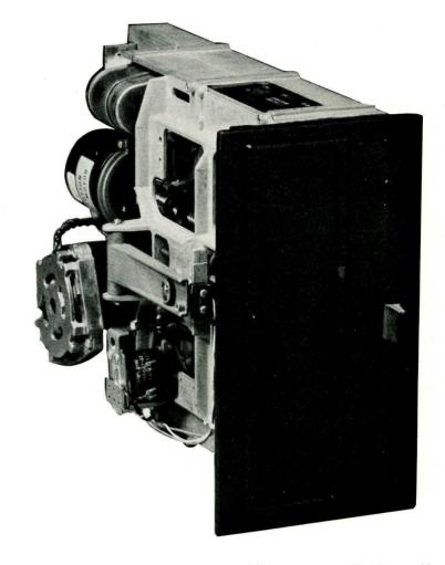
the spindle rotates the diskette within the envelope. This envelope has an inner liner which serves to cushion and clean the medium automatically during rotation. Optical sensing of the index hole is achieved through a phototransistor and LED system.
