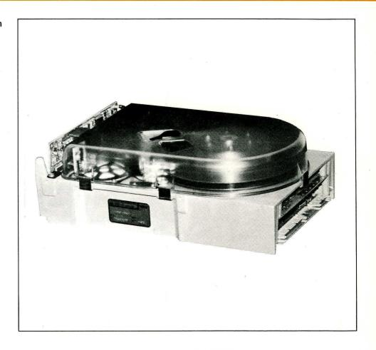
The use of large scale integrated (LSI) circuitry and microprocessor control means that only three circuit boards are used. Phaselocked oscillator data recovery and reference clocking increases data integrity.
