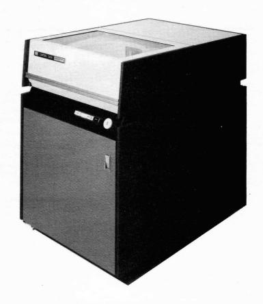
The CONTROL DATA 9747 Disk Storage Unit is a 60-million byte, random-access storage device. It uses CDC® 9873 Disk Pack, or equivalent, for the recording and reading of information in IBM (or customer derived) format compatible recording modes. Each removable pack contains eleven disks. Information is stored on 20 oxide-coated surfaces at 200 tracks per inch, 400 tracks per surface.
