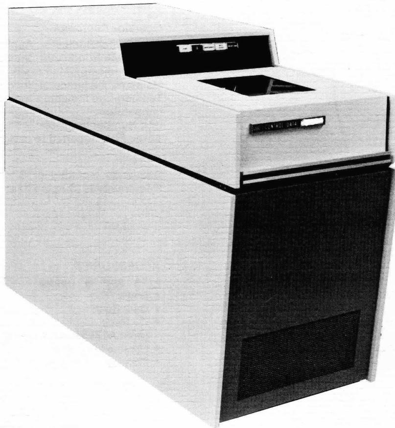
CONTROL DATA 9754 Disk Storage Units are 100-million byte, random-access peripheral storage devices which use the CDC® 879 Disk Pack or equivalent (IBM 3336). Each disk pack is removable and contains 10 oxide recording disks. Data can be written on 19 of 20 surfaces, and positioning information is permanently recorded on the remaining recording surface.
