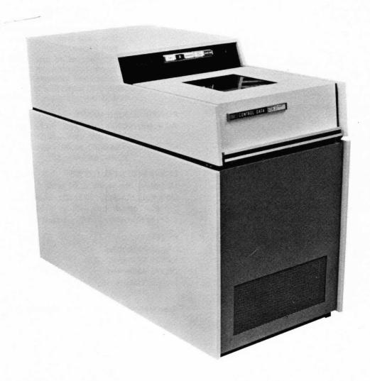
The CONTROL DATA 9756 Disk Storage Unit is a 100-million byte, random-access peripheral storage device. It uses the CDC® 879 Disk Pack, or equivalent IBM 3336, for the recording and reading of information. Each disk pack is removable and contains ten oxide-coated recording disks. Data can be written on 19 of the 20 recording surfaces. Positioning information is permanently recorded on the remaining recording surface.
