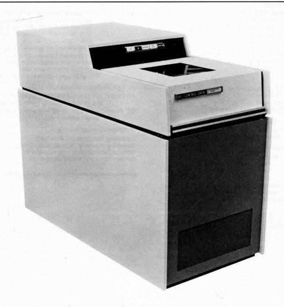
The CONTROL DATA 9780 Disk Storage Unit is a 200-million byte, random-access, peripheral storage device. Each removable disk pack contains ten oxide recording disks. Data can be written on 19 of the 20 recording surfaces. Positioning information is permanently recorded on the remaining surface.
