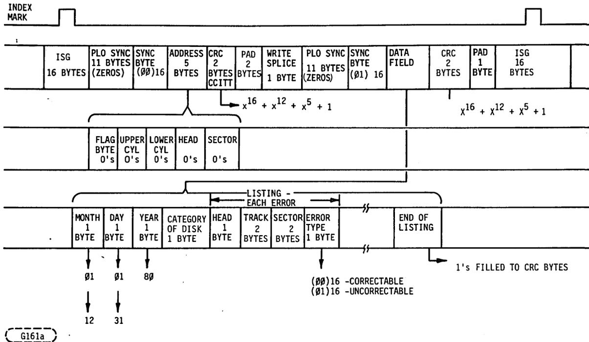
Figure 8. Format for Surface 0, Track 0, Sector 0--
