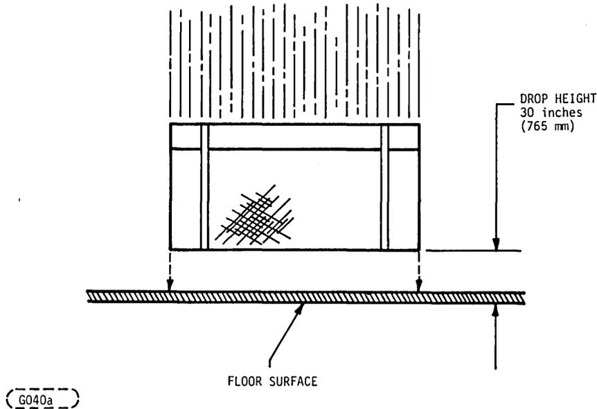
Figure 6. Flat Drop Test
