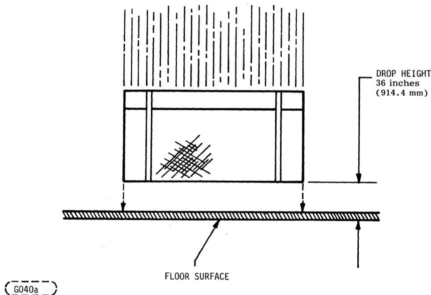
Figure 6. Flat Drop Test
