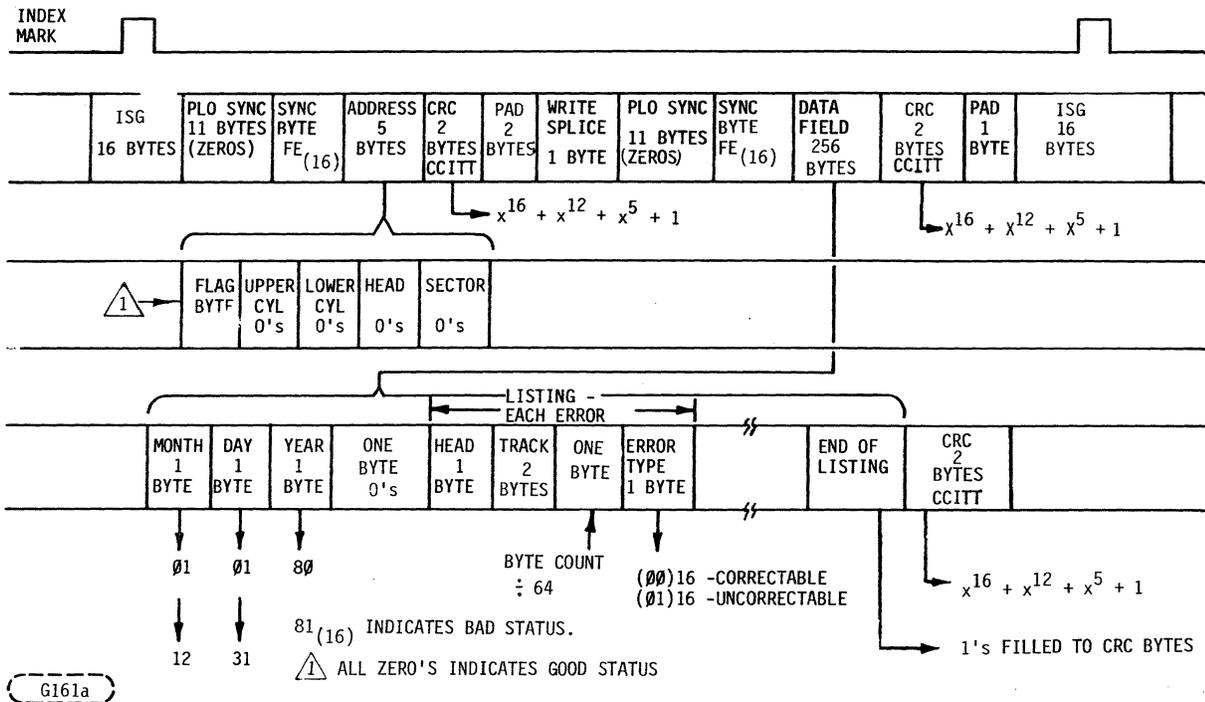
Figure 8. Format for Surface 0, Track 604, Sector 0--
