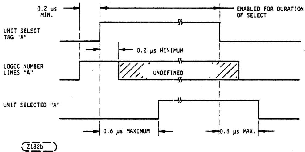
Figure 5.2-5. Logic Number Select and Timing Diagram
