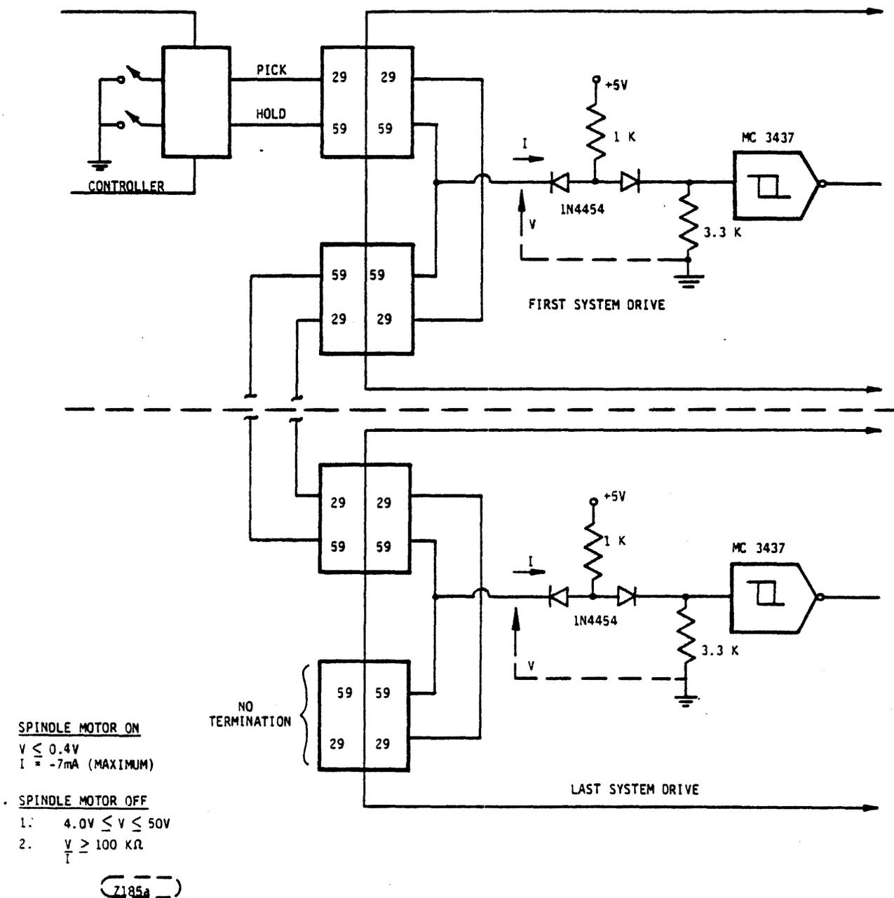
Figure 5.2-6. Spindle Motor Power Sequencing Control
